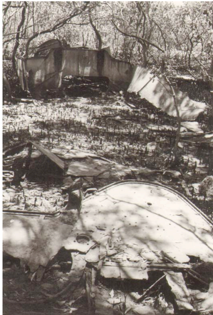
Figure 62. 1966 photograph of Mosquito 's partially intact stern section. Note Bulkhead 5 in foreground and Bulkhead 7 in centre background. Image courtesy of S. Prior and the Queensland Maritime Museum (no accession number).
