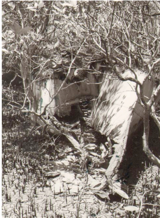
Figure 64. 1966 bow-on photograph of Mosquito's forward section, showing corrosion-generated separation of the bow (at right centre) from the midships hull. Image courtesy of S. Prior and the Queensland Maritime Museum (no accession number).
