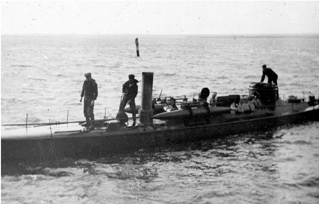
Figure 49. Lonsdale underway in Port Phillip Bay ca. 1905, showing Whitehead torpedoes mounted on dropping gear amidships. Image courtesy of the Queenscliff Maritime Museum (no accession number).
