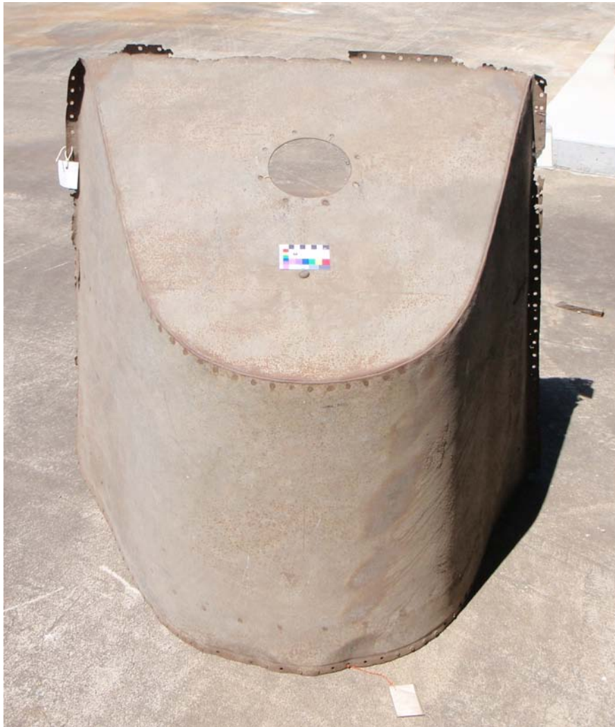
Figure 66. Mosquito's intact stern casemate, currently housed in the collection of the Queensland Museum, South Bank. Note the overall excellent condition of the casemate's painted galvanised steel fabric.
