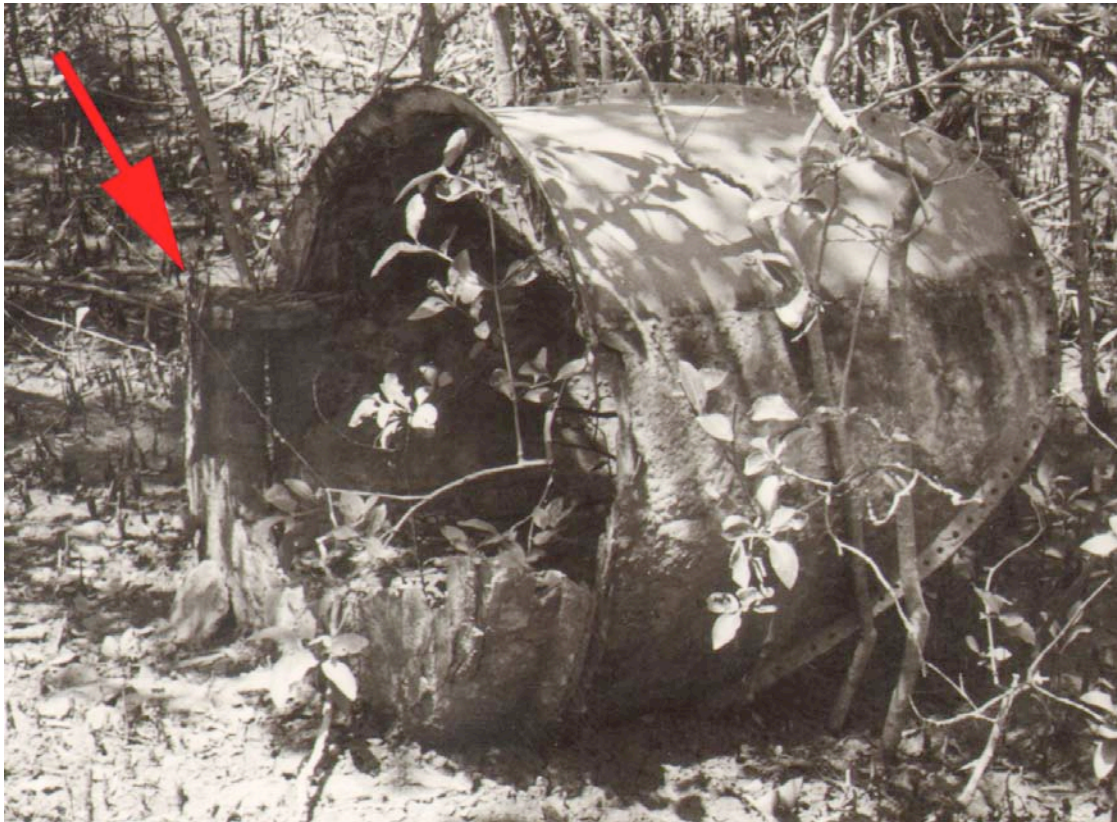
Figure 63. Mosquito 's disarticulated but largely intact conning tower, as photographed in 1966. Arrow highlights remnants of articulated conning tower hatch cover. Image courtesy of S. Prior and the Queensland Maritime Museum (no accession number).
