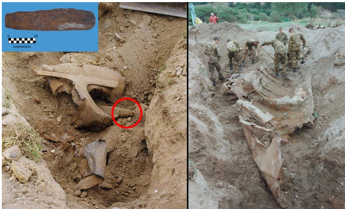
Figure 72. Left , Defender's crushed stern section. Circle highlights wooden plug embedded in exterior screw aperture at the time of recovery; right , Defender's midships section in situ ; inset , wooden plug removed from the interior propeller shaft bushing. Images courtesy of David Bundy.
