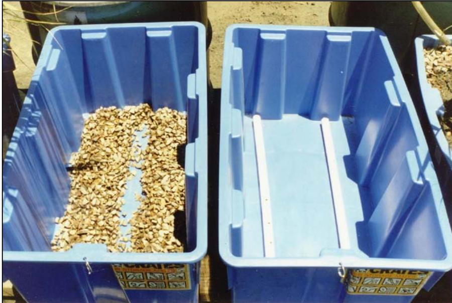
**Plate 2.1a** the outlet pipework (right) for drainage and collection of outflow from the system, gravel (right) used to protect drainage system from blockages in the RBTS cells.
