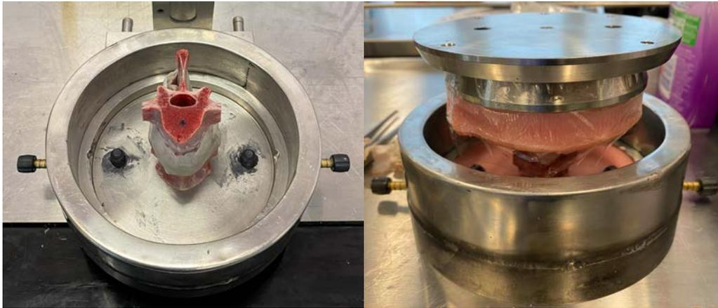
*Figure 3.4 Alignment of the centre of the disc and the bottom cup and the disc covered with saline-soaked gauze (left) and completion of potting with the top and bottom cups (right)*
