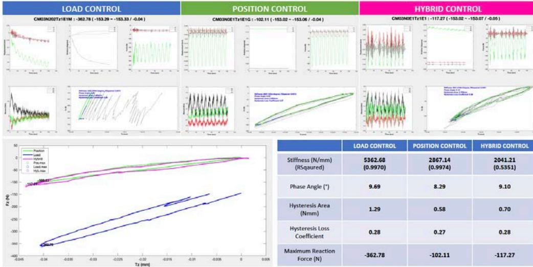
Appendix E.2 CM04 (10 cycles at 0.1Hz, additional flexion test for 5 cycles at 0.01Hz)
