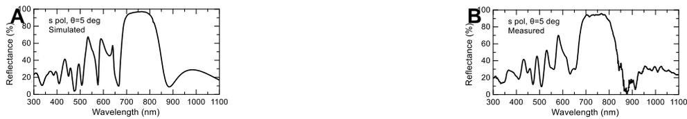
**Figure S18** (A) and (B) Simulated and measured reflectance spectra, respectively.
