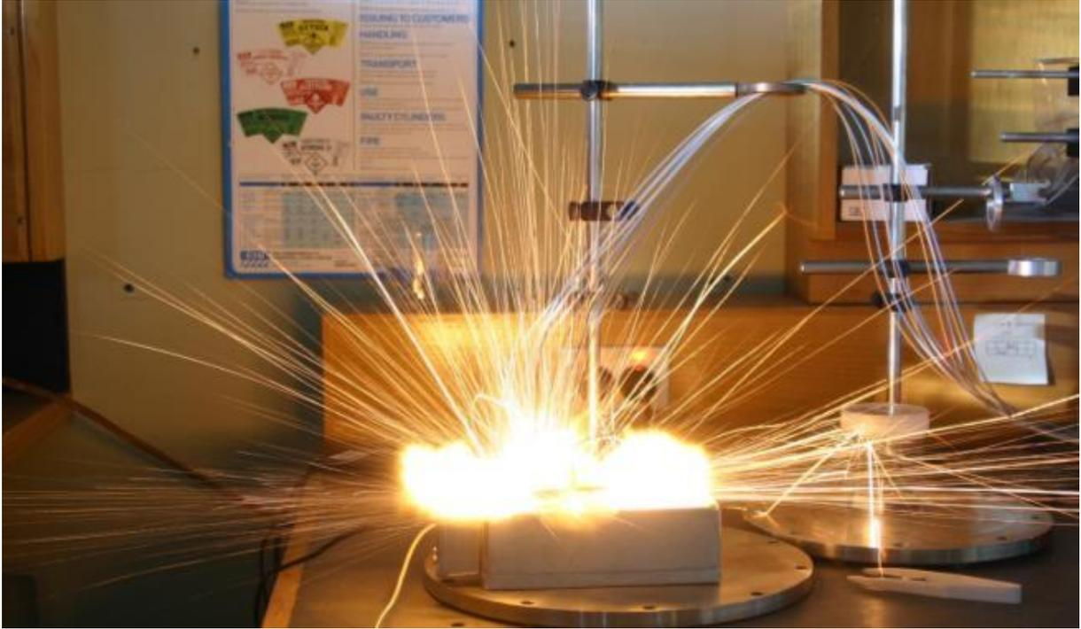
**Approximately 20 mg of porous silicon loaded with sodium perchlorate, initiated using a high voltage spark.**
