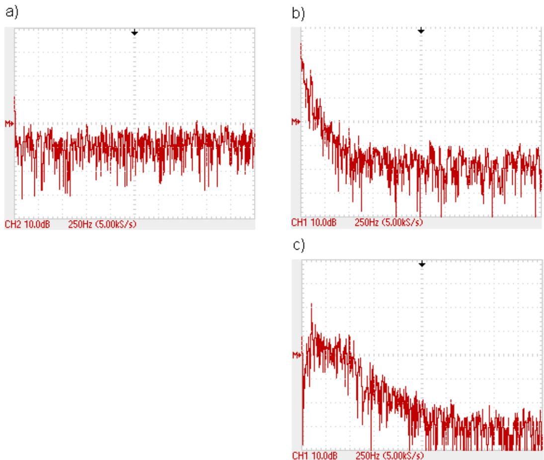
*Figure 7-3 Frequency response of analog ECG monitors: a) white noise source with consistent frequency response from dc to 2.5 kHz, b) Datex AS/3 Anaesthetic Monitor with 30 dB fall in frequency response by 300 Hz, and c) HP 78353 Neonatal ECG Monitor has a slower roll-off with -30dB at 1000 Hz*
