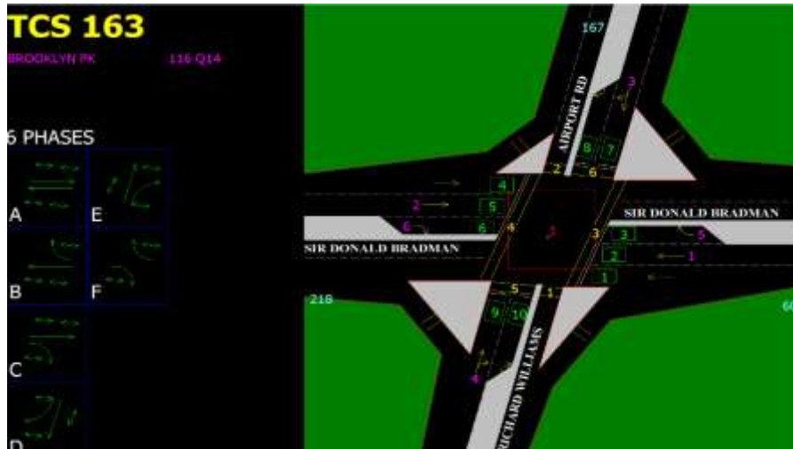
Figure 3: SCATS images showing detector locations.
