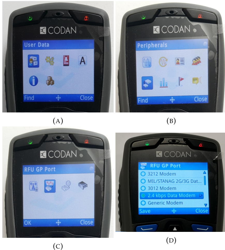
FIGURE 9.7: The sequence of steps followed on the handset for Codan HF radio to make the 2.4kbps internal data modem accessible via the RFU6 connector.
