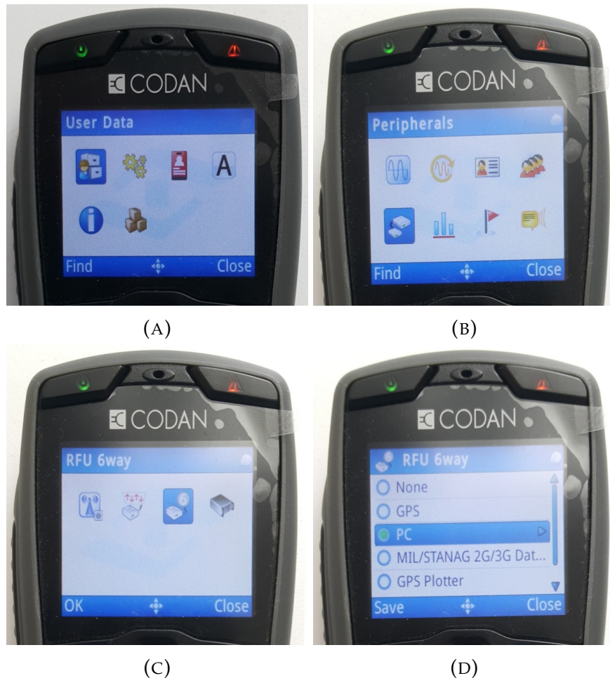
FIGURE 9.8: The sequence of steps followed on the handset for Codan HF radio to tell the Envoy radio that a computer is connected to the 6-way RFU6 cable.
