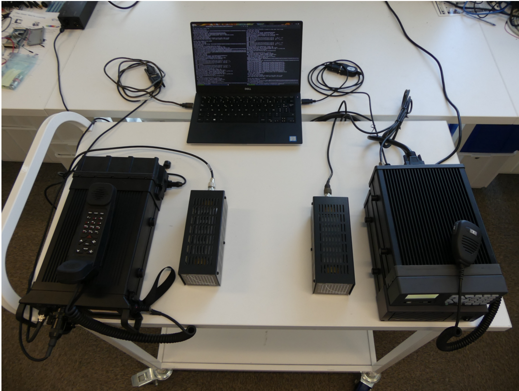
FIGURE 9.1: Two Barrett HF radios 2090 and 2050 during a live lab test, and each one is connected to a dummy load and serial interface. Both radios have been provided by Barrett company.
