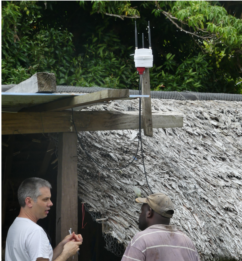
FIGURE 3.8: Installing Serval Mesh Extender on a roof of a house during the piloting of Serval Mesh in Vanuatu 2017. The process doesn't require any expensive hardware or expertise, making it possible in a small village. Also, as there is no configuration required, the devices can be moved around based on the needs of the community, without needing to coordinate with, or seek permission of a network operator or other authority.
