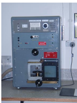
Figure 3: Electrostatic discharge apparatus purpose built by the Defence Science and Technology Group.
