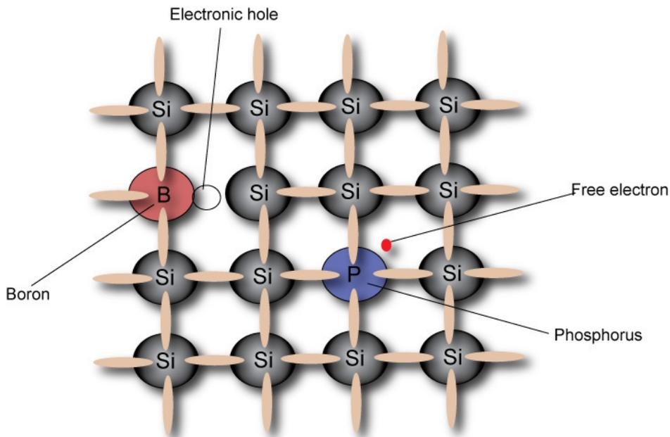
**Figure 1.4 – An illustration for both boron (p-type) and phosphorous (n-type) doping within the silicon lattice. Boron doped silicon contains electronic holes that can act as current carriers. The current carriers for phosphorous doped silicon are the free surplus electrons.**
