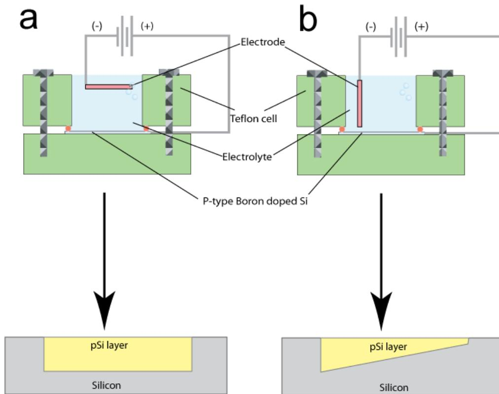
**Figure 1.7 – (a) Conventional anodisation of pSi. The film is evenly anodised anisotropically, thus give an equal thickness throughout. (b) Asymmetric anodisation of pSi resulting in a thickness and pore size gradient.**
