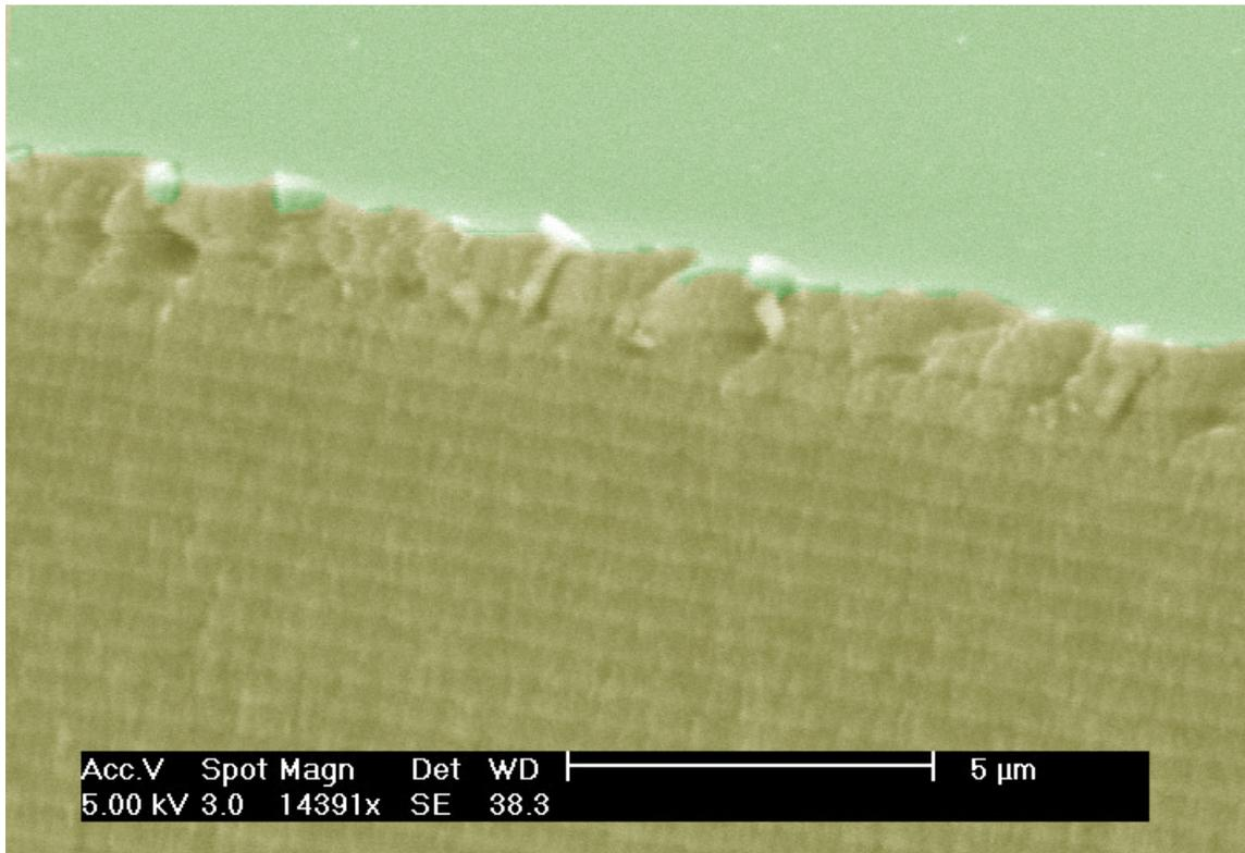
**Figure 1.5 – SEM of a multilayered pSi film. The alternating layers within the film can be easily resolved.**
