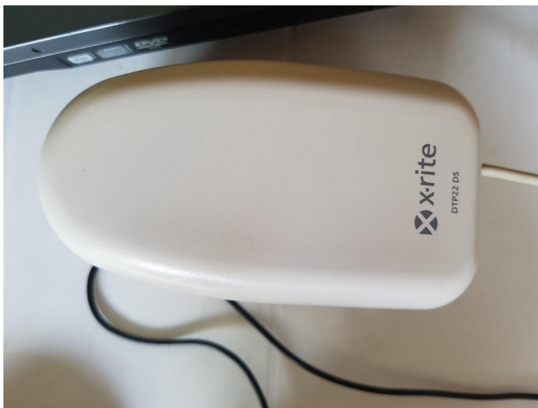
Figure 104 X-Rite Inc. DTP22 Digital Swatchbook Spectrophotometer (Photo: K. Jerbić).
