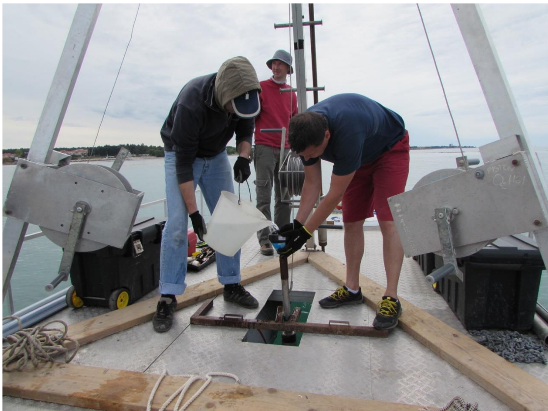
Figure 76 Adding water to the hydraulic core catcher (Photo: K. Jerbić).
