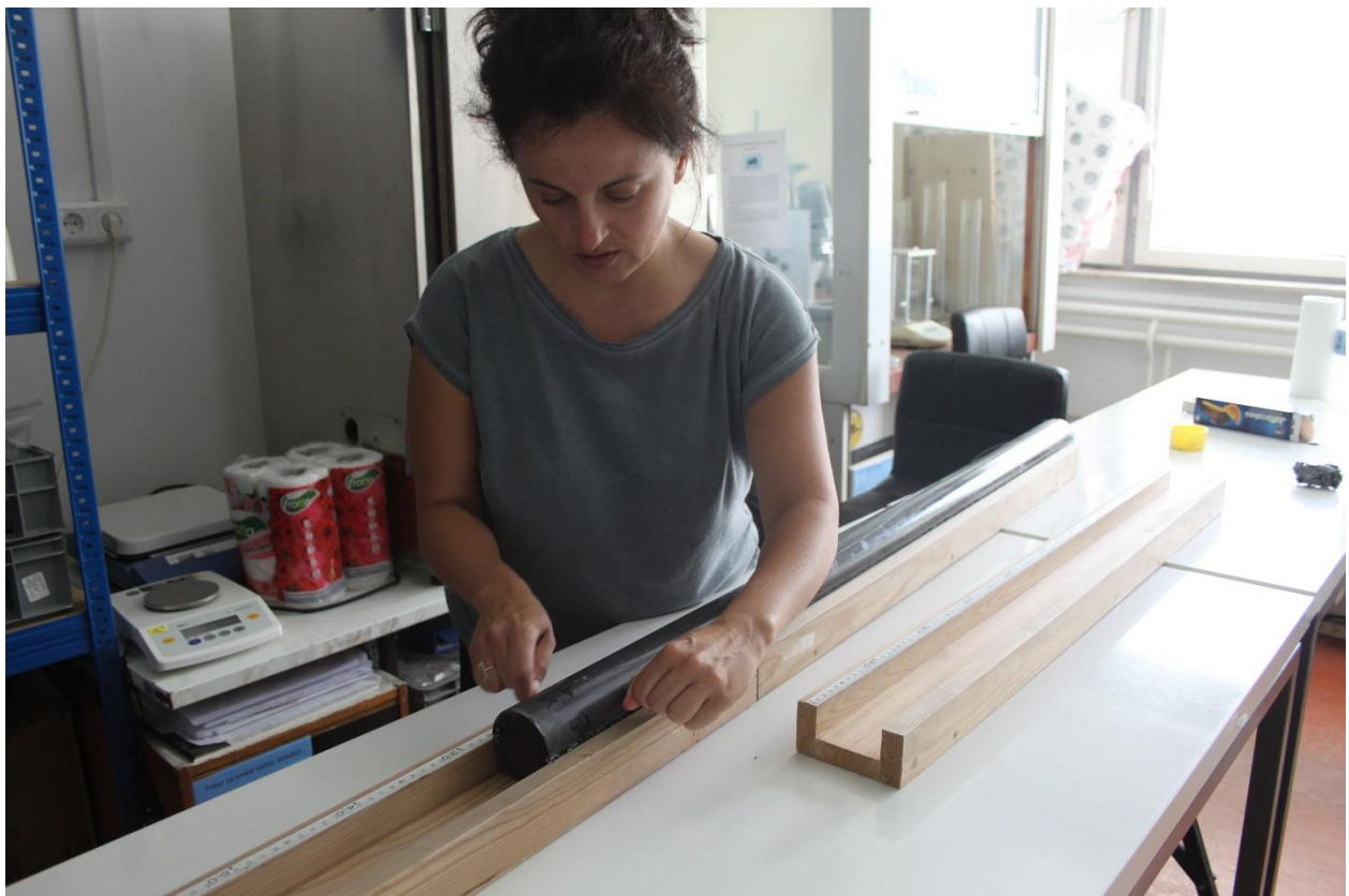
Figure 100 Cutting through the sediments with a fishing line (Photo: D. Brunović).
