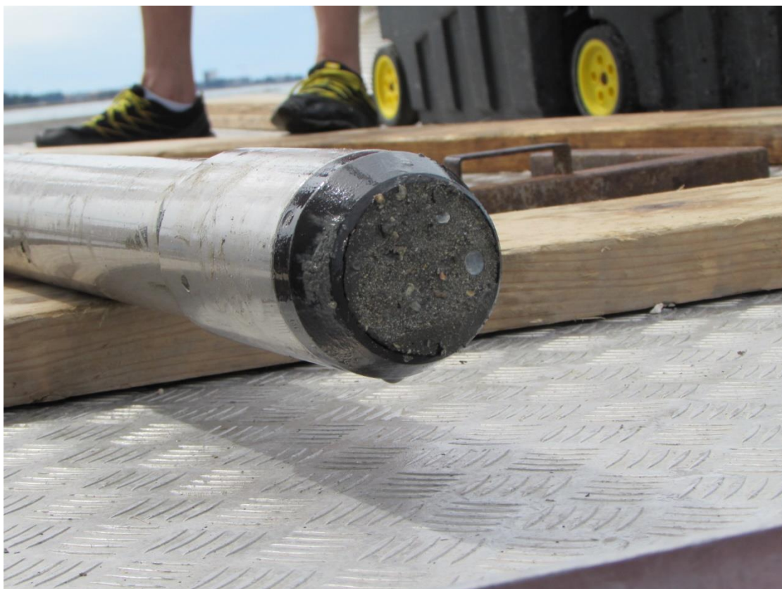
Figure 74 Steel tube corer filled with sediment (Photo: K. Jerbić).
