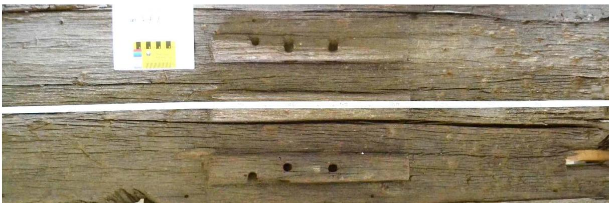
Figure 6-10. Lashing holes on Butuan Boat 1 keel plank lug 7 (KP-L7). Photograph by author.
