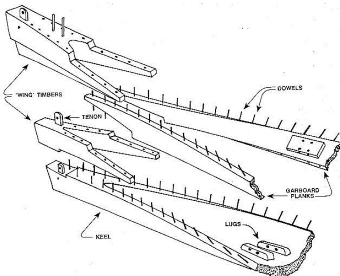
Figure 7-6. Hypothetical reconstruction of the Butuan Boat 2 wing end b Vosmer (Clark et al. 1993).
