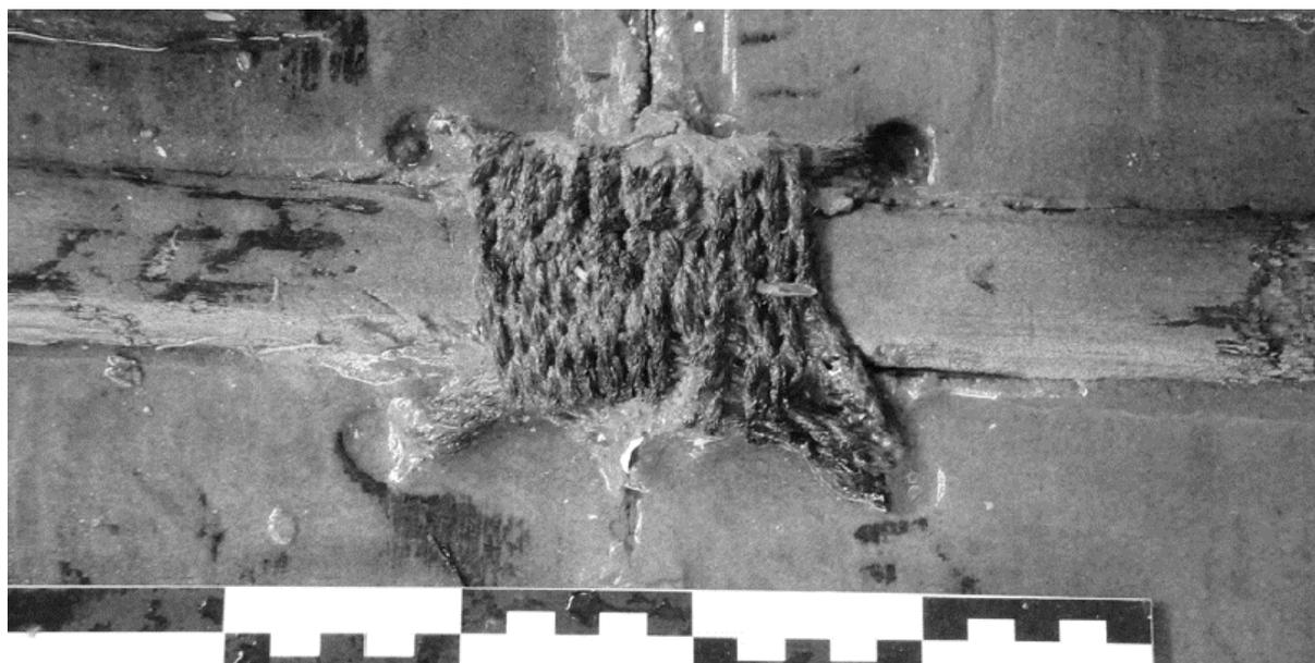
Figure 5-21. Close-up of Punjulharjo Boat plank lacing (Manguin 2012:Figure 7).
