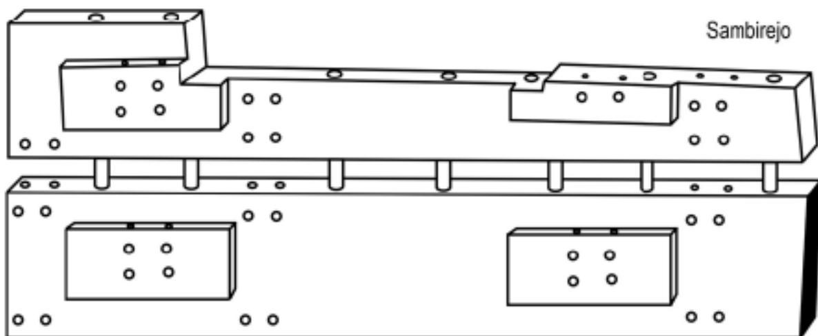
Figure 5-19. Drawing of Sambirejo planks showing lugs, lashing, lacing and dowel holes (Manguin 2012:Figure 2).
