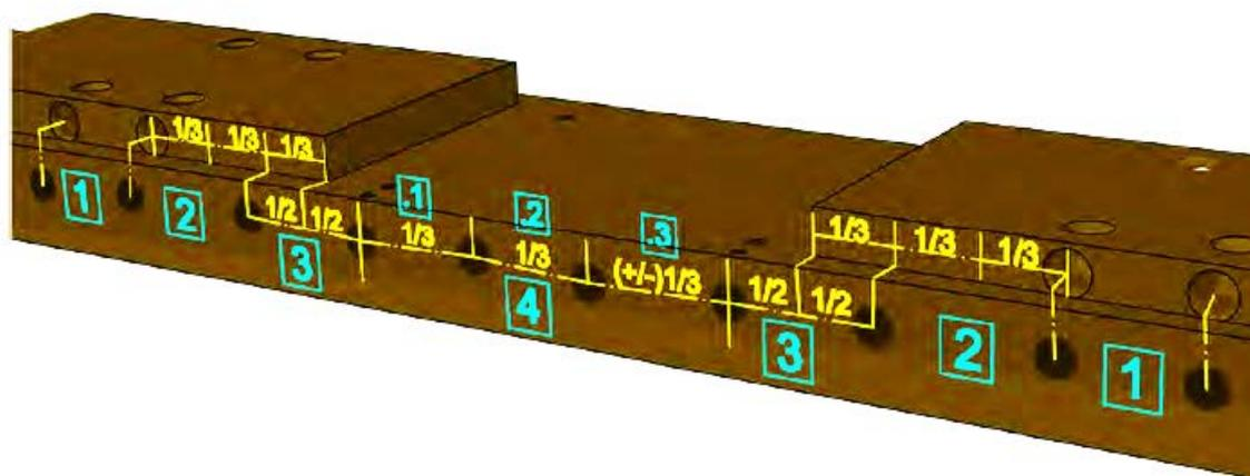
Figure 5-26. Cirebon type (iii) plank showing dowel arrangement (Liebner 2014:Figure 3.2-37).
