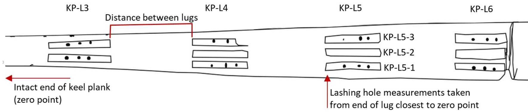
Figure 6-2. Keel plank lug and lashing holes measurement conventions. Illustration by author.
