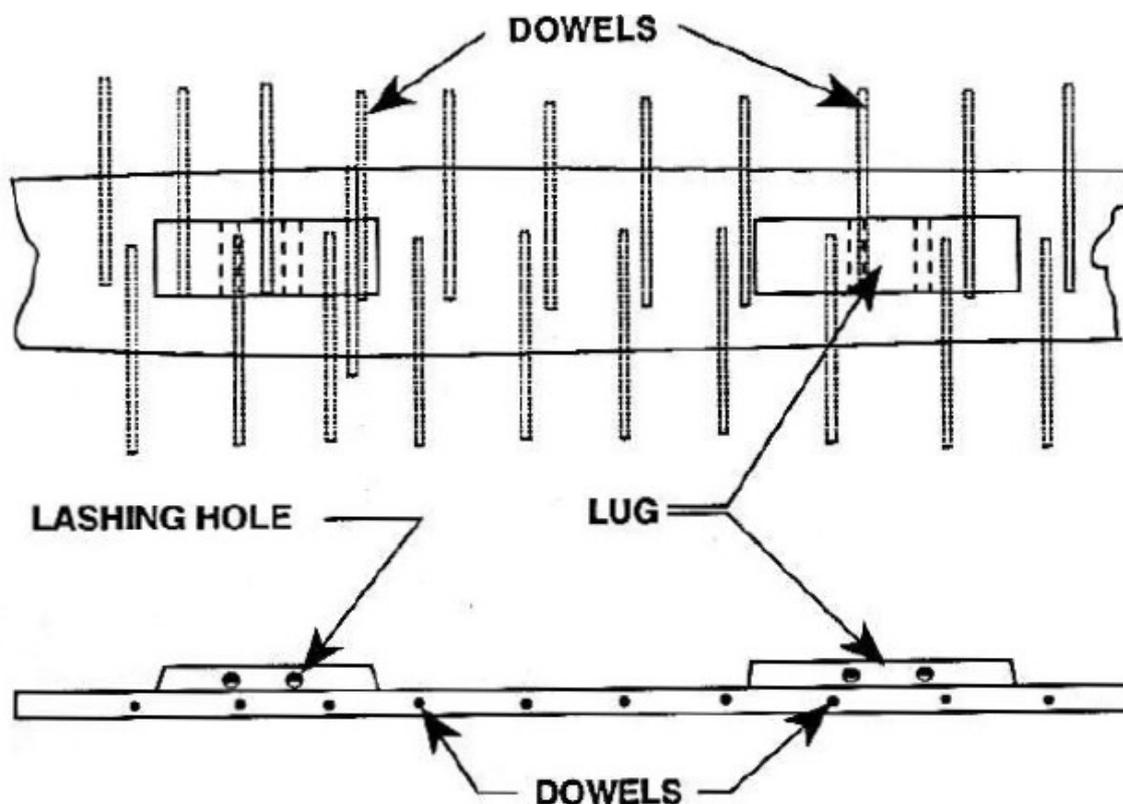
Figure 5-11. Dowel and lug arrangement of Butuan Boat 5 (Green et al. 1995:185)
