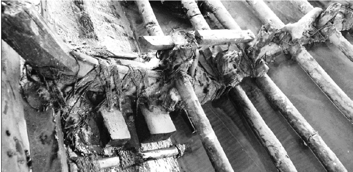
Figure 5-20. Punjulharjo Boat with well-preserved ligatures used for lashing and lacing (Manguin 2012:Figure 6).
