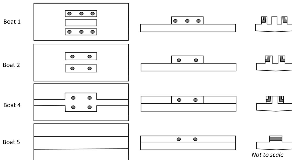
Figure 7-5. Lug arrangements on the Butuan Boat keel planks. Illustration by author.
