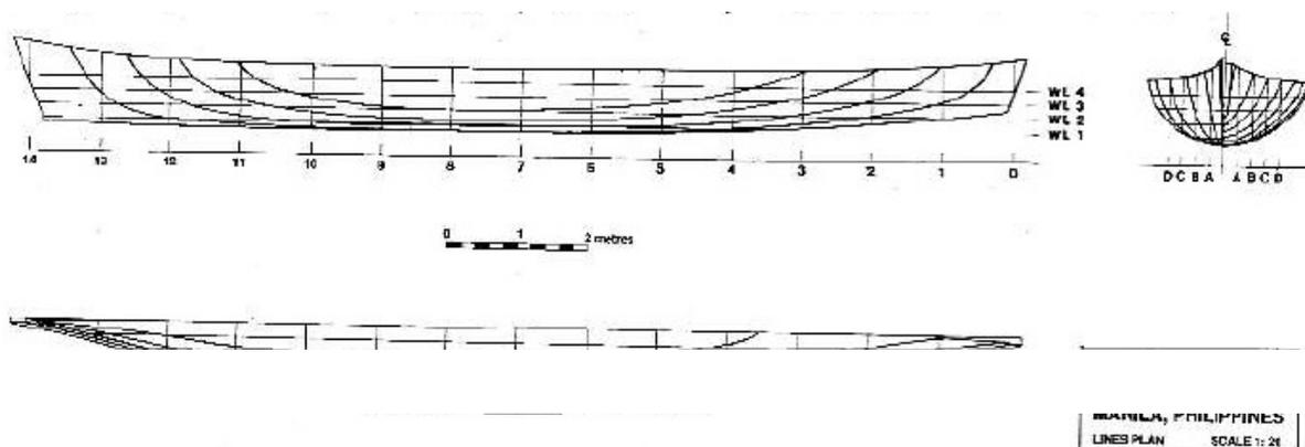
Figure 5-9. Lines drawing of Butuan Boat 2 by Vosmer (Clark et al. 1993:152).
