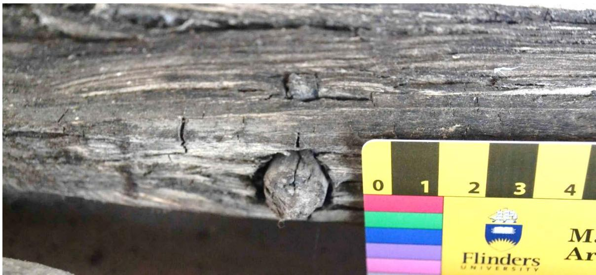
Figure 6-41. Wooden peg locking dowel in place in Butuan Boat 5 planking Photograph by author.
