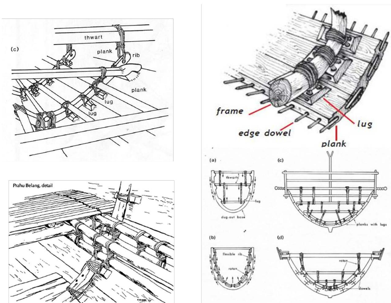
Figure 7-3. Depictions of lashing patterns and techniques by various authors based on Indonesian boats (upper-left, bottom-left and bottom-right; Horridge 1985:52, 53) and a hypothetical reconstruction of Butuan Boat 2 (upper-right; Cuevas et al. 2004:5).
