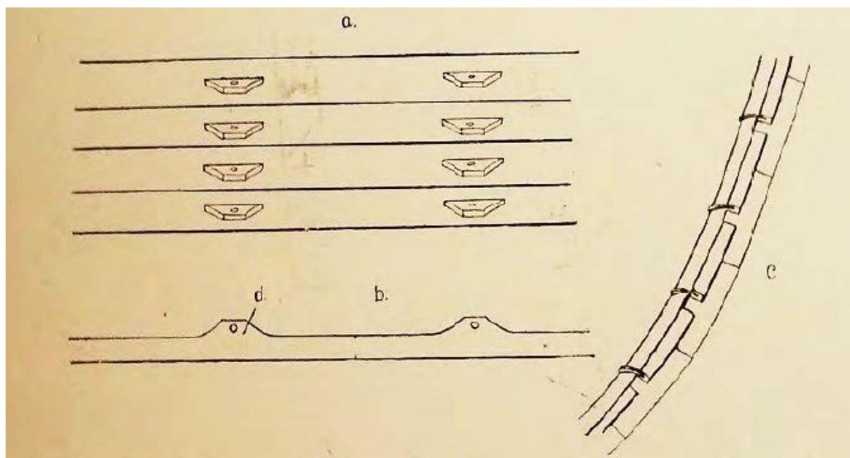
Figure 4-6. Drawing of a Galela boat showing construction details (Hornell 1920:59).
