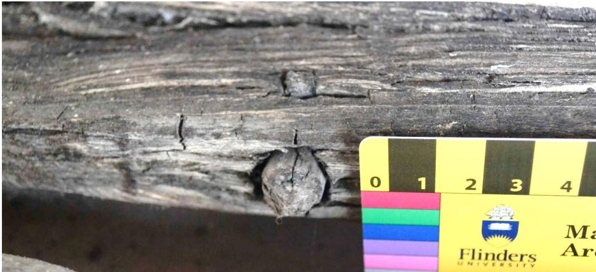
Figure 6-41. Wooden peg locking dowel in place in Butuan Boat 5 planking Photograph by author.
