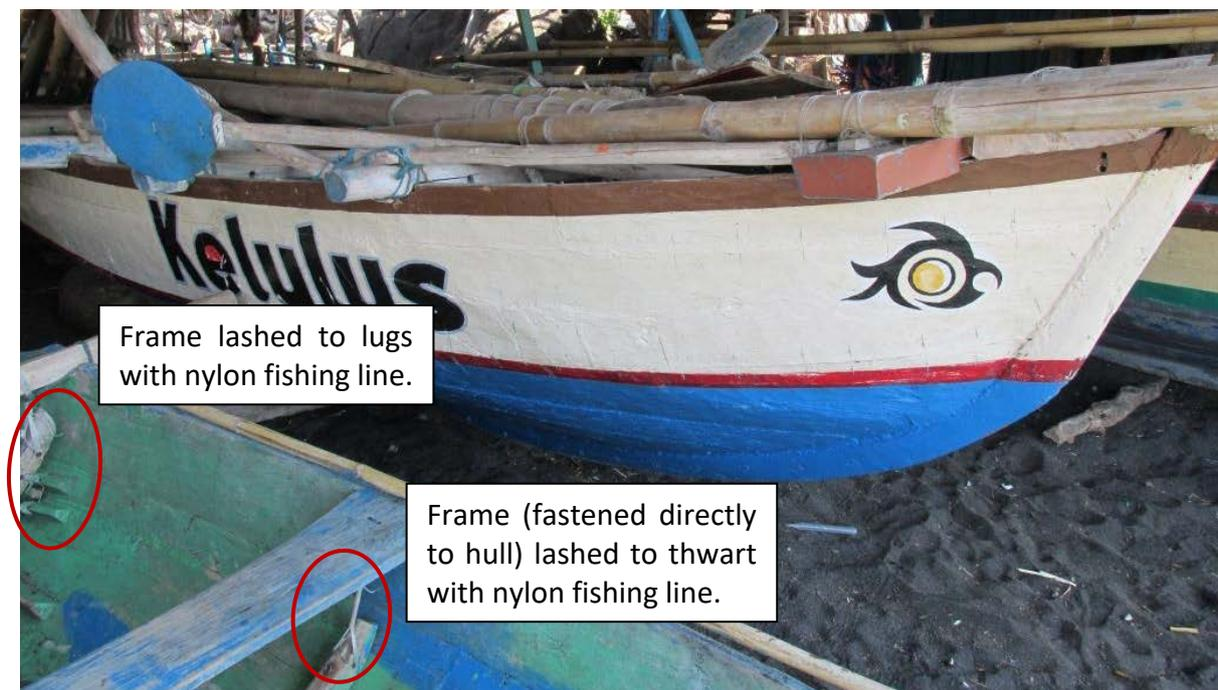
Figure 4-19. Lamalera boat with lugs and nylon fishing line lashing (foreground; after Burnet 2015).
