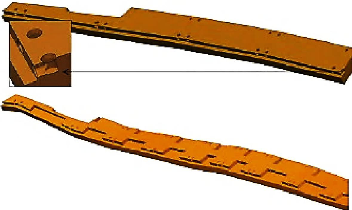
Figure 5-25. Cirebon planks types (i) (top) and (ii) (bottom; from Liebner 2014:Figures 3.2-28–29).
