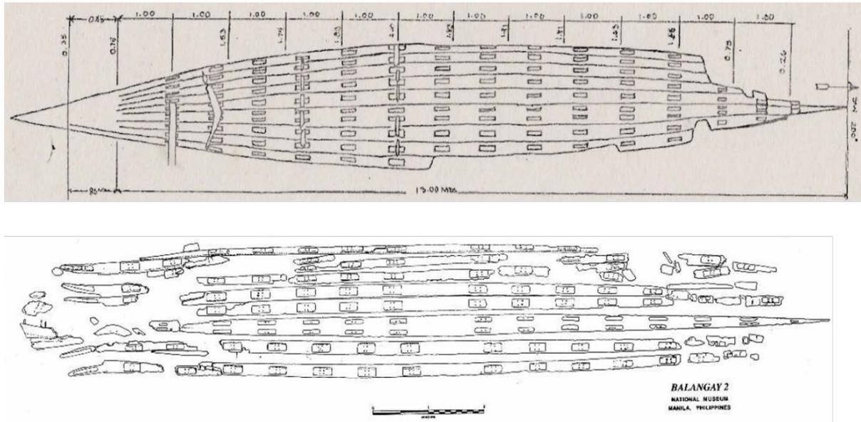
Figure 2-8. (Top) Timber drawing of Butuan Boat 2 that appeared in a conservation report showing an additional row of lugs (Abinon 1978:5). Compare to bottom drawing from a tracing of a photomosaic (Clark et al. 1993:45).
