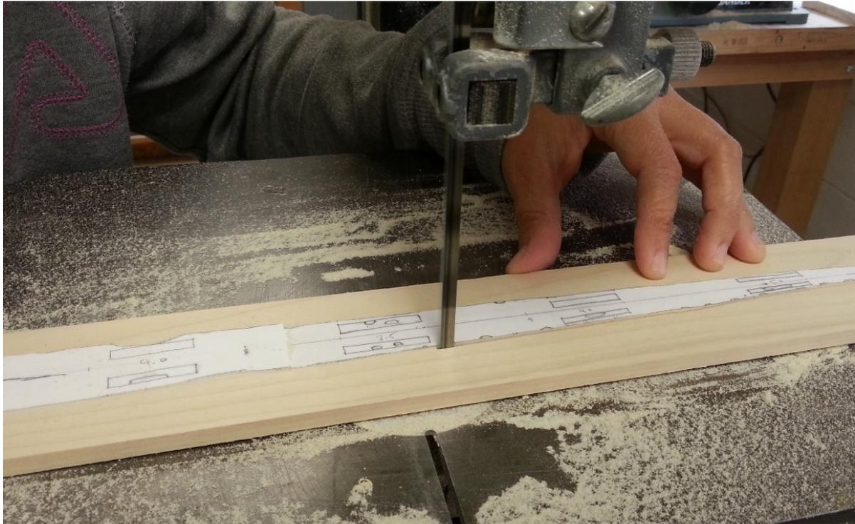
Figure 1-5. Cutting the wood to shape with a band saw. Photograph by Wendy Van Duivenvoorde.
