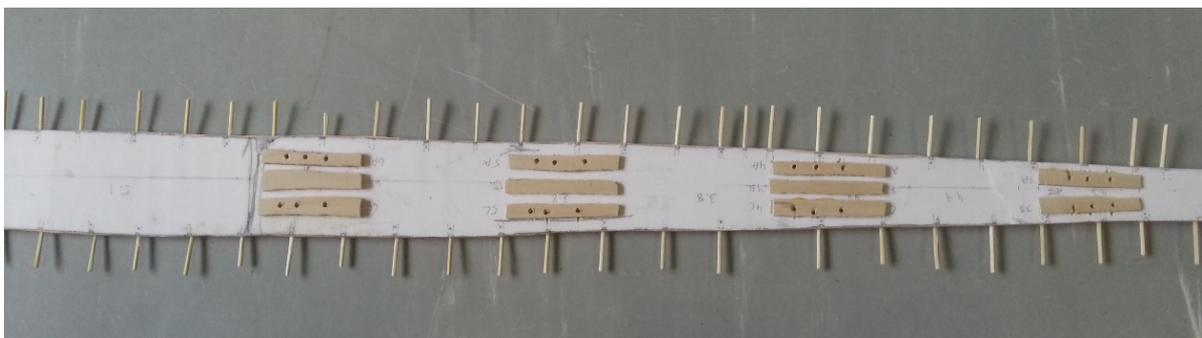
Figure 1-6. Dowels inserted into plank edges. Photograph by author.
