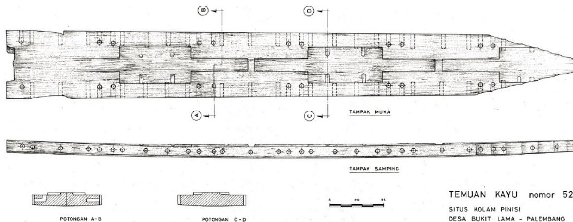
Figure 5-18. Kolam Pinisi Boat keel plank (Manguin 2012:Figure 3).
