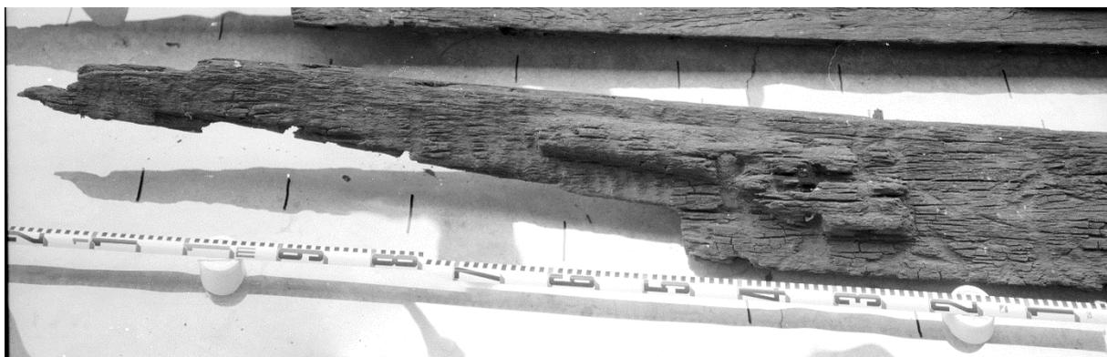
Figure 6-11. Butuan Boat 1 Strake A-1 (STR-A1) possible scarf end. Photograph courtesy of the Western Australian Museum.
