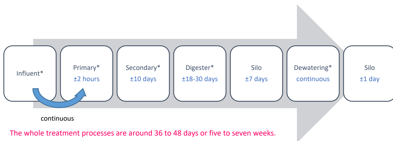
Figure A-70. Common treatments timeline at the wastewater treatment plants
