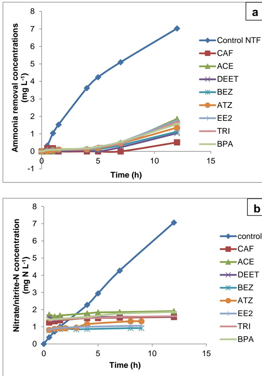
**Figure 5.2** The nitrification performance that shown as ammonium removal (a) and nitrate/nitrite-N generation (b) in the control NTF without CoC challenge and the NTFs challenged with individual CoC.
