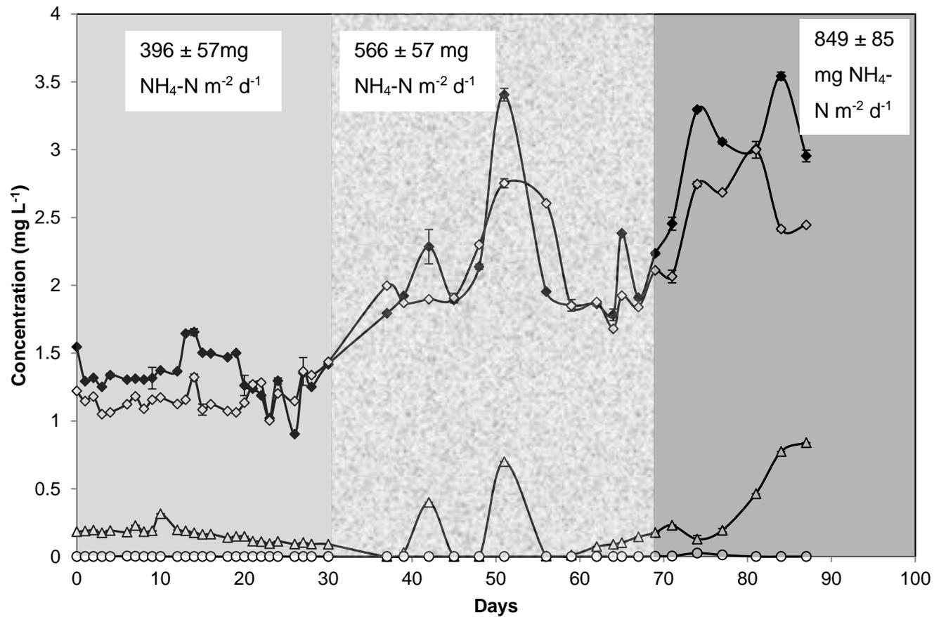
**Figure 3.4** Long term nitrification monitoring in the short filter with feeding low concentrations of ammonium (1.0–4.0 mg NH<sub>4</sub>-N L<sup>-1</sup>). Data points show average concentration ± SD of influent ammonium-N (◆), effluent ammonium-N (◇), nitrate-N (△) and nitrite-N (○). Shade areas indicate different ammonium surface loading rate ranges.
