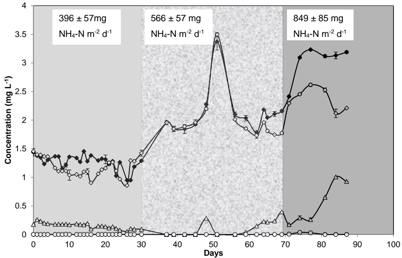
**Figure 3.3** Long term nitrification monitoring in the tall filter with feeding low concentrations of ammonium (1.0–4.0 mg NH<sub>4</sub>-N L<sup>-1</sup>). Data points show average concentration  $\pm$  SD of influent ammonium-N (◆), effluent ammonium-N (◇), nitrate-N (△) and nitrite-N (○). Shade areas indicate different ammonium surface loading rate ranges.
