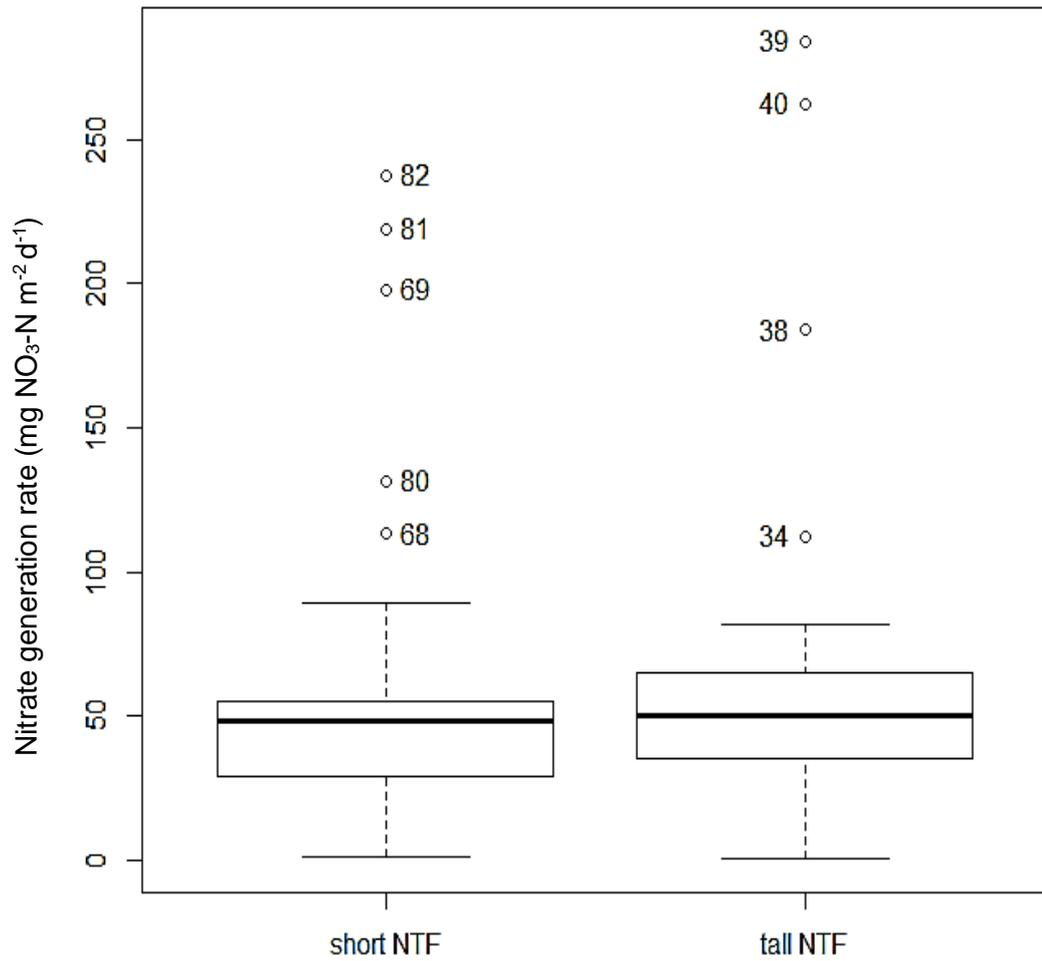
**Figure 3.6** Nitrification performances, presented as nitrate-N generation rate ( $\text{mg NO}_3\text{-N m}^{-2} \text{d}^{-1}$ ), of the tall and short NTFs. The bold lines present mean values of nitrate-N generation rates for both NTFs.
