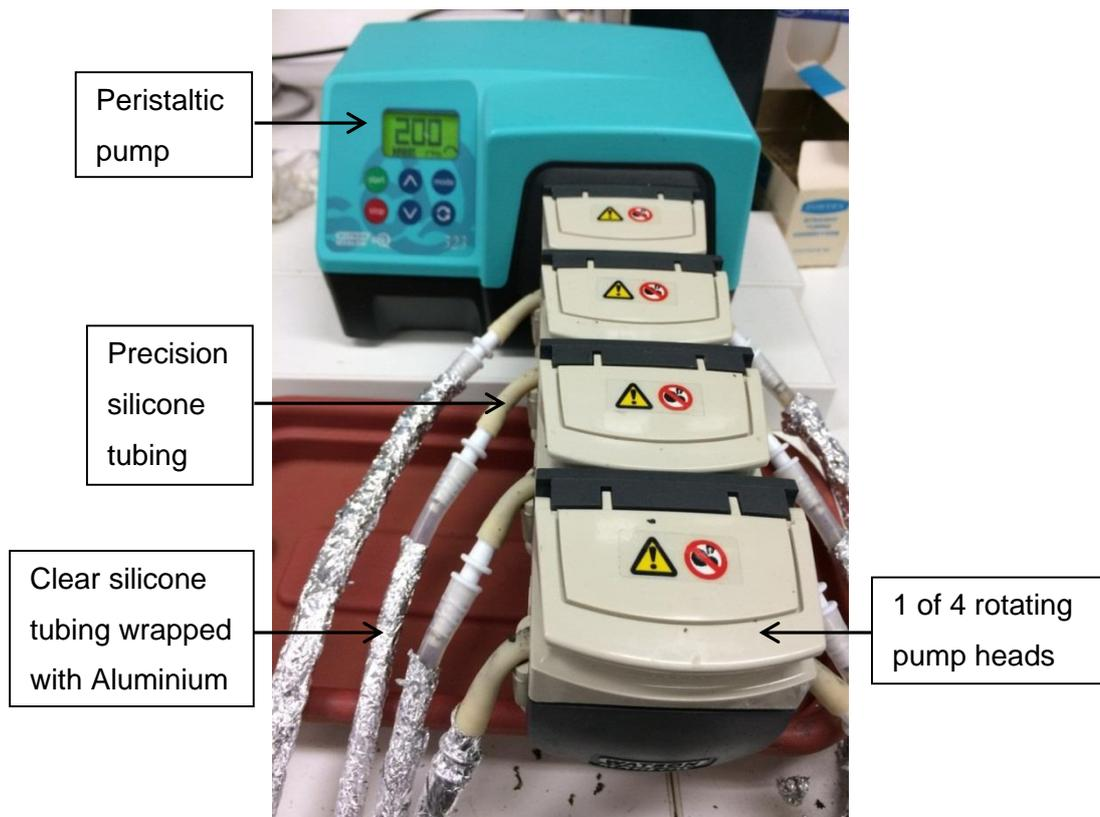
**Plate 2.11** The peristaltic pump used for water circulation.
