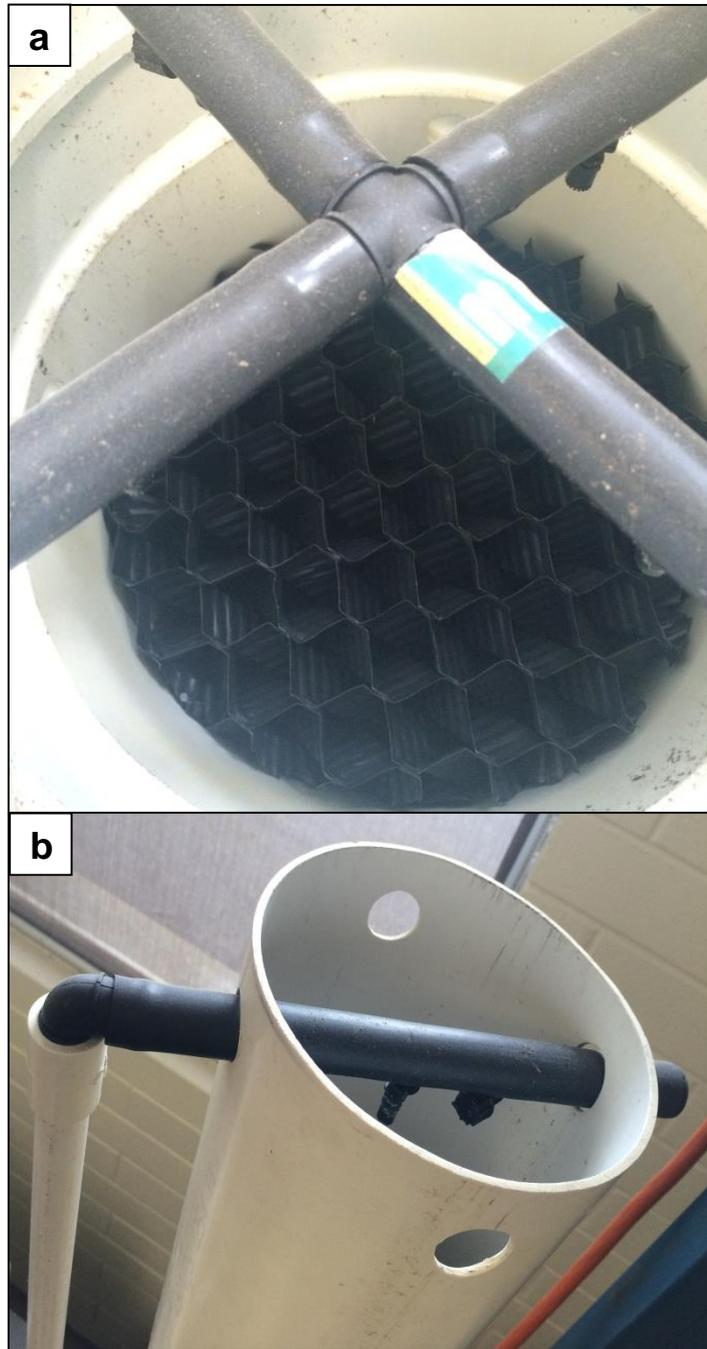
**Plate 2.7** Distribution system for NTFs: (a) Cross sprinklers distribution for the short NTF, (b) two sprinklers for the tall NTF distribution.
