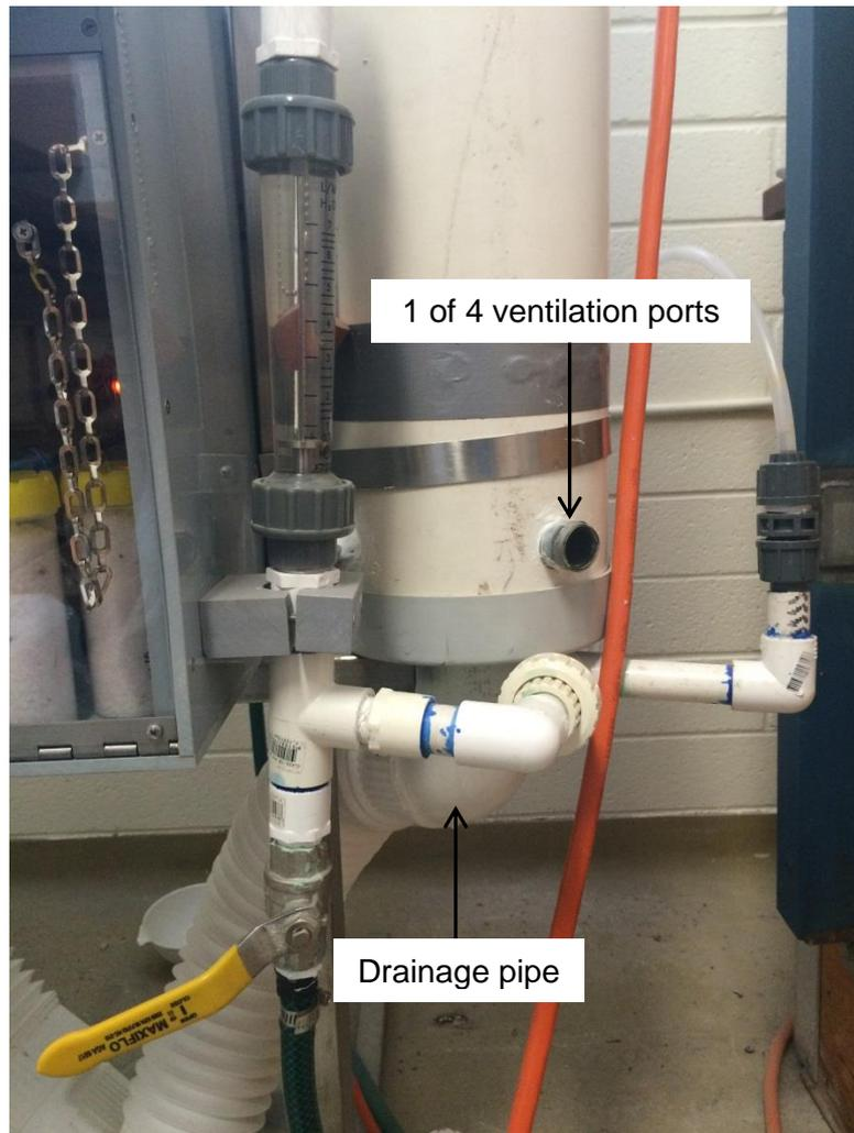
**Plate 2.8** The drainage pipe and ventilation ports of NTFs.
