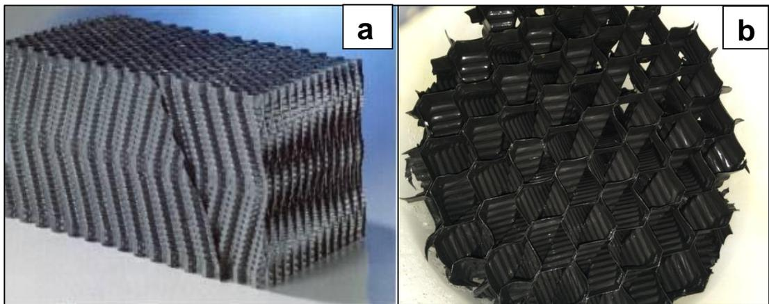
**Plate 2.5** (a) Photograph of polypropylene media (2H Plastics, Australia); (b) the polypropylene media positioned in NTF column.
