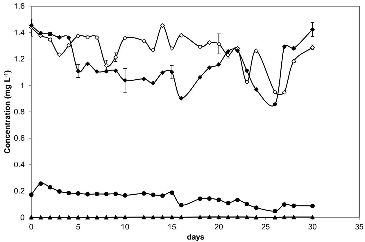
**Figure 3.1** Nitrification performance in the tall filter during start-up fed with low concentrations ( $1.4 \pm 0.2$  mg  $\text{NH}_4\text{-N L}^{-1}$ ) of ammonium. Data points show average concentrations  $\pm$  SD of influent ammonium-N ( $\diamond$ ), effluent ammonium-N ( $\blacklozenge$ ), nitrite-N ( $\blacktriangle$ ) and nitrate-N ( $\bullet$ ).
