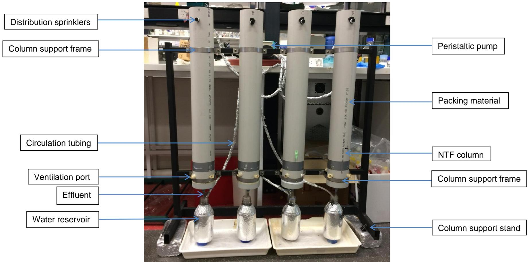
**Plate 2.9** Four parallel NTFs in the laboratory.
