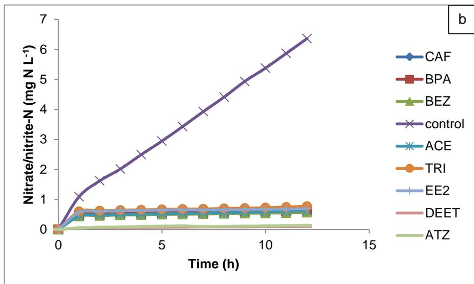
**Figure 4.4** Nitrification performance that shown as ammonium removal (a) and nitrate/nitrite-N generation (b) in the control NTF and the NTFs in the presence of individual CoC.
