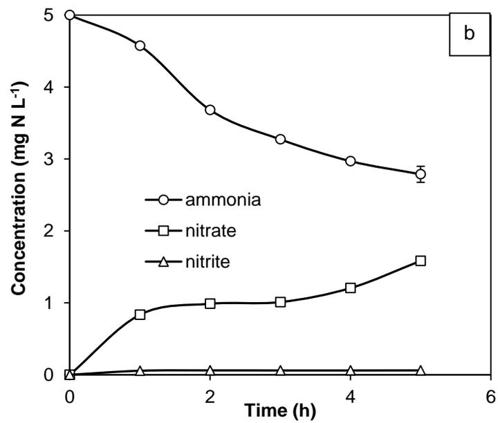
**Figure 6.2** Nitrification performance in the NTFs fed 5 mg NH<sub>4</sub>-N L<sup>-1</sup> and operated under different experimental conditions: (a) representative inorganic nitrogen profiles in the NTFs over 5 h following ammonia addition in the absence of exogenous organic carbon; (b) representative inorganic nitrogen profiles in the NTFs over 5 h in the presence of ammonium (5 mg NH<sub>4</sub>-N L<sup>-1</sup>) and sucrose (75 mg L<sup>-1</sup>)
