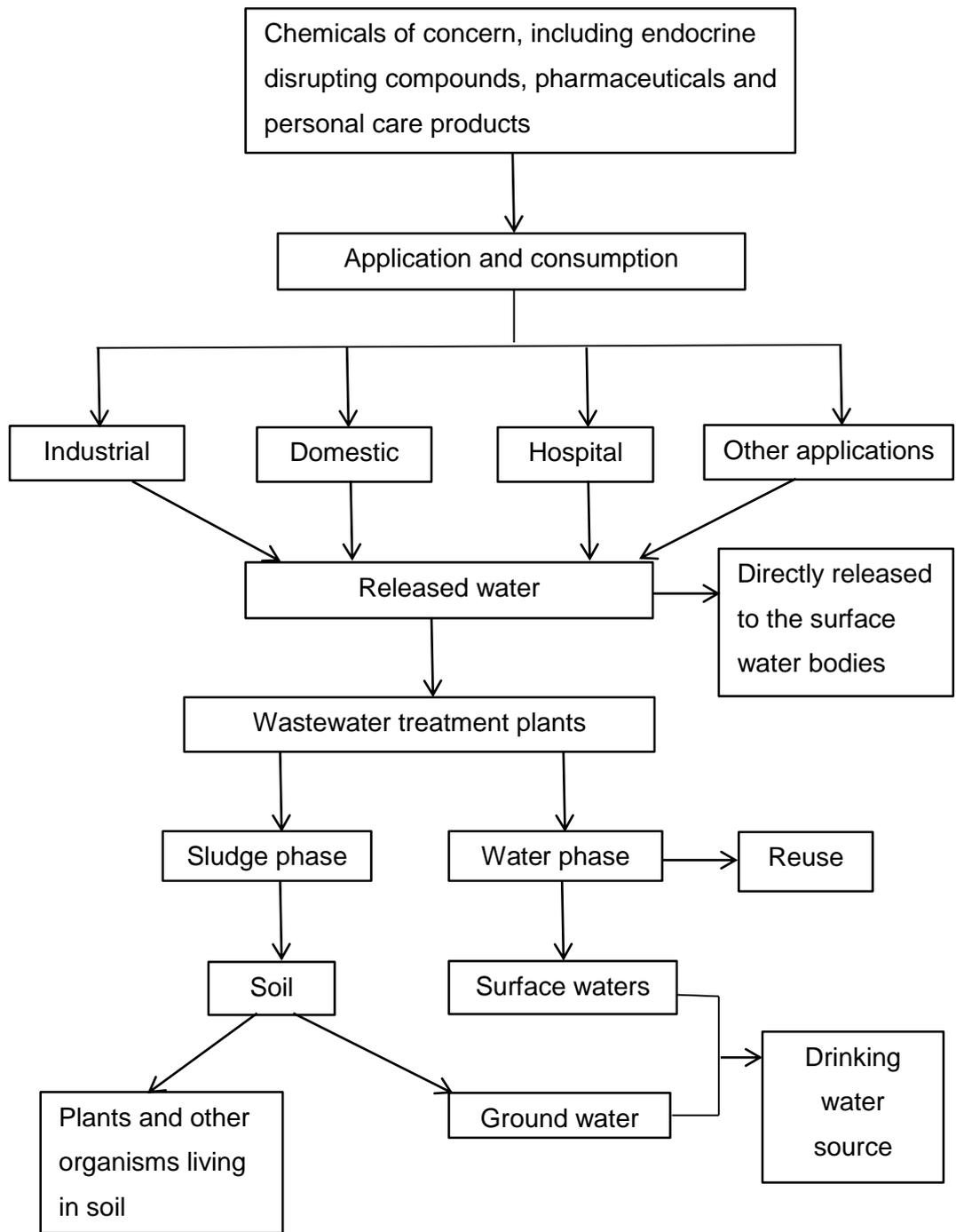
**Figure 1.2** Theoretical distribution of CoC in the environment.
