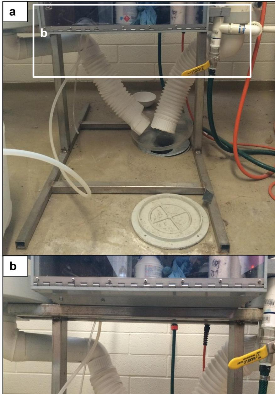
**Plate 2.2** Support stand for NTFs: (a) Overview of the NTFs support stand structure; (b) The cross-strut, on which the filters sit.
