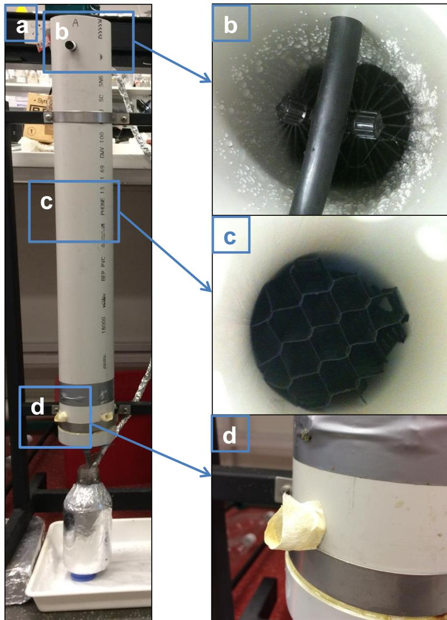
**Plate 2.10** Detailed NTF construction: (a) one of the four parallel NTF columns; (b) water distribution; (c) packing material; (d) one of the four ventilation ports for each column.
