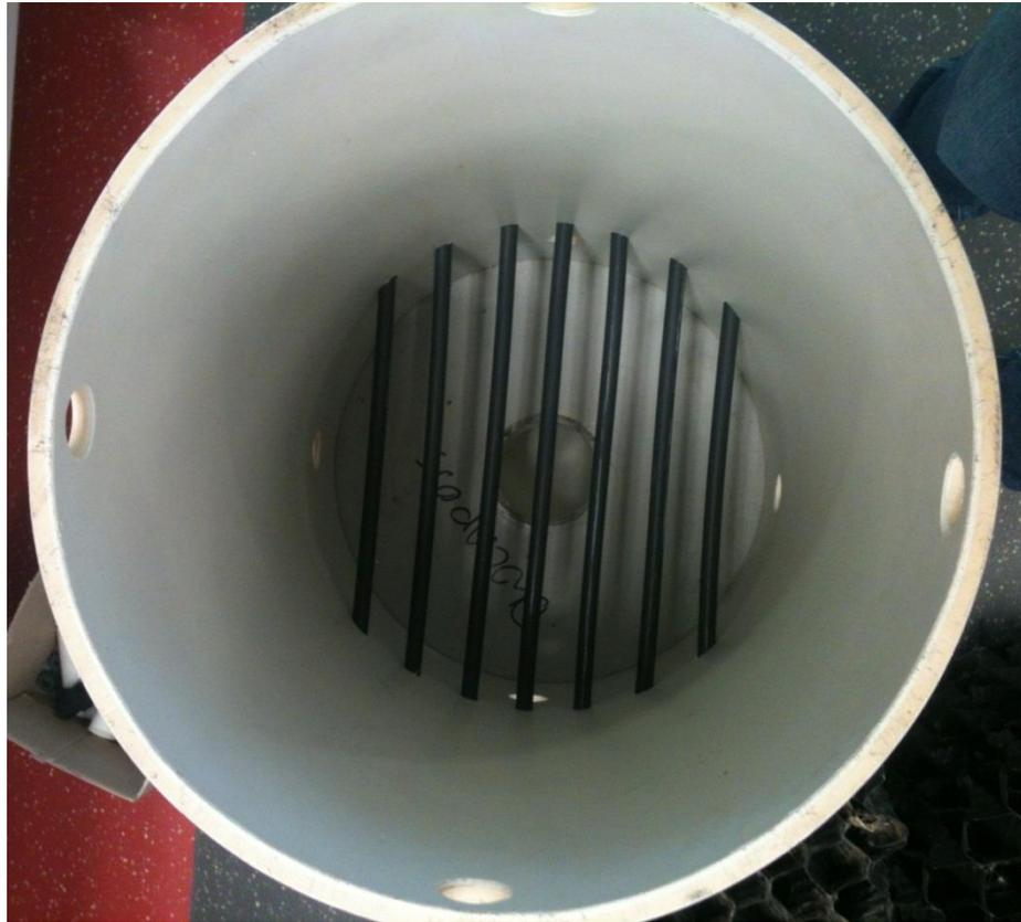
**Plate 2.4** The media support stand positioned inside the NTF.
