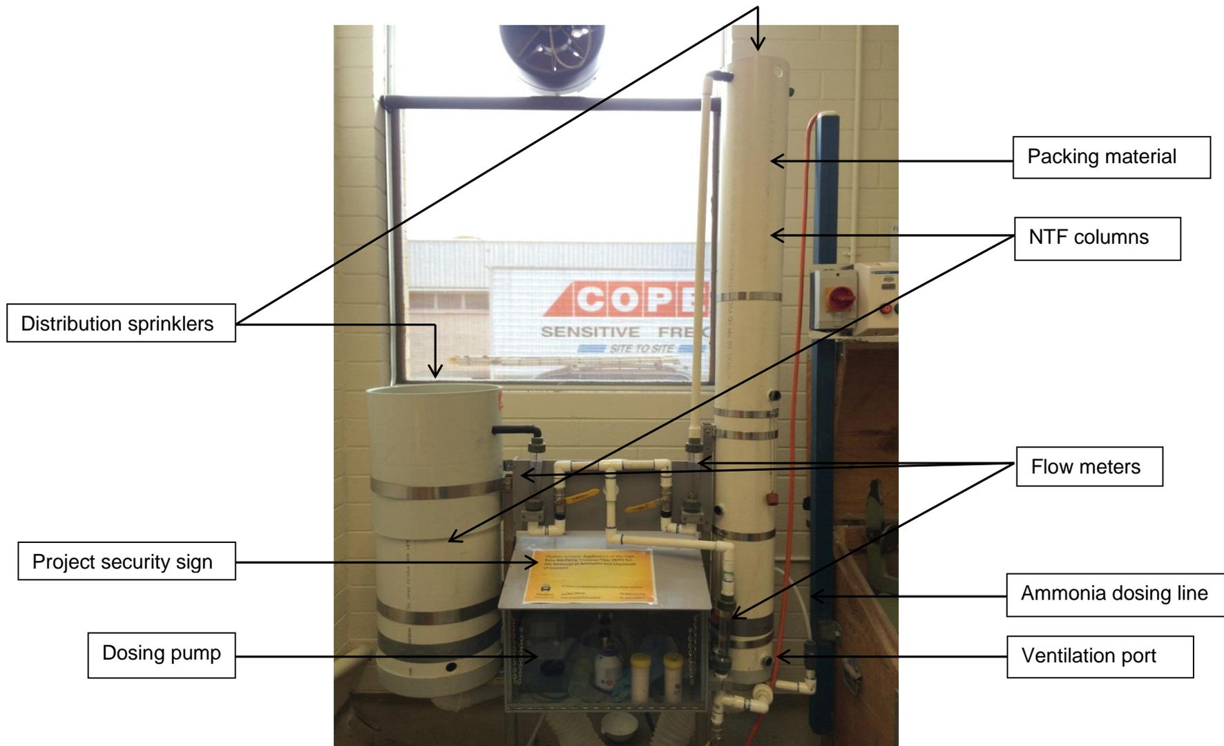
**Plate 2.1** Two laboratory-scale NTFs of different aspect ratios and containing the same filter packing medium specific surface area.
