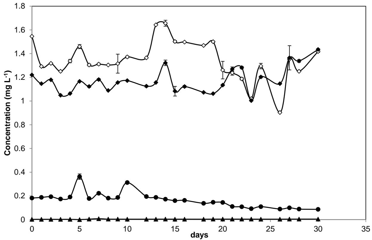
**Figure 3.2** Nitrification in the short filter during start-up, fed with low concentrations ( $1.4 \pm 0.2$  mg NH<sub>4</sub>-N L<sup>-1</sup>) of ammonium. Data points show average concentration  $\pm$  SD of influent ammonium-N ( $\diamond$ ), effluent ammonium-N ( $\blacklozenge$ ), nitrite-N ( $\blacktriangle$ ) and nitrate-N ( $\bullet$ ).
