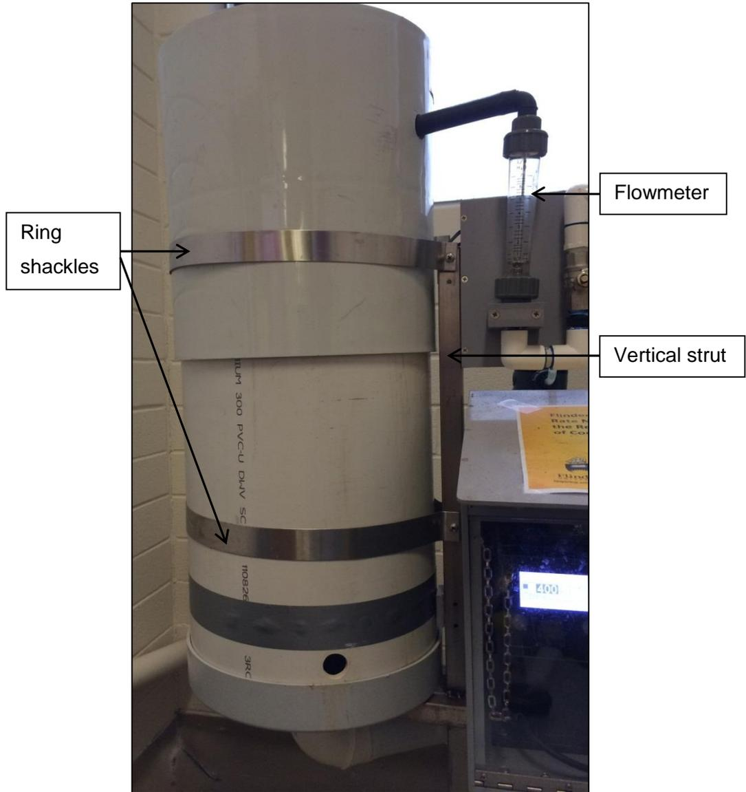
**Plate 2.3** The support frames for NTFs.
