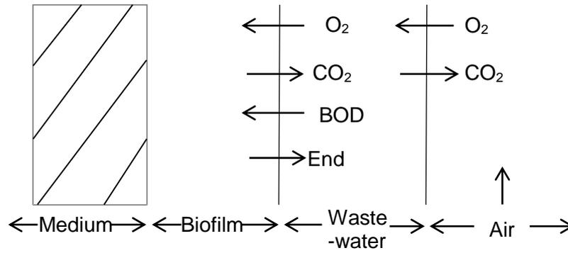
**Figure 1.1** A schematic representation of the biological film in a trickling filter.
