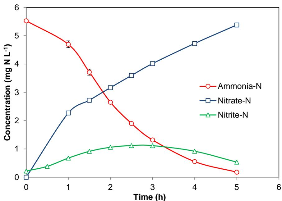
**Figure 5.1** The typical nitrification performance, presented as the concentration changes of ammonia-N, nitrate-N and nitrite-N, in the four parallel NTFs before challenging with CoC. (All data points show means ± 1 SD)
