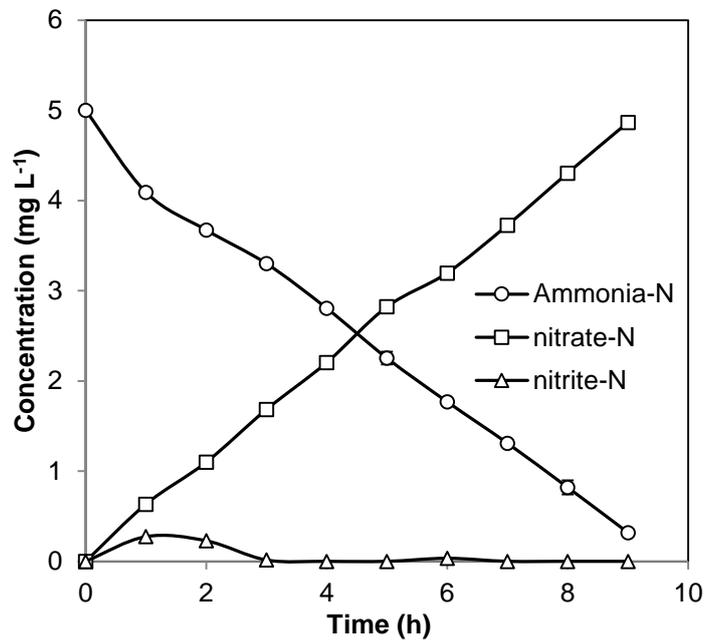
**Figure 4.3** Representative ammonium-N ( $\text{mg NH}_4\text{-N L}^{-1}$ ) removal against time in a recirculating NTF fed a solution of  $5 \text{ mg NH}_4\text{-N L}^{-1}$  in the absence of CoC, and the removal rate was  $0.52 \pm 0.15 \text{ mg NH}_4\text{-N L}^{-1} \text{ h}^{-1}$ . All data points present parameter means  $\pm 1 \text{ SD}$ .
