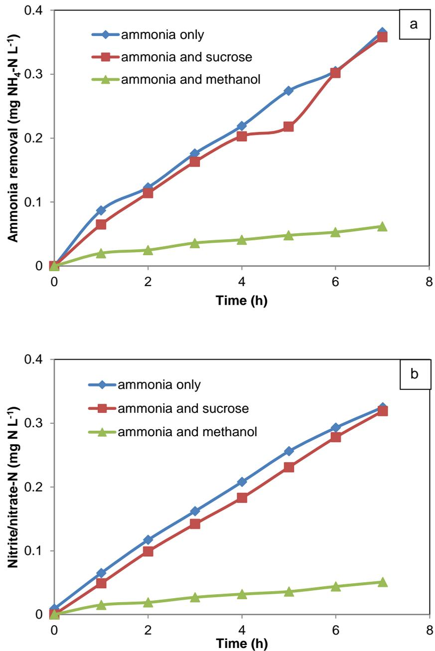
**Figure 6.1** Nitrification performance shown as ammonium removal (a) and nitrite/nitrate-N generation (b) after 7 hours recirculation in the NTF under three experimental conditions: ammonia only (5 mg NH<sub>4</sub>-N L<sup>-1</sup>), ammonia (5 mg NH<sub>4</sub>-N L<sup>-1</sup>) with sucrose (75 mg L<sup>-1</sup>) and ammonia (5 mg NH<sub>4</sub>-N L<sup>-1</sup>) with methanol (1 mL in 1 L recirculating water).
