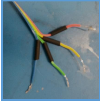
Figure 3-37: Heat shrink wrap placed onto each of the four wires.
