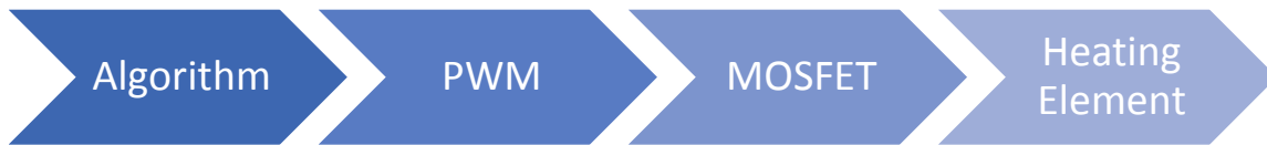
Figure 3-18: Process required to turn the heating elements on and off.
