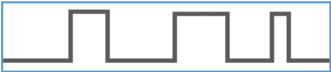
Figure 5-6: Example stimulus applied during a pseudo-random binary sequence test ( How to Perform a Step Test - Control Station , no date).
