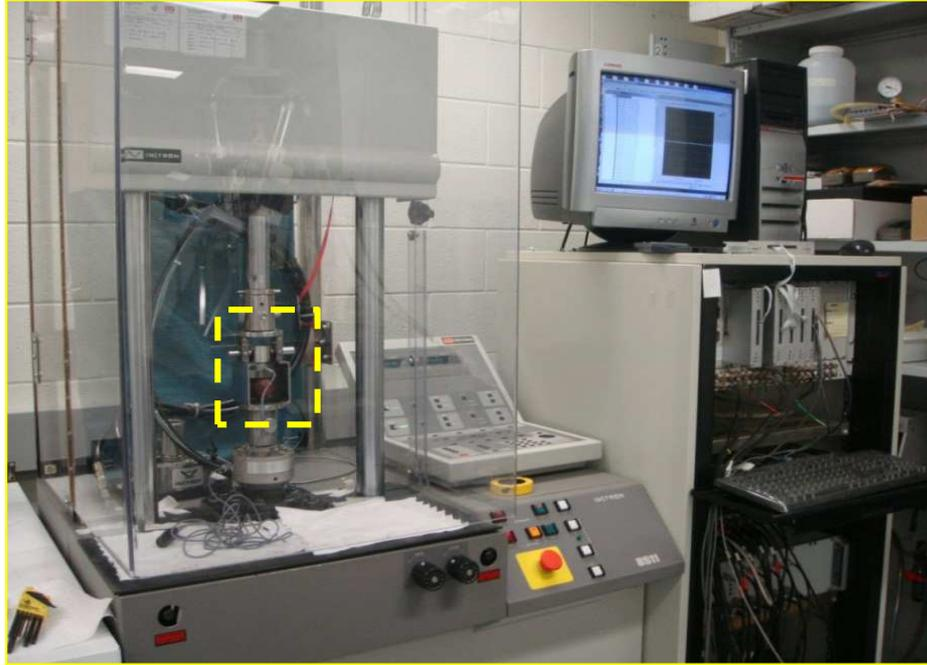
Figure 6.1: A mechanical testing machine (Model 8511, Instron Pty. Ltd., High Wycombe, UK) was in operation for the pullout test and the acquisition software displayed on the computer screen captured the displacement of screw and pullout force ( $F_{\text{Pullout}}$ ) data. A custom-made fixture was mounted onto the testing machine (illustrated inside the yellow dotted box) to firmly grip the specimen during testing.
