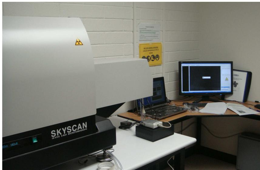
Figure 5.16: The high resolution micro-computed tomography (micro-CT) scanner (Skyscan model 1076, Skyscan, Kontich, Belgium) that was used in this study. It has capability for in vivo and ex vivo scanning of small animals and bone specimens.
