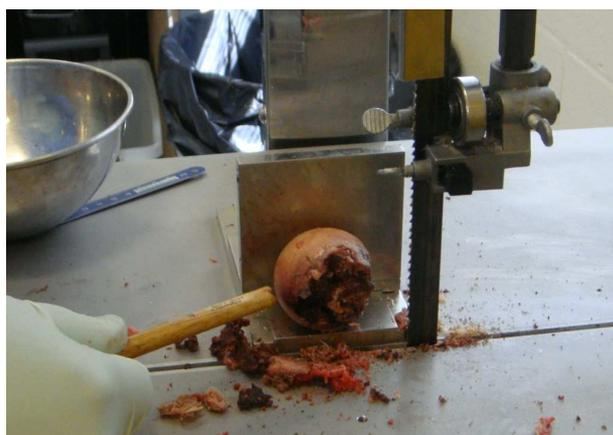
Figure 5.1: A floor-standing bandsaw was used to cut the excised femoral heads from the femoral neck, level jagged edges, and trim off remnants of soft tissues, to allow easy access for the insertion of the cancellous screw into the femoral head specimens.
