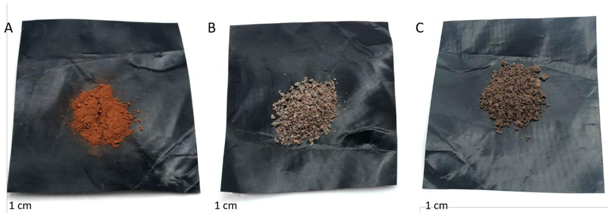
**Figure 181** – **A**) 0.1 grams of  $\gamma$ -Fe<sub>2</sub>O<sub>3</sub> nanoparticles (<50nm), **B**) 0.65 grams of 50-poly(S-*r*-canola) polysulfide, **C**) 0.75 grams of 50-poly(S-*r*-canola) /  $\gamma$ -Fe<sub>2</sub>O<sub>3</sub> composite material.
