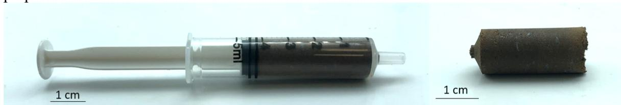
**Figure 186** – Syringe containing un moulded composite (Left) and the resulting moulded composite cylinder (Right).
