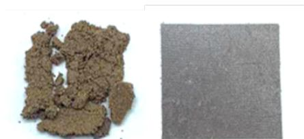
**Figure 88** – Image showing 50-poly(*S-r*-canola) before and after moulding for 10 minutes at 10 MPa, 100 °C.
