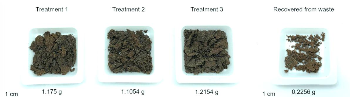
**Figure 175** – Images showing the composite material directly after magnetic filtration / separation from the sand / water slurry.
