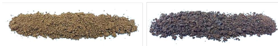
**Figure 81** – Images showing 50-poly(*S-r*-canola) before (left) and after (right) being heated for 24 hours at 110 °C.
