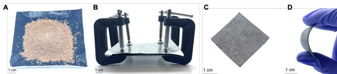
**Figure 82** – **A)** 50-poly(*S-r*-canola) particles on a metal sheet separated by PTFE paper. **B)** Compression system used to compress the 50-poly(*S-r*-canola) particles into direct contact. **C)** Section of mat prepared using reactive compression moulding. **D)** Image demonstrating the flexibility of the mats.
