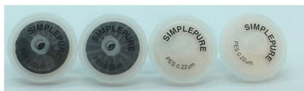
Figure 5. Carbon-polymer blend is easier to remove from water by filtration than either PAC or GAC. Left to right: syringe filter clogged with GAC (GC 1200, 0.5–0.7 mm, Activated Carbon Technologies), syringe filter clogged with PAC (Kuraray, PGW 150 MP), syringe filter used to filter the carbon-polymer blend (no clogging), and an unused syringe filter.
