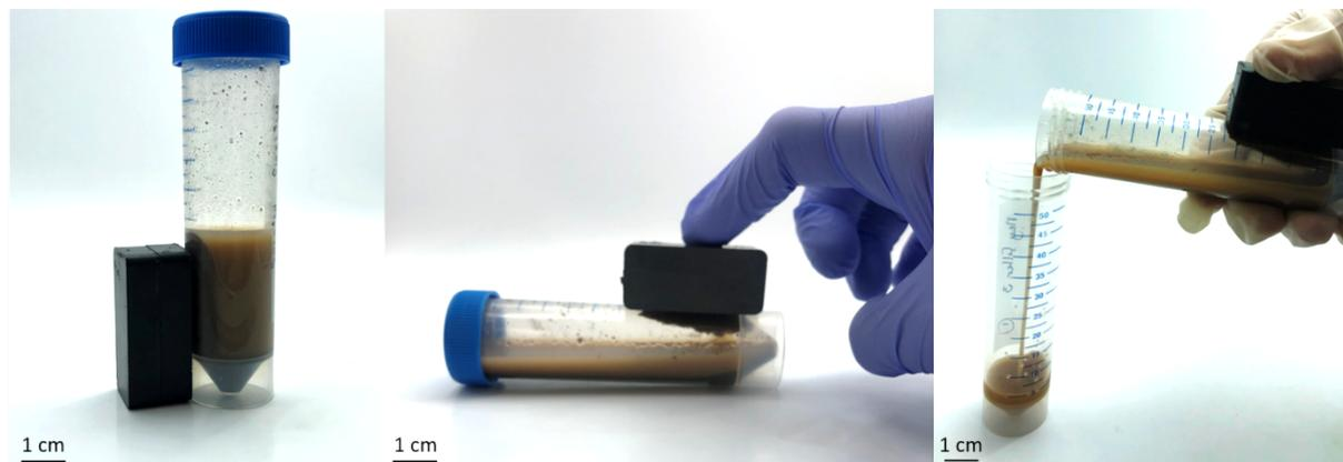
**Figure 174** – Images demonstrating the magnetic filtration and separation of the composite powder from a tailings / water slurry.
