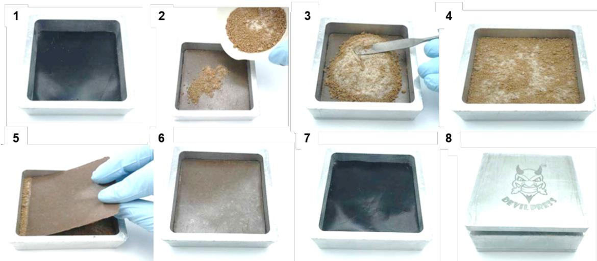
**Figure 131** – Images showing step-by-step process to prepare the sand composites using the method described above.
