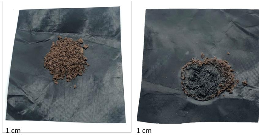
**Figure 183** – Image showing the magnetic composite before (left) and after (right) 50 seconds of microwave irradiation. This demonstrates that under 50 seconds of irradiation the composite will start to decompose.
