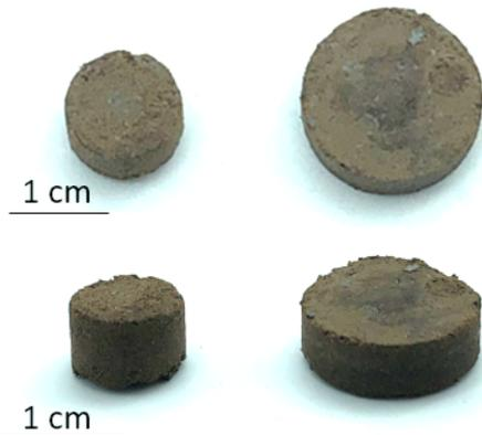
**Figure 185** – Images showing the composite disks made from the magnetic composite using reactive compression moulding in the microwave.
