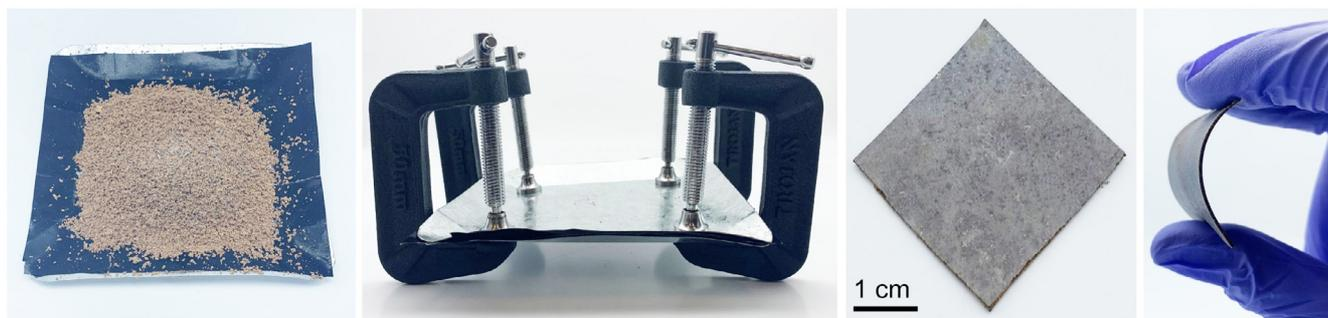
**Figure 1.** A) Heating 20 g of 50-poly(*S-r*-canola) in a beaker at 110 °C for 24 hours in an oven does not result in melting and the polymer is recovered as a slightly darkened powder. B) Heating 20 g of polymer between two PTFE sheets and metal plates, with pressure applied from C-clamps, results in the formation of a monolithic and flexible rubber mat (110 °C, 24 h, oven).
