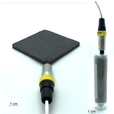
**Figure 164** – Image showing the samples with probe inserted for thermal conductivity measurement.
