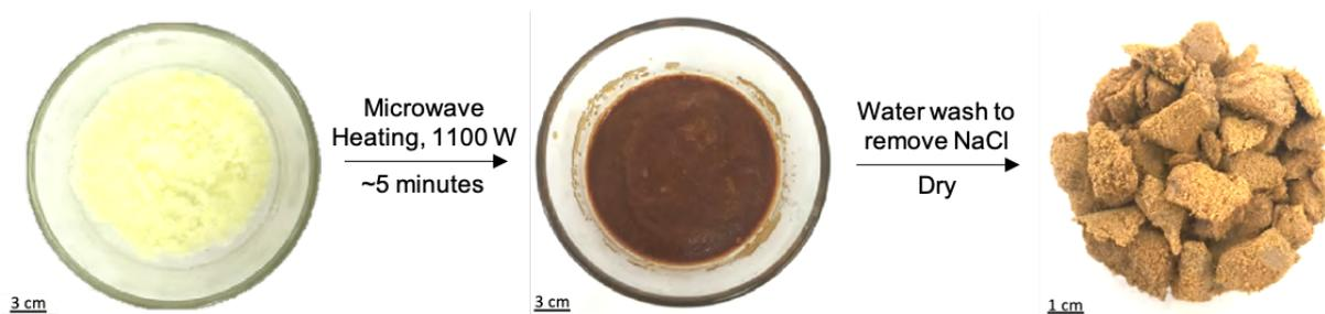
**Figure 52** – Images of reaction mixture in bowl before (left) and after (middle) inverse vulcanization in a household microwave for ~5 minutes and the porous 50-poly(*S-r*-canola) product after washing to remove salt.
