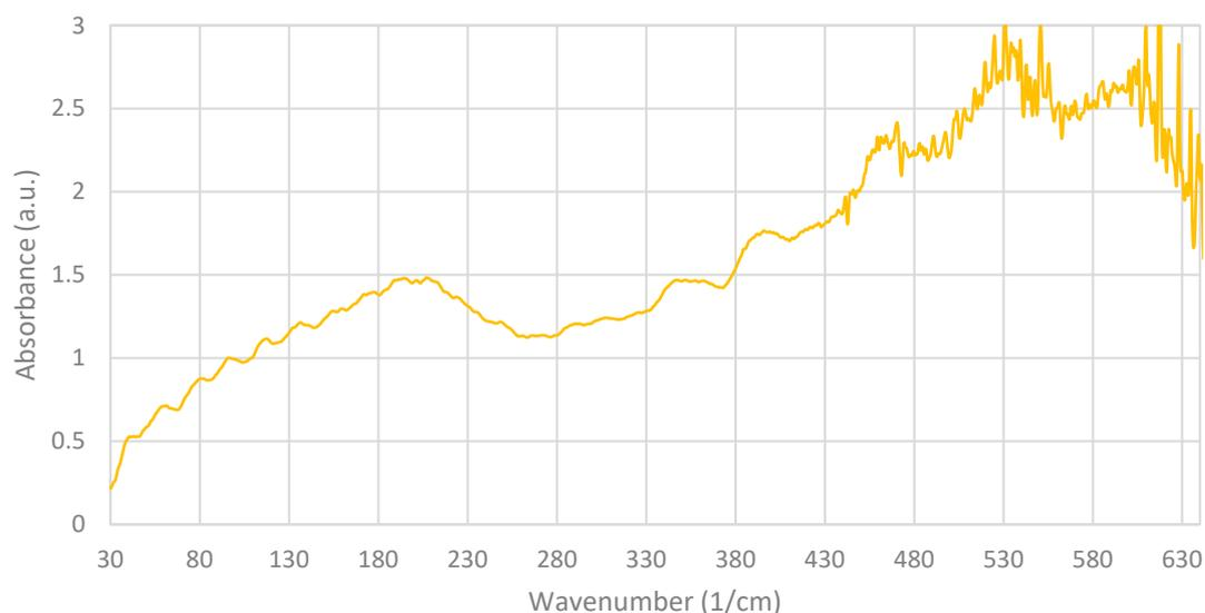
**Figure 4-33: FIR spectrum of pressed bilirubin conjugate in paraffin wax pellet (1:2.5 ratio mix), analysed at the Australian Synchrotron (THz/FIR Beamline) using a SiBolo detector with amplitude of 1370.**
