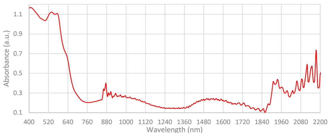
**Figure 4-130: UV-Vis.-NIR reflectance spectrum of previously refrigerated neat sheep's blood (reference: centrifuged serum), analysed using a UV-Vis.-NIR Lambda 950 Spectrophotometer at Flinders University.**
