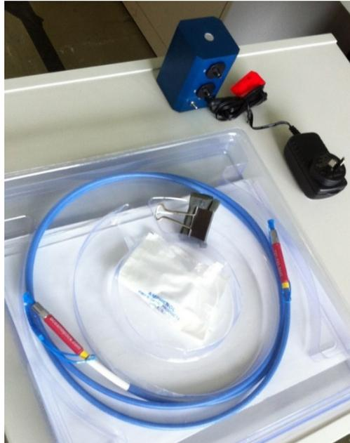
**Figure 3-3: ISP-REF Integrating Sphere shown here with the aperture upwards. Also shown is the sphere's fiber optic cable and bulldog clip utilised for the novel setup when coupled to the ASD FieldSpec.**
