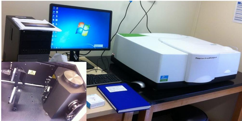
**Figure 3-1:** Perkin Elmer UV-Vis.-NIR Lambda 950 Spectrophotometer setup with the 150 mm integrating sphere accessory. Inset: open sample compartment for 150 mm integrating sphere accessory showing the vertical reference sample port.
