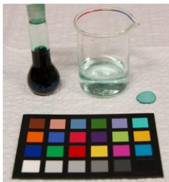
Figure 4-142: Biliverdin at 2.28 mg/mL in PBS (volumetric flask), diluted in PBS (beaker) and a reflectance sample of the 2.28 mg/mL biliverdin in PBS solution (circular filter paper).
