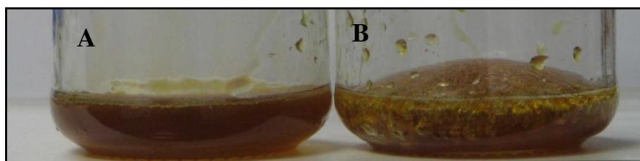
**Figure 3.19** Effect of Relative Humidity during curing of Castor oil and PMDI
