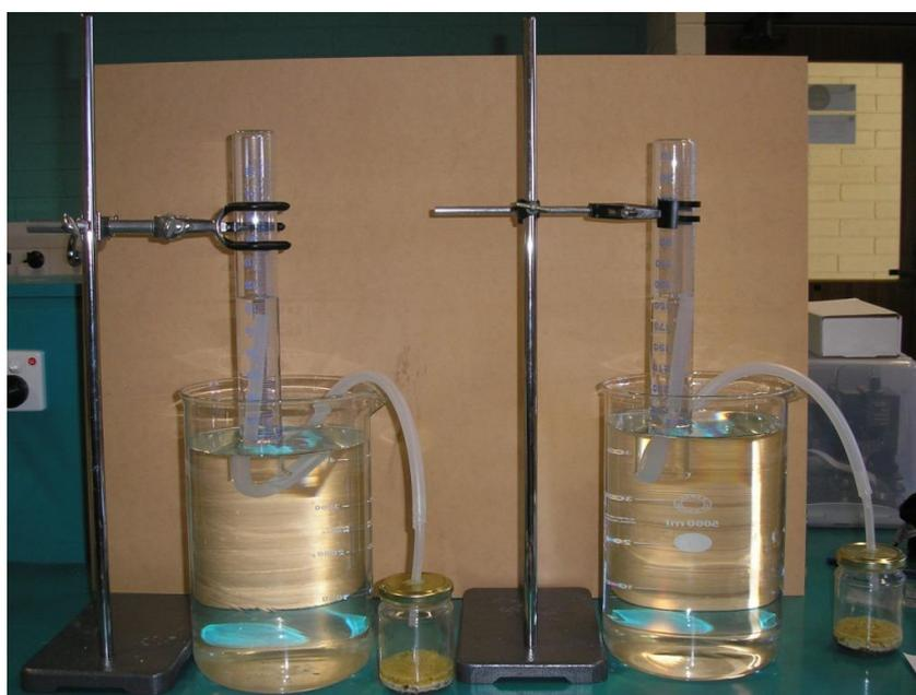
**Figure 2.4** CO<sub>2</sub> measurement apparatus
