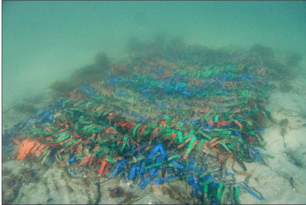
Figure 5 Fouled artificial seagrass fronds on James Matthews after 2 years on site. Courtesy of WAM.
