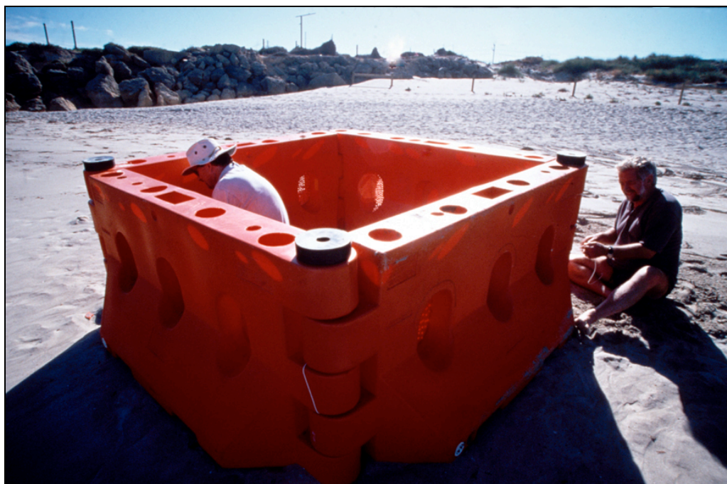
Figure 8 Crash-barrier trial square ex situ , prior to placement adjacent to James Matthews . Courtesy of WAM.
