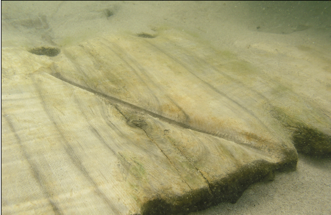
Figure 4.10: Additional evidence of salvage on Vessel A, grove measures 14 cm in length and 1 cm in width (La Barre 2015).
