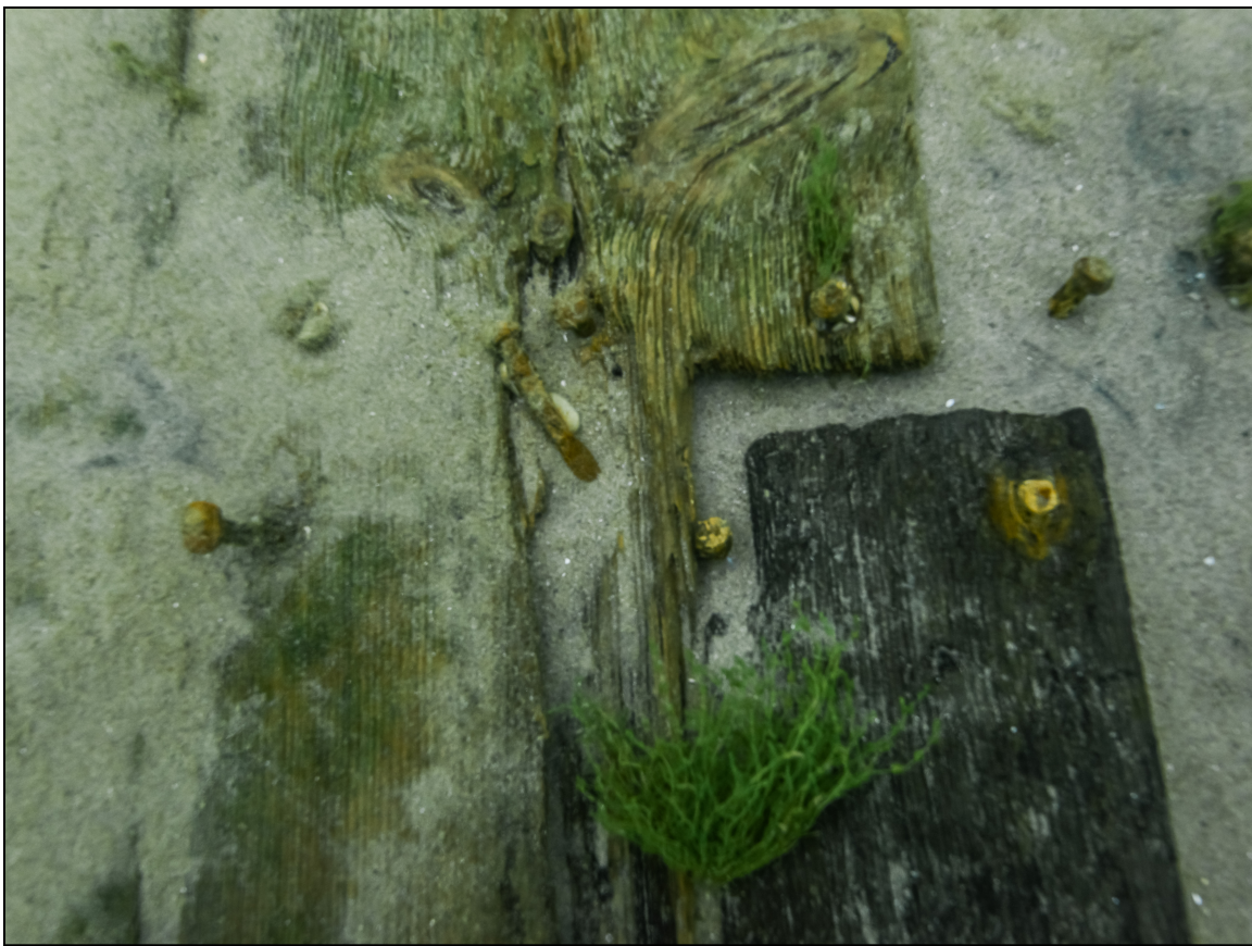
Figure 4.13: Intersection of changing ceiling planking material on Vessel B, darker plank measures 9 cm sided and 2.5 cm molded (La Barre 2015).
