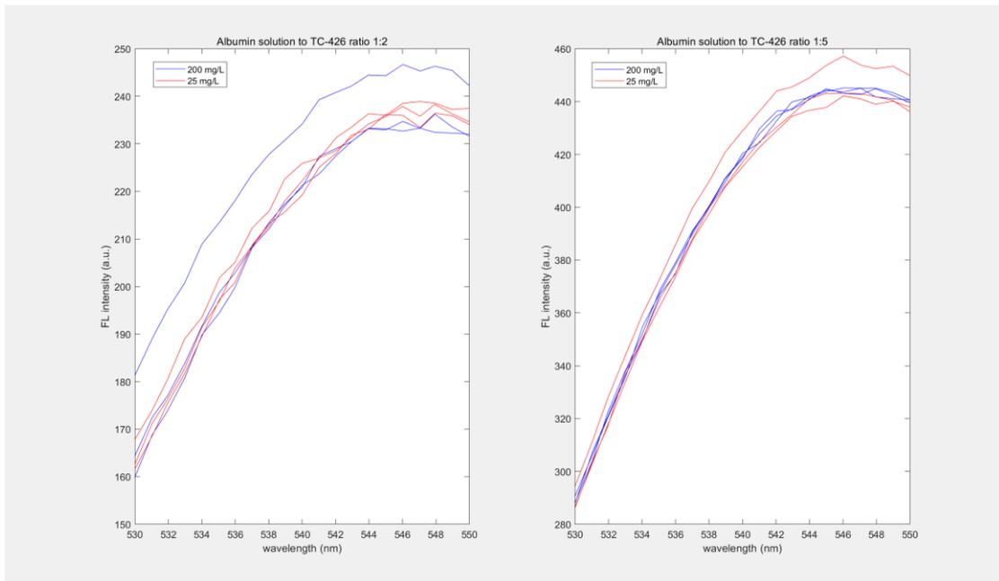
Figure 4.27 Result of TC-426 to albumin ratio 1:2 in real urine sample
