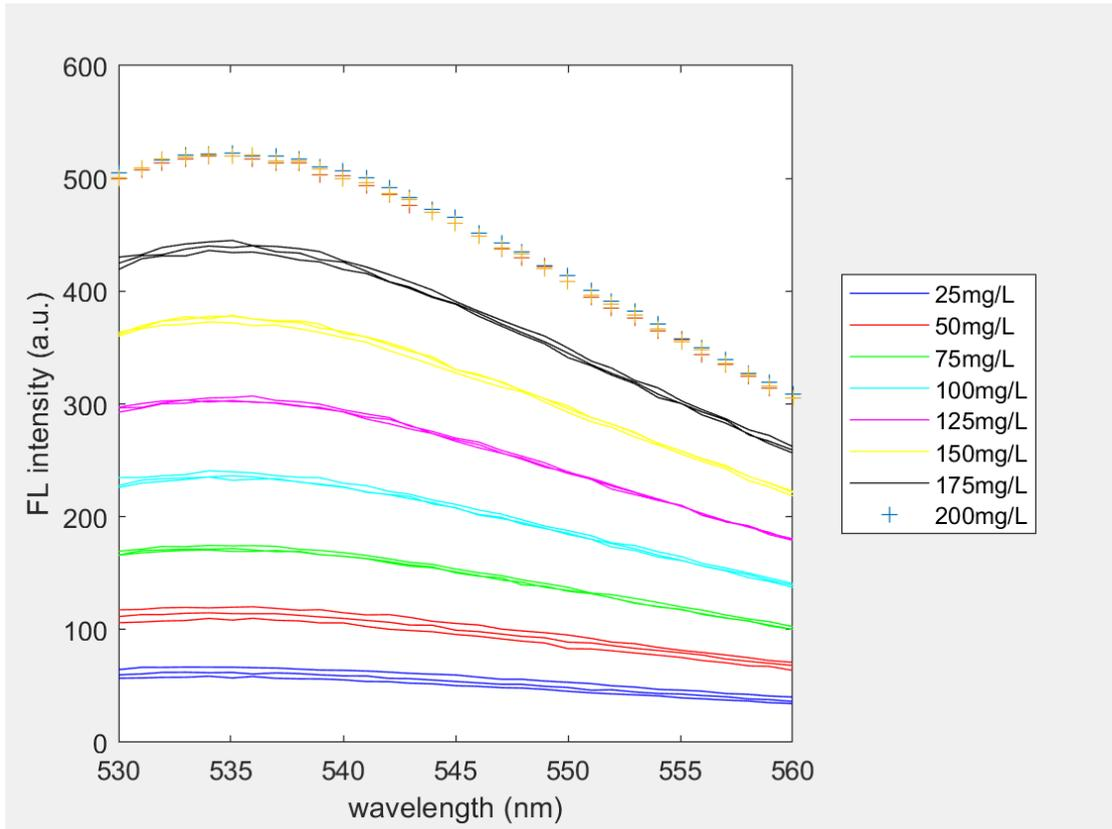
Figure 4.20 Results of albumin with different concentrations in artificial urine with the presence of creatinine
