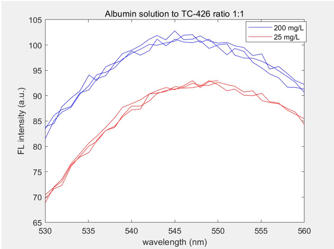
Figure 4.26 Result of TC-426 to albumin ratio 1:1 in real urine sample
