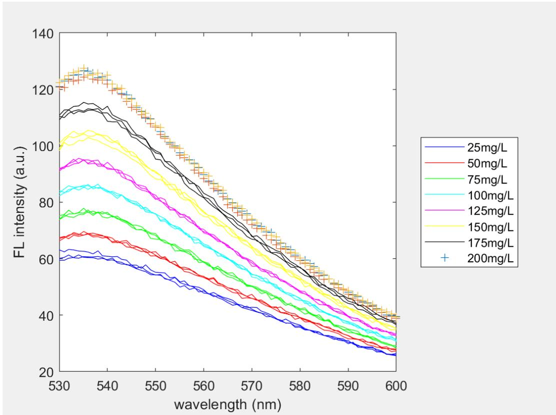
Figure 4.34 Results of albumin with different concentrations in real urine sample with the presence of creatinine
