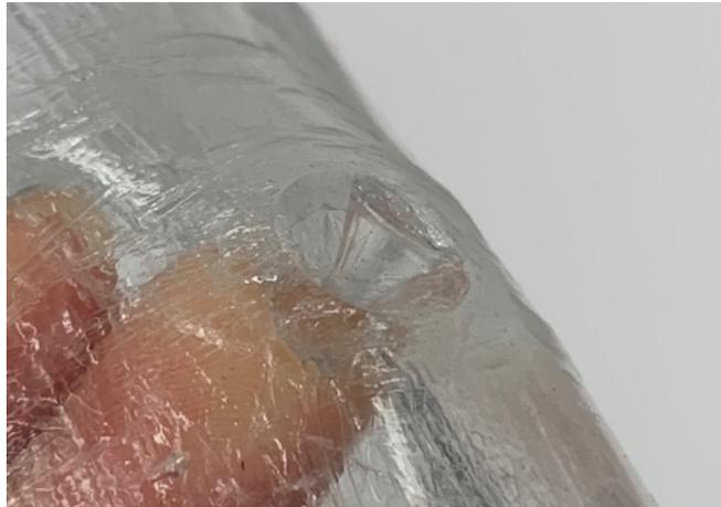
Figure 12: Punctured gelatine from pre-existing base plate holes
