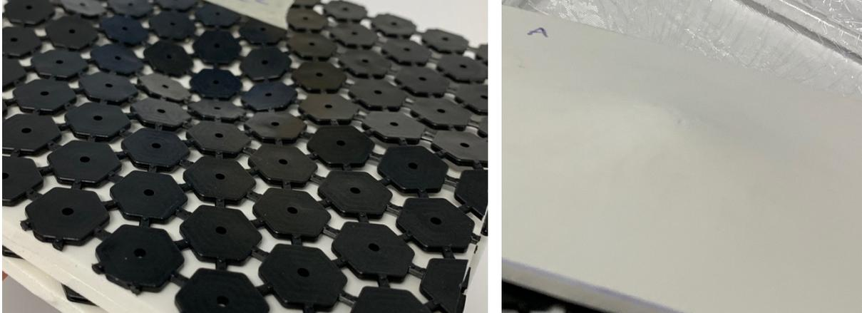
Figure 32: No visible hinge fractures in sample GAXAAX, resulting in a 619N increase between the first and third drop
