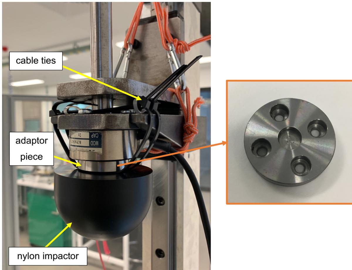
Figure 9: Nylon hemispherical impactor fixed onto sliding unit in drop tower
