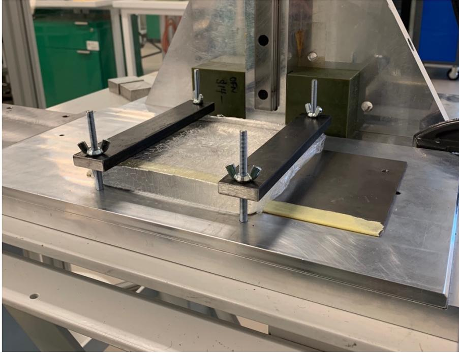
Figure 10: Fixation of gelatine sample on flat metal sheet with wing nut fasteners
