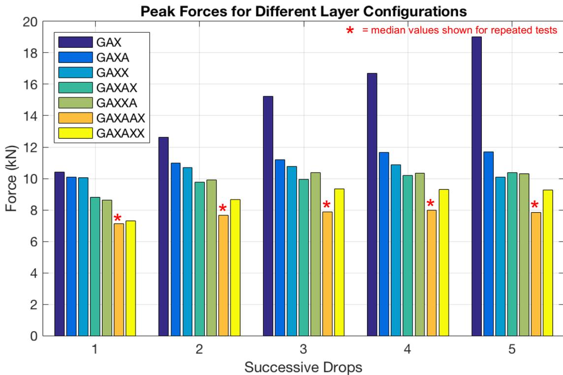
Figure 26: Comparison of peak forces for various configurations of Foam A and Isoblox X
