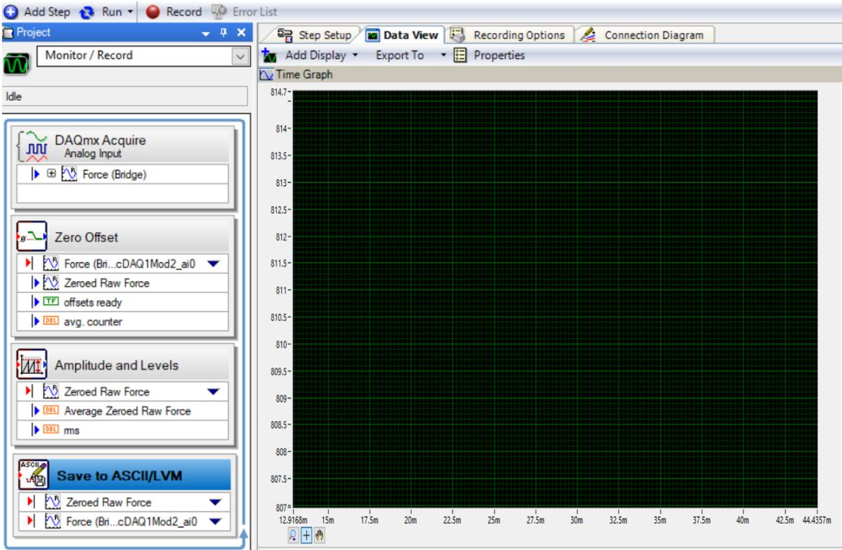
Figure 19: NI SignalExpress project used to capture load cell data
