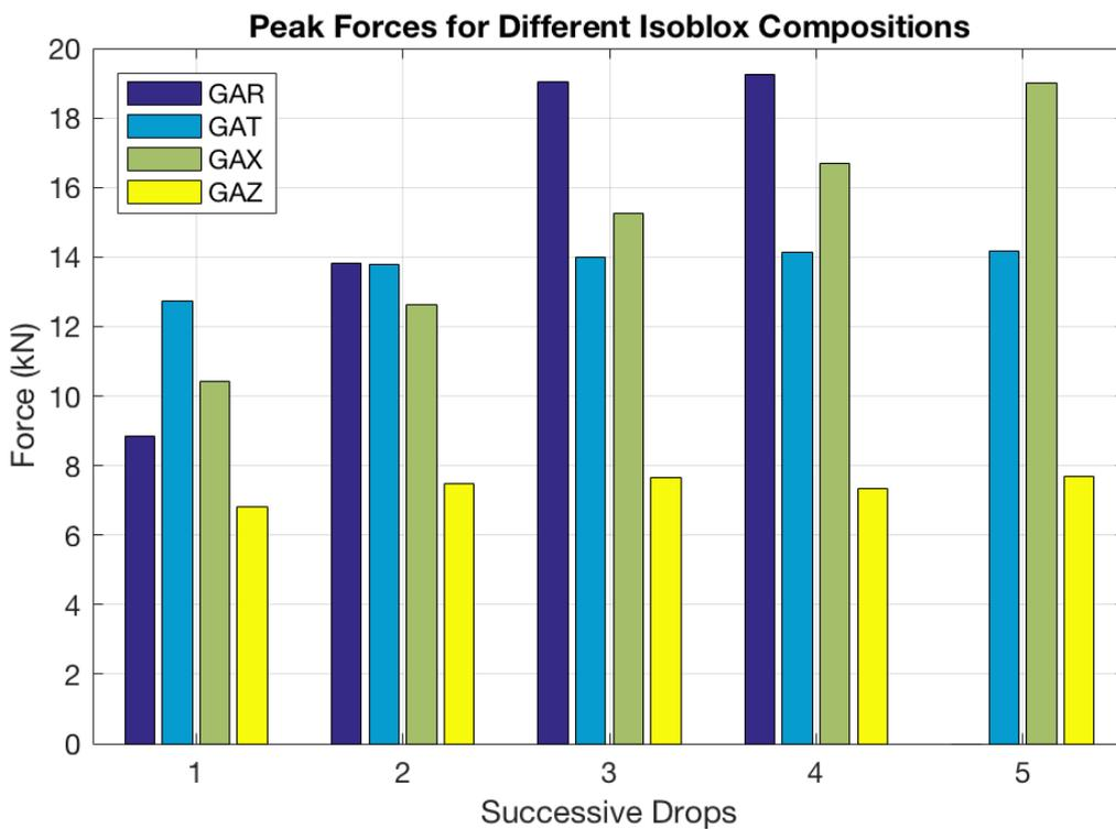
Figure 28: Comparison of peak forces for Isoblox compositions
