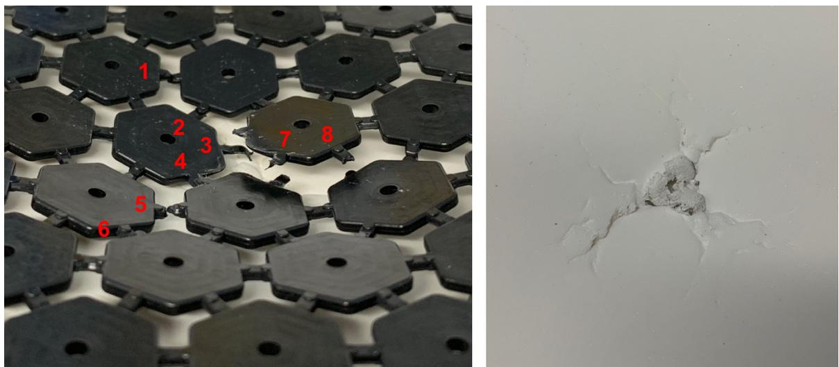
Figure 33: Sample GAX contained eight hinge fractures, reporting a 4833N increase between the first and third drop
