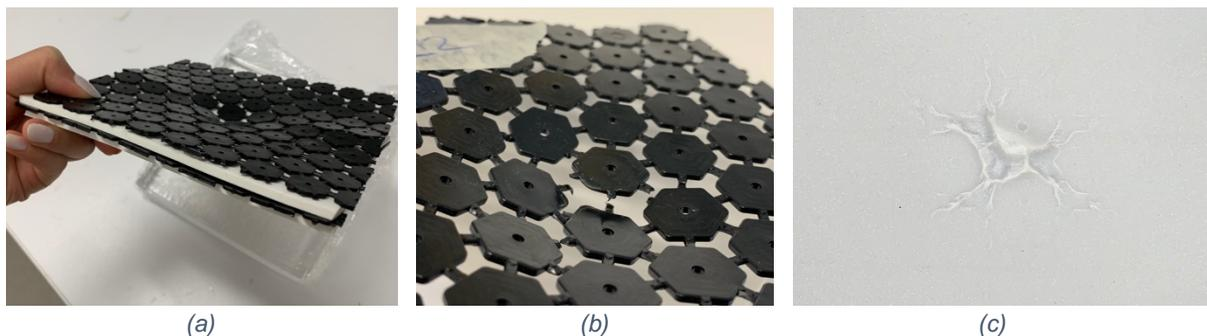
Figure 31: Damage to material samples in the form of (a) permanent Isoblox deformation, (b) Isoblox hinge fracture, and (c) foam deformation
