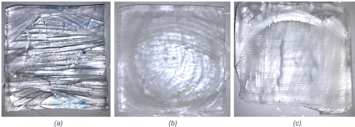
Figure 14: Uneven gelatine slices obtained by cutting by (a) knife, (b) wire, and (c) hacksaw
