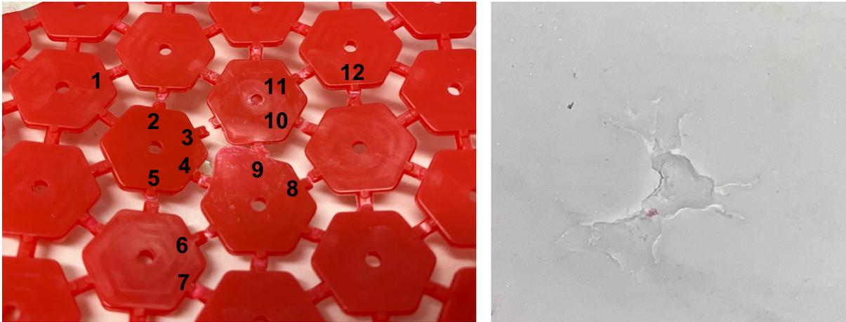
Figure 34: Sample GAR contained twelve hinge fractures, reporting a 10186N increase between the first and third drop
