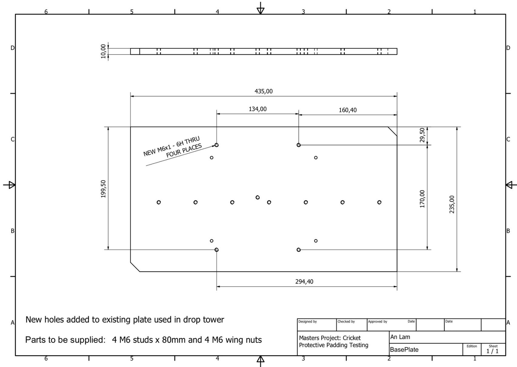
New holes added to existing plate used in drop tower
