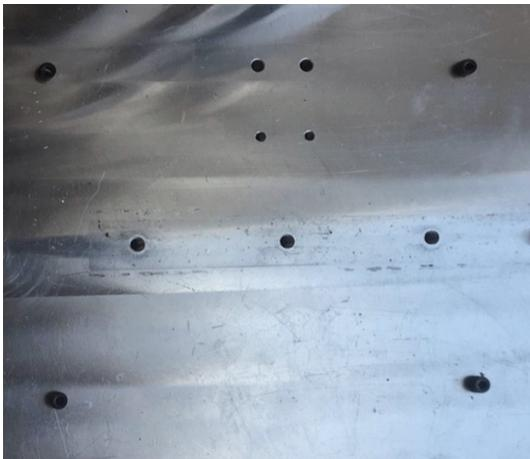
Figure 11: Exposed holes in drop tower base plate
