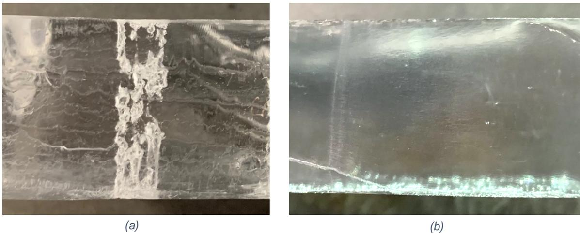
Figure 29: (a) Damage observed after drop testing in all previous gelatine layers (b) No visible damage in gelatine layers tested with optimised samples GAXDZ and GADZ
