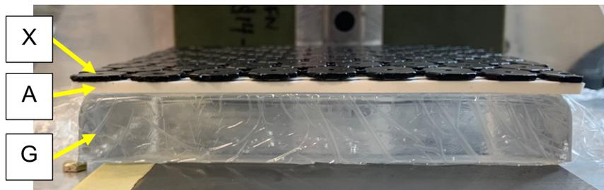
Figure 22: Sample GAX positioned on drop tower base plate
