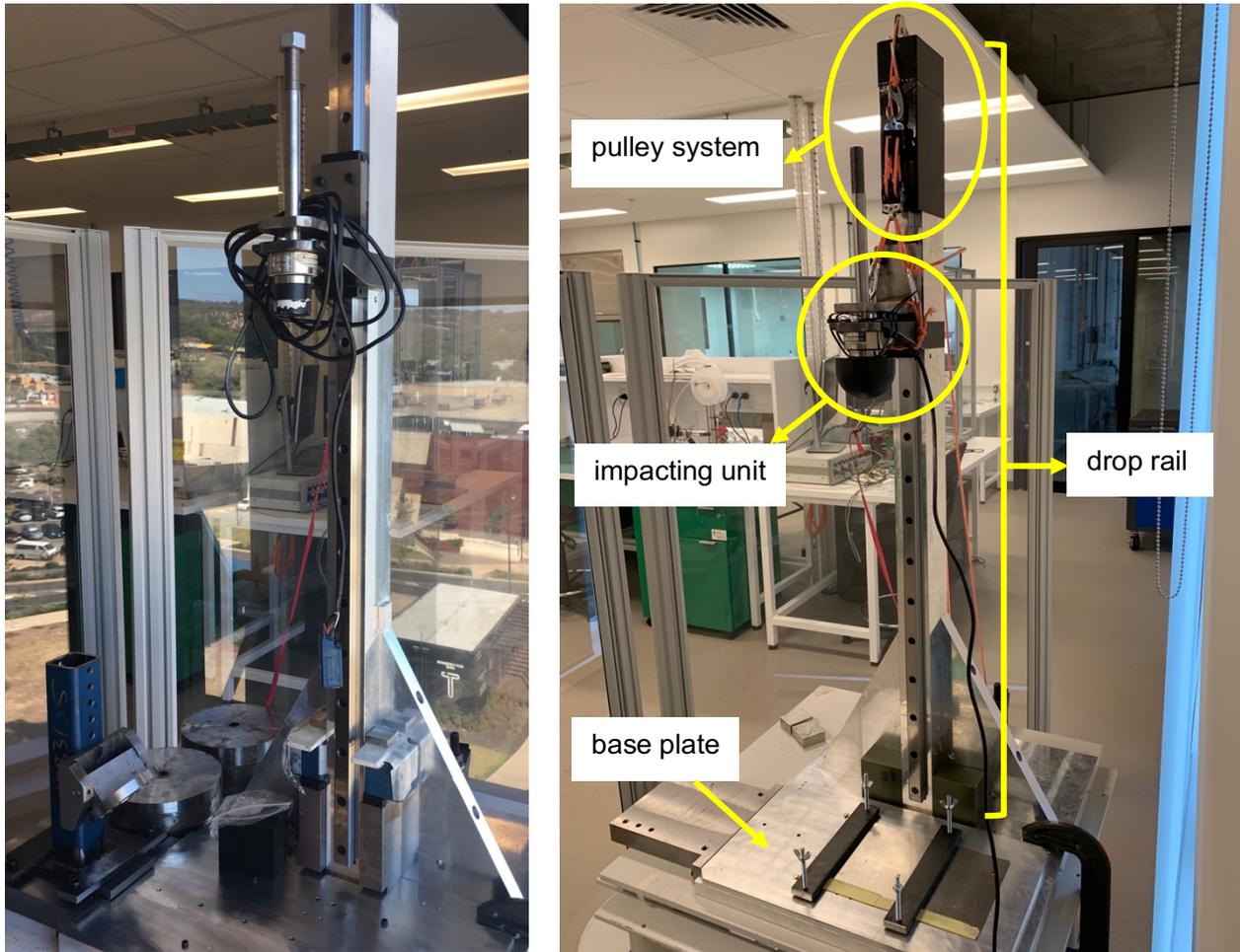
Figure 6: Original (left) and modified (right) drop tower apparatus
