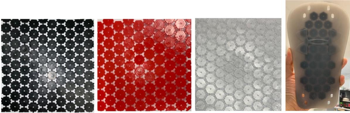
Figure 17: Four Isoblox compositions X, R, T and Z (left to right)
