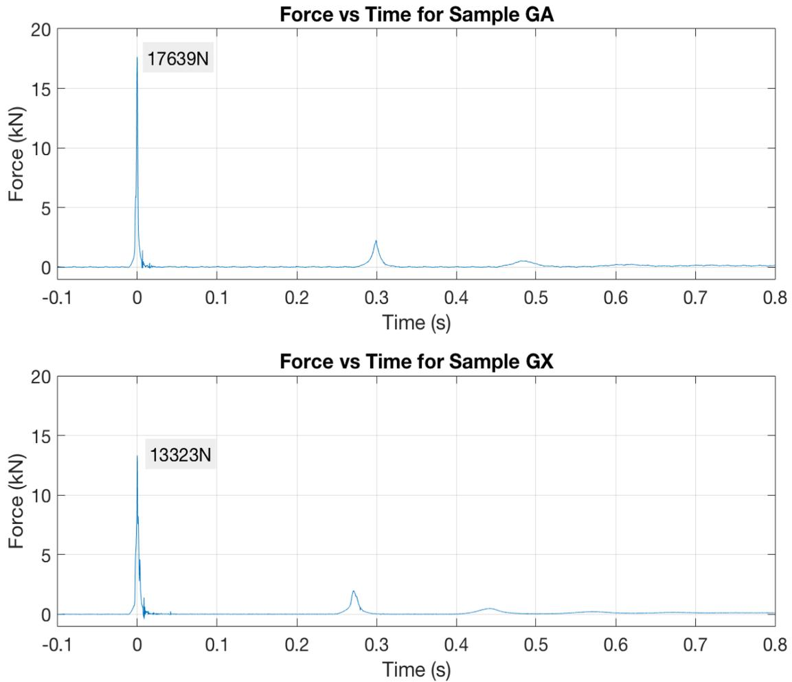
Figure 24: Force vs. time profiles for samples GA and GX, showing high peak forces approaching load cell capacity
