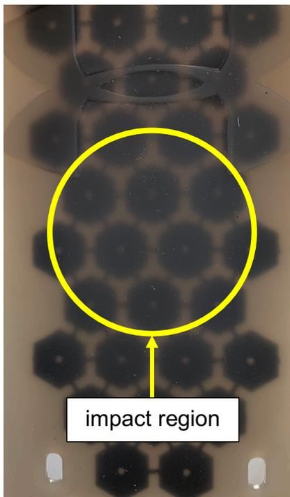
Figure 35: No visible damage to the Isoblox Z layer in samples GAXDZ and GADZ
