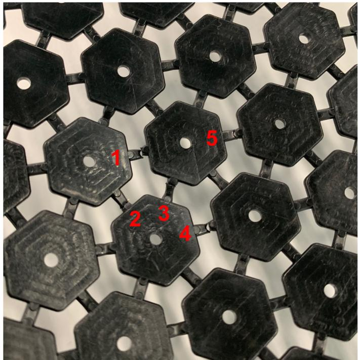
Figure 36: Five hinge fractures in Isoblox X layer after testing on sample GAXDZ
