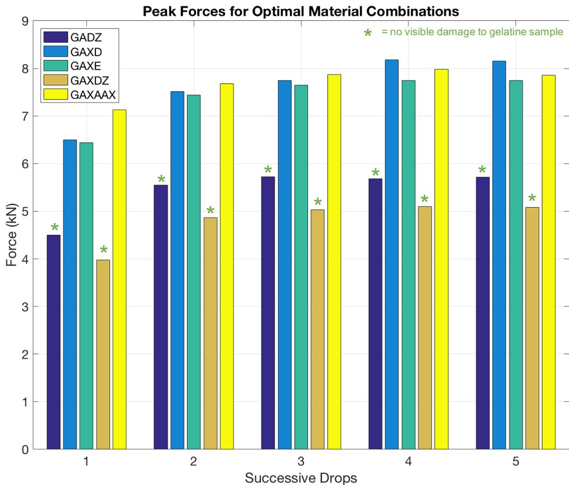
Figure 30: Comparison of new optimised material configurations (GADZ and GAXDZ) with previous samples
