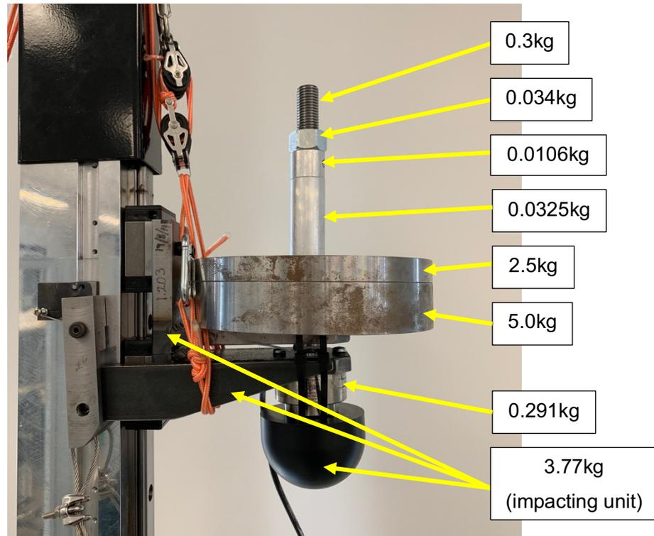
Figure 21: Masses added to impacting unit result in a total drop mass of 11.30kg
