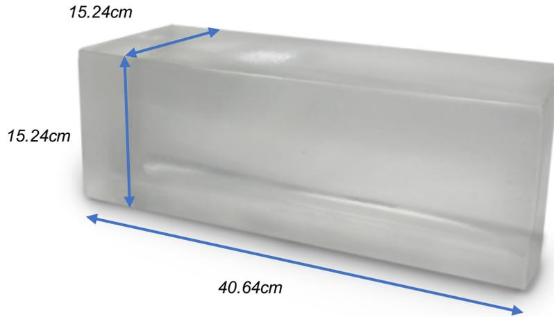
Figure 13: 10% ballistics gelatine block. Adapted from (Clear Ballistics, 2017)
