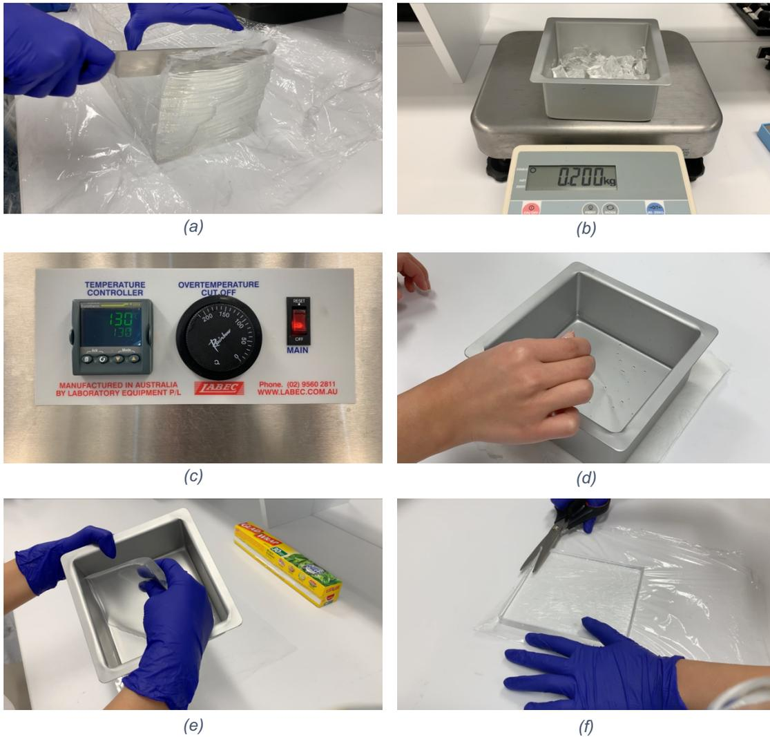
Figure 15: Process of re-melting ballistics gelatine to desired size involving (a) cutting a rough portion from the gelatine block, (b) measuring the desired mass into a mould, (c) melting the gelatine in the oven for one hour at 130°C, (d) release surface bubbles using a pipette, (e) removing the sample from the mould after cooling for one hour, and (f) trimming the edges to remove the meniscus.
