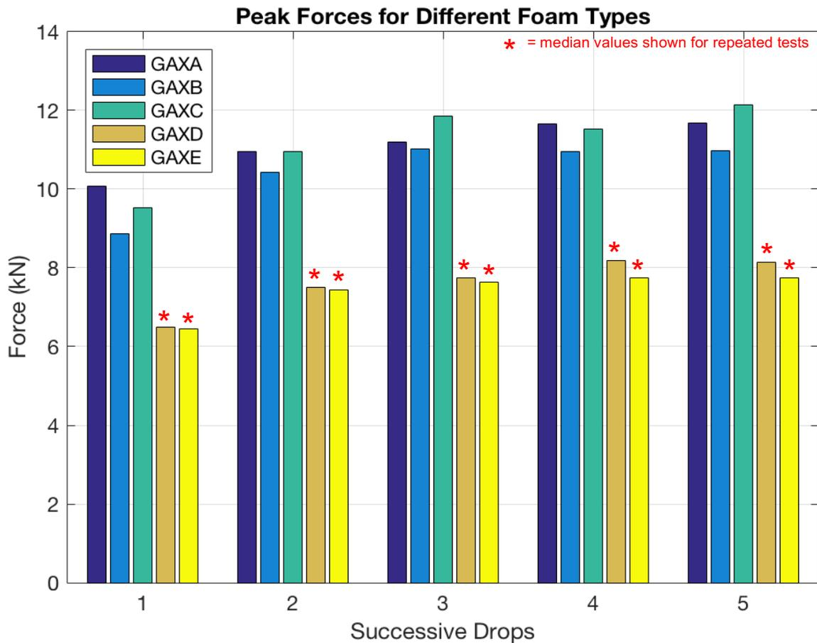
Figure 27: Comparison of peak forces for Foams A-E
