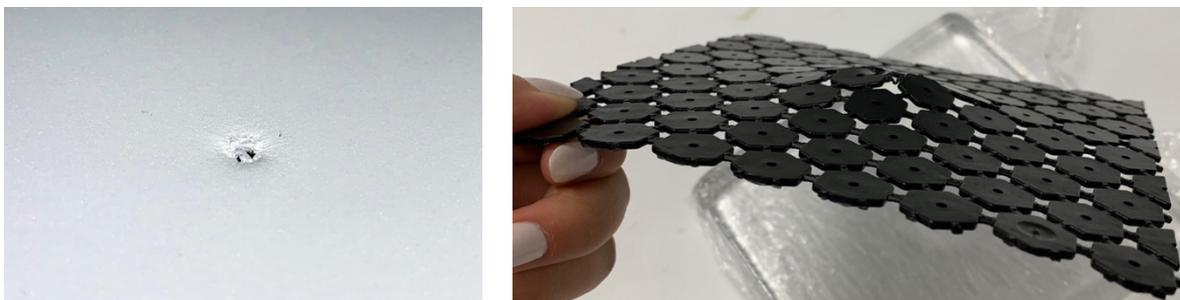
Figure 25: Permanent damage to samples GA (left) and GX (right) after one drop
