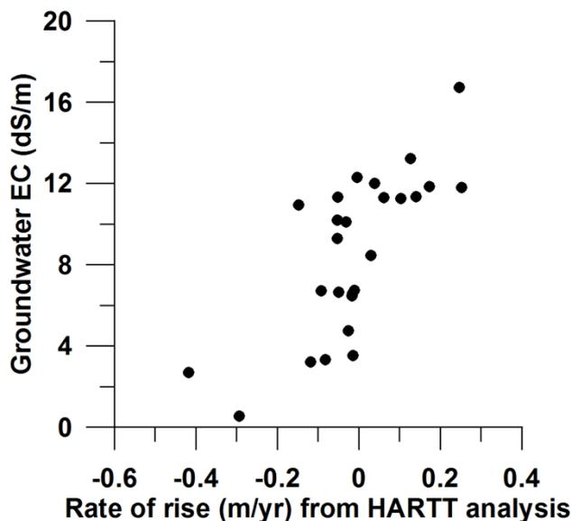
Figure 4.15 Groundwater EC and rate of rise
