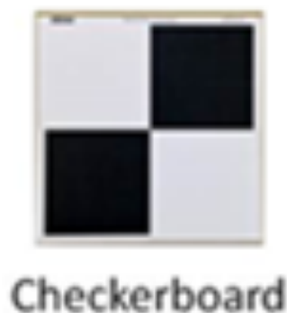
Figure 3.11 The scanner target type used in this research
