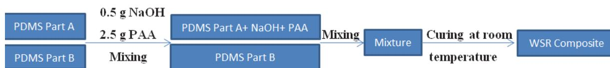
Figure 3.1 Schematic of processing WSR
