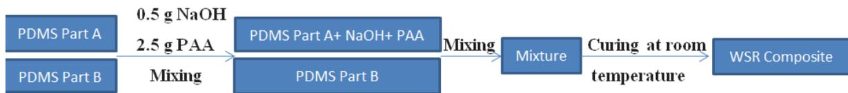
Figure 3.1 Schematic of processing WSR
