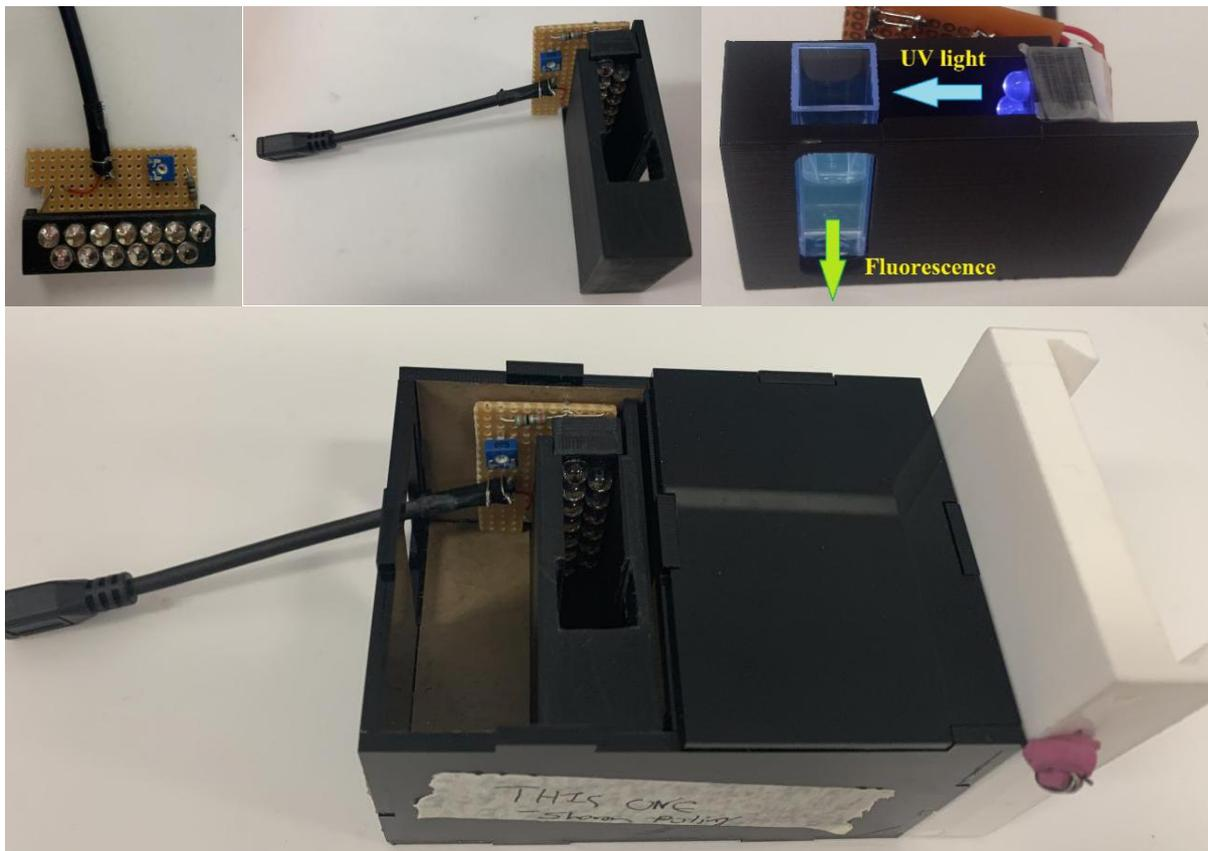
**Figure 65 Physical picture of Urine tester device**
