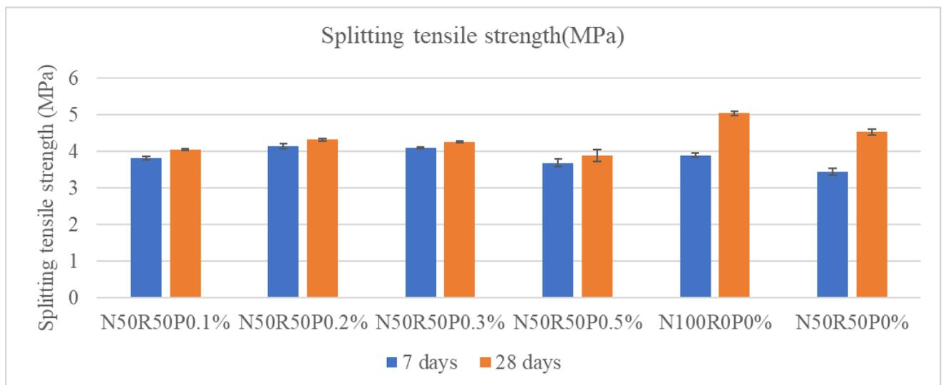
Figure 18. Splitting tensile strength chart for RAC, treated RAC and NAC
