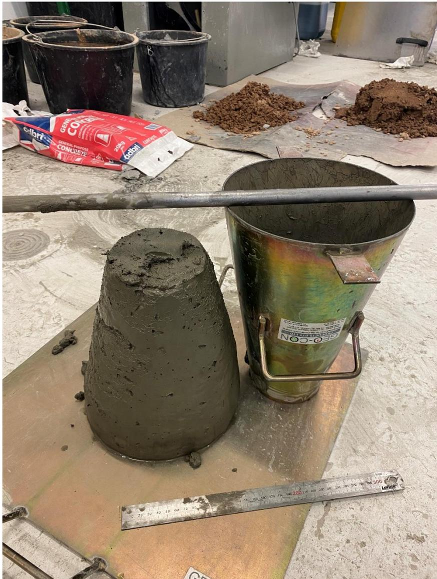
Figure 25.Slump test
