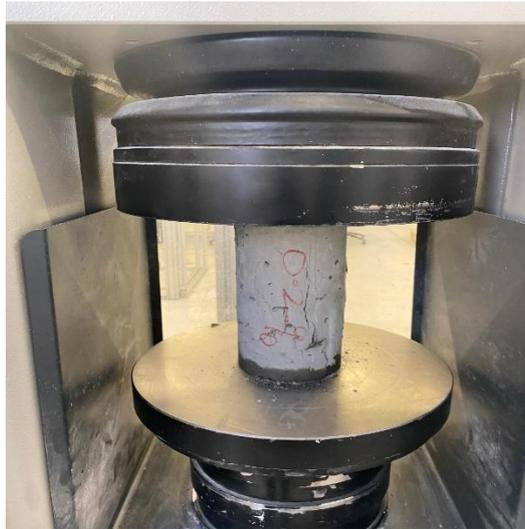
Figure 14. Compressive strength test
