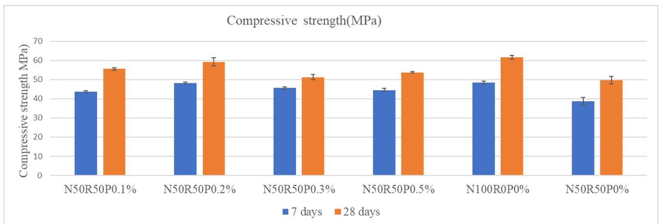
Figure 15. The compressive strength of RAC and NAC at 7 and 28 days
