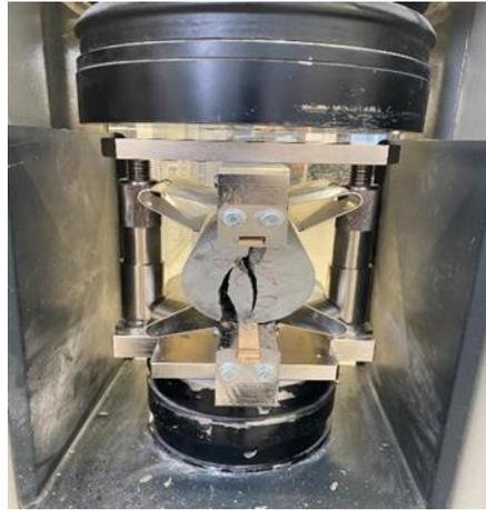
Figure 17. Splitting tensile strength test
