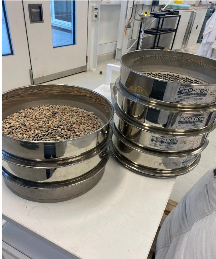
Figure 28. Particle size distribution using the AS method
