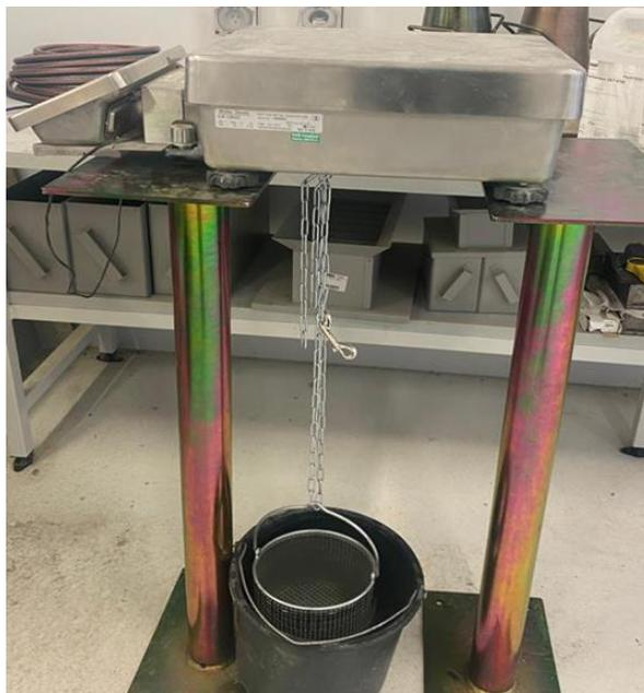
Figure 24. Specific gravity and water absorption test on NCA and RCA
