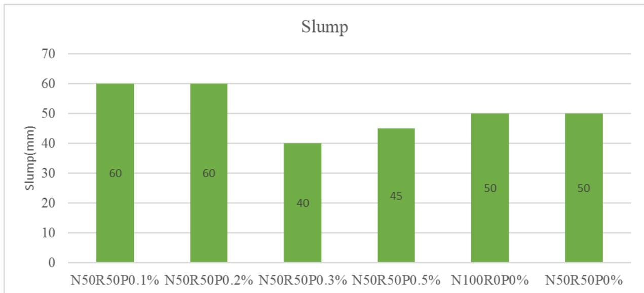
Figure 13. The slump value for the NAC and RAC mixes
