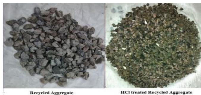
Figure 7. Recycled coarse aggregate before and after treatment with HCL(Abhiram & Saravanakumar 2015)
