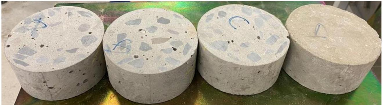
Figure 27.Specimens for water absorption test
