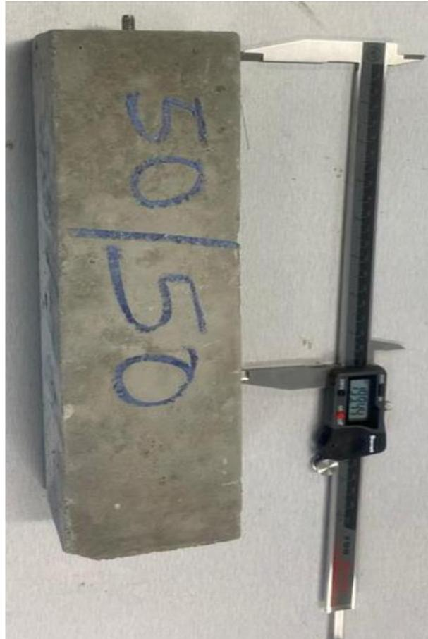
Figure 26.Measurement of drying shrinkage on one of the specimens
