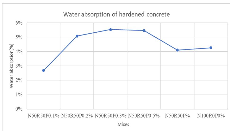
Figure 20. The water absorption of NAC, RAC and treated RAC
