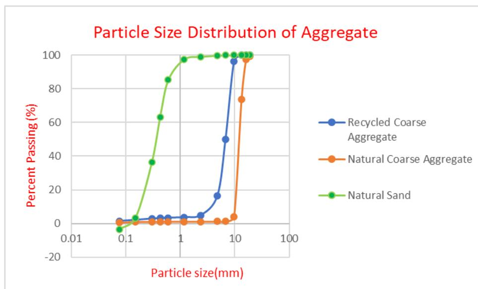
Figure 8. Sieve analysis result for natural sand, RCA and NCA
