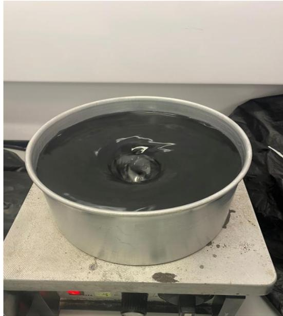
Figure 10. Stirring and mixing of graphene particles with water
