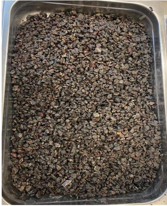
Figure 23. Ready for mix treated RCA
