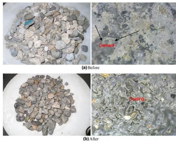
Figure 4. Coating procedure with polycarboxylate dispersant (Ryou & Lee 2014)
