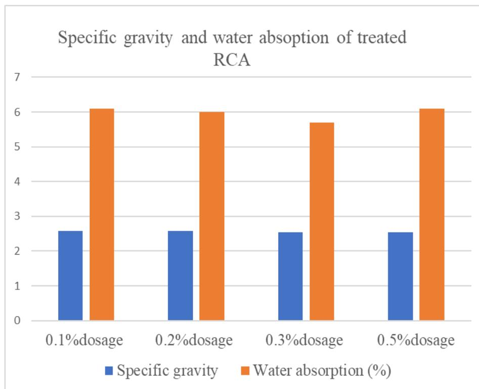
Figure 12. Specific gravity and water absorption rate of treated RCA
