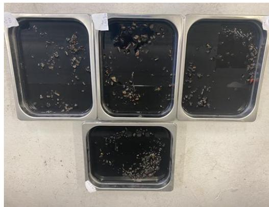
Figure 11. Soaking of RCA into different dosages of graphene
