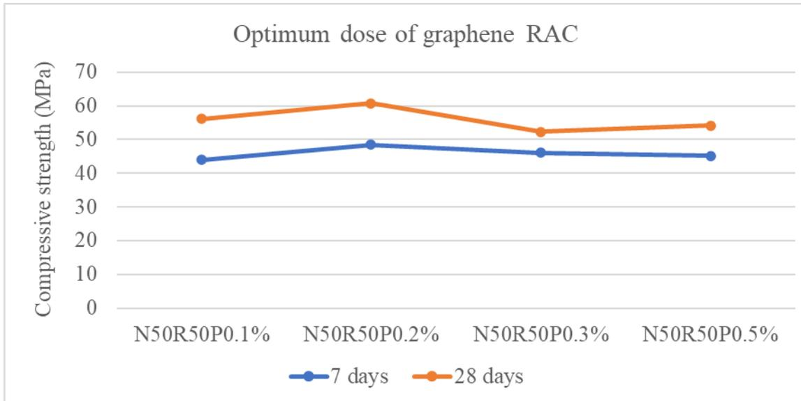
Figure 16. Optimum graphene dose at 7 and 28 days
