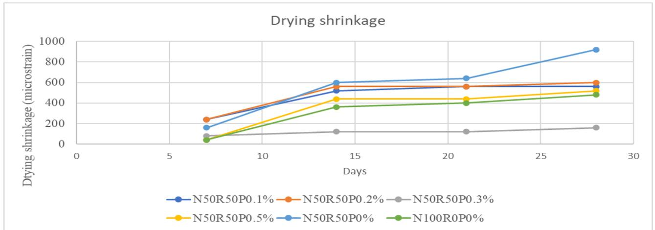
Figure 19. Drying shrinkage of RAC and NAC
