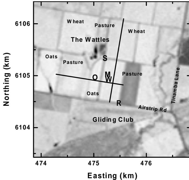
**Figure 2.2** NDVI image of The Wattles property showing the location of the eddy covariance instruments in the wheat ("W") and oat ("O") fields, the location of the meteorological mast in the wheat field ("M"), the scintillometer source ("S") and receiver ("R") and the aircraft north-south and east-west flight tracks (black lines).
