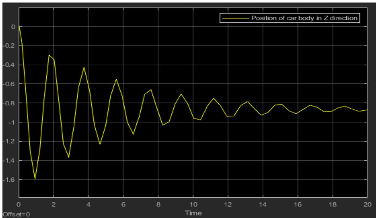
Figure 52 Position of the car body in the Z direction for the inertial body frame
