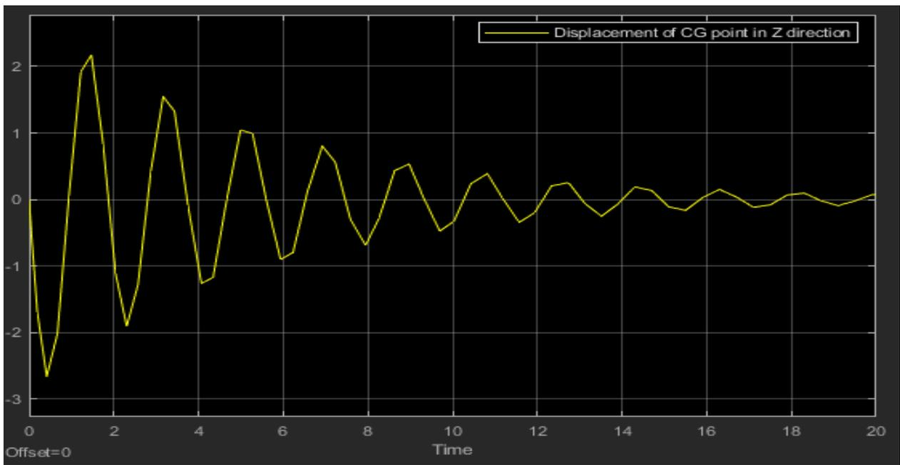
Figure 48 Displacement of CG point in z-direction for the inertial body frame
