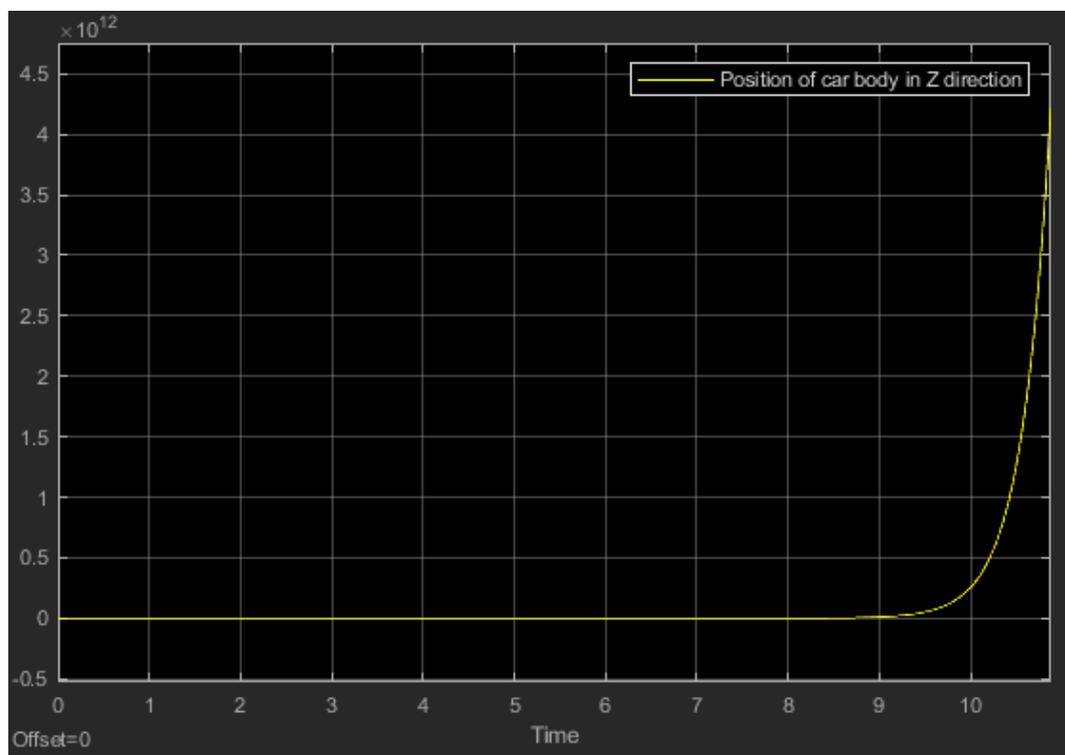
Figure 67 Position of the car body on the z-axis in the inertial frame
