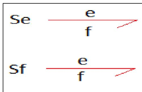
Figure 11- Bond graph symbol of Source elements
