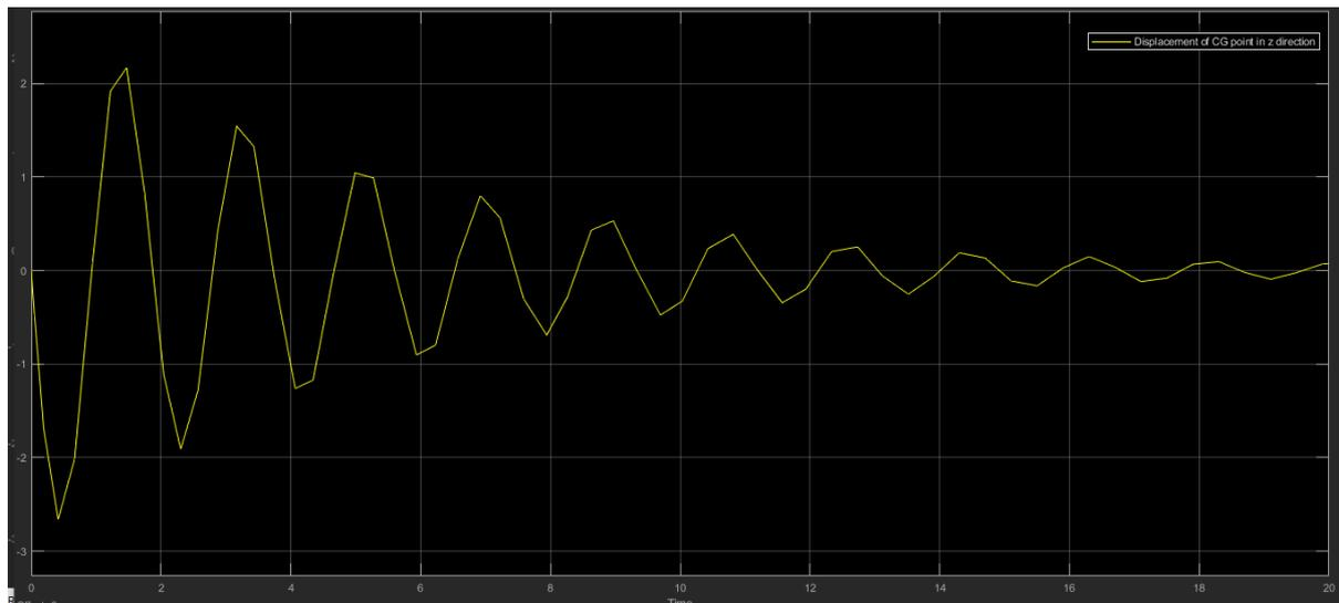
Figure 42 Displacement of CG point in z-direction for the non-inertial body frame
