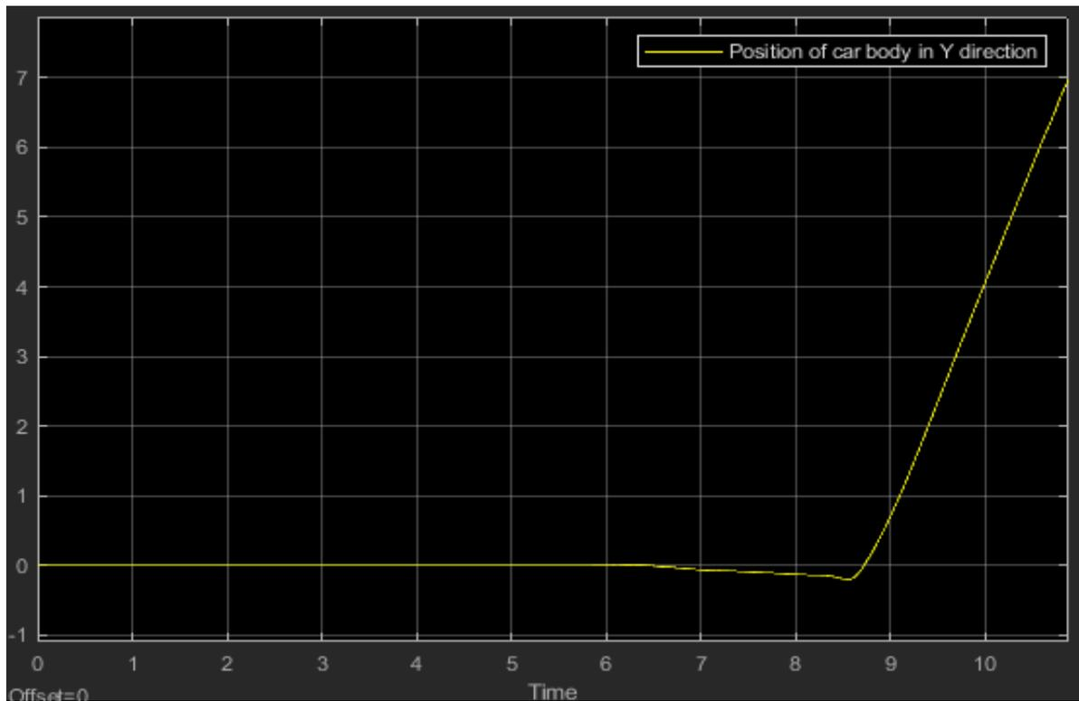
Figure 66 Position of the car body on the y-axis in the inertial frame
