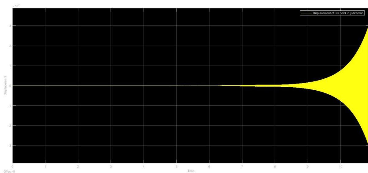
Figure 54 Displacement of CG point in the y-direction for non-inertial frame
