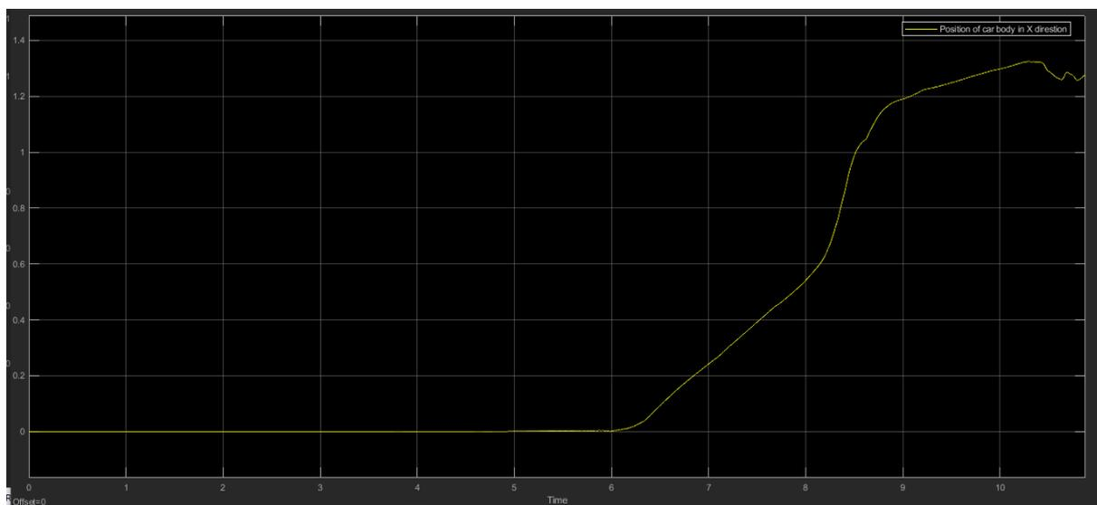
Figure 65 Position of the car body on the x-axis in the inertial frame
