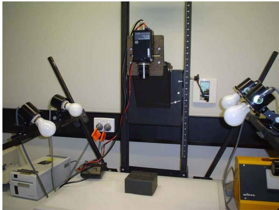
Figure 2.7 Imaging apparatus used to analyse hot dip simulation samples.
