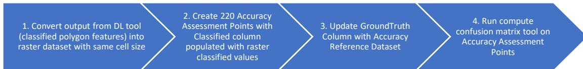
*Figure 25- Manual Accuracy Assessment Tool Check for DL Results*
