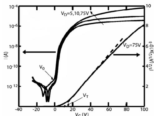
Figure 1.7. Typical transfer curve with the gate voltage  $V_g$  being swept and the drain voltage being swept from -40 to 100V [2]
