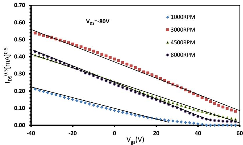
Figure 3.4-  $\sqrt{I_d}$  vs.  $V_{gs}$  curve of solution processed TIPS-DBC OFETs prepared using different spin rates. Data is theoretically fit using equation (1).
