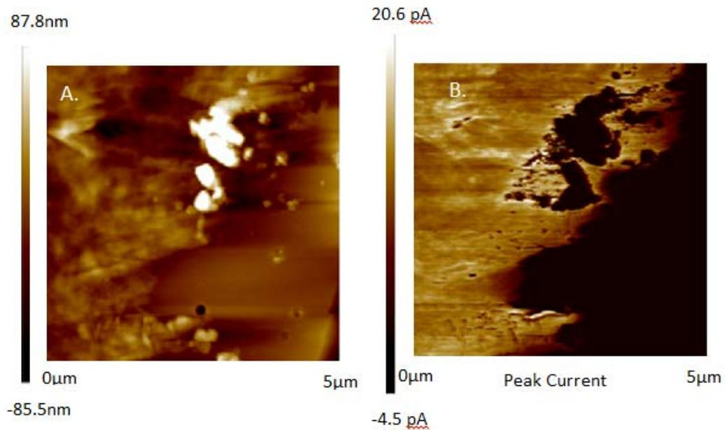
Figure 5.12. Conductive AFM conductive map A.10µm x 10µm peak current image B.5µm x 5µm AFM peak current image.
