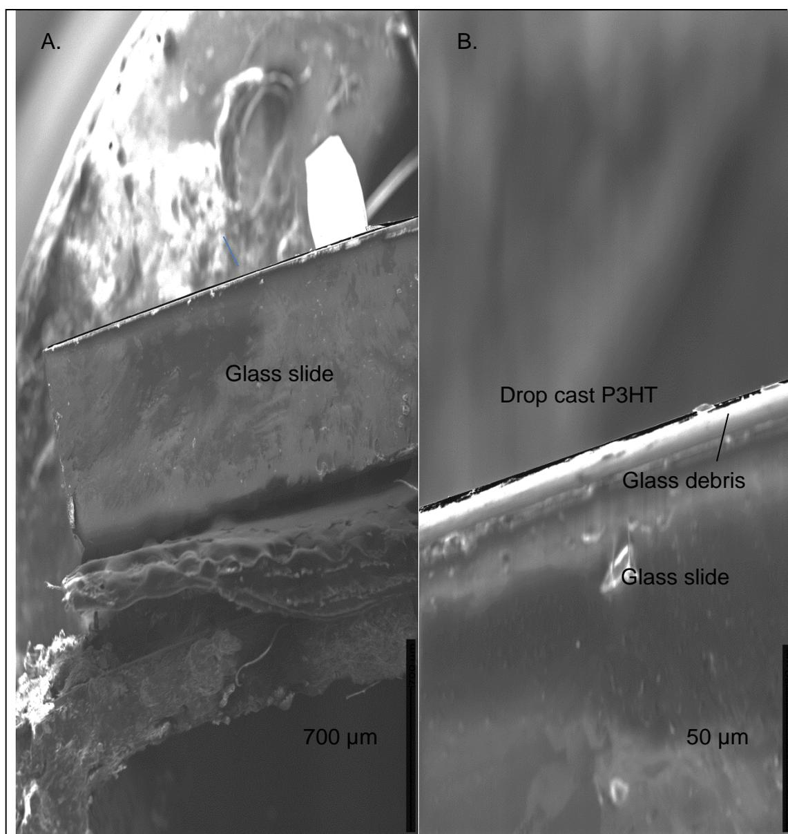
Figure A.3 – Cross section SEM images of drop cast 30mg/mL P3HT films on liquid nitrogen snapped glass slide.
