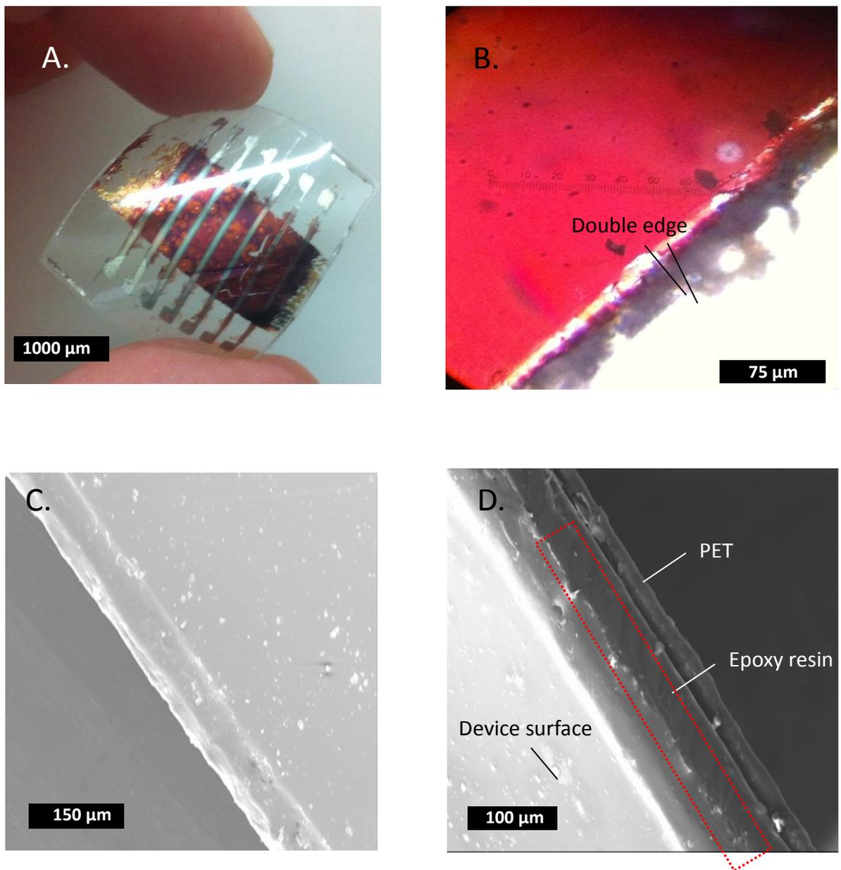
Figure 5.3. Mechanically cut two terminal devices on flexible PET substrates. A. Optical image of a two terminal device substrate on PET. B. Optical microscope image of the cut edge. C. Planar SEM of the cut surface. D. Cross section SEM of mechanical through PET.
