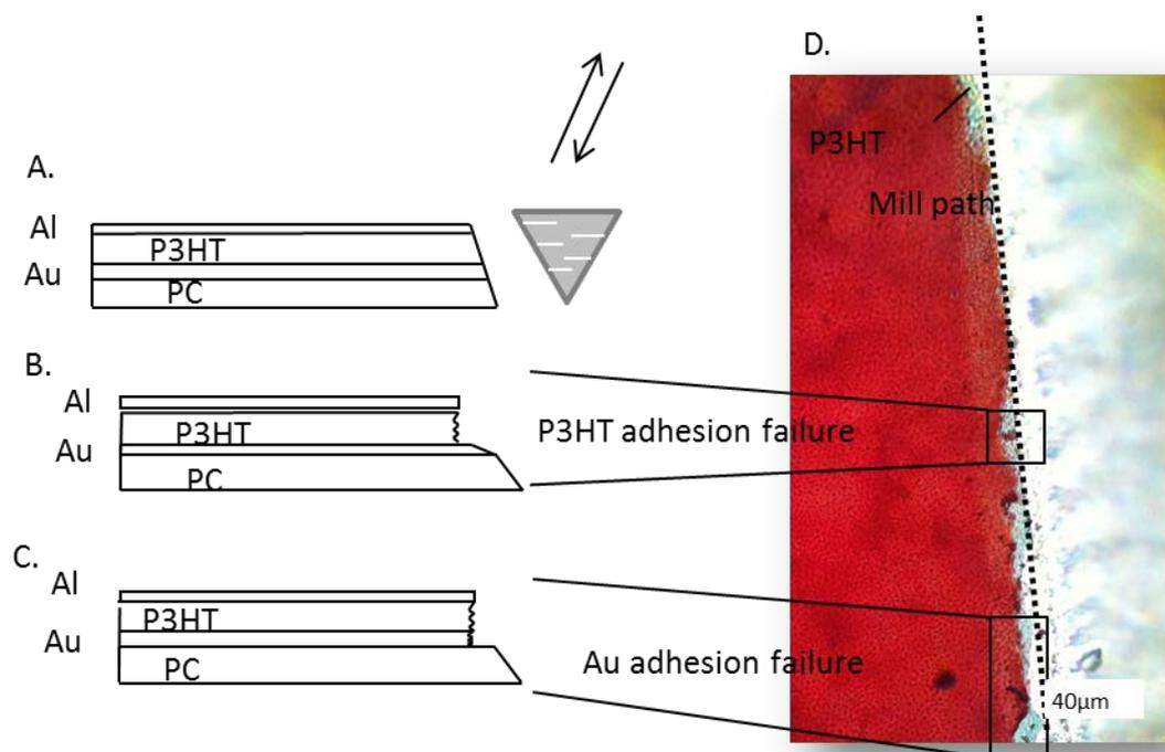
Figure 5.6. Delamination occurring during the CNC machine cutting of substrates. A. Idealised device structure B. Gold adhesion failure removing/stripping P3HT in the process C.P3HT adhesion failure and D. Optical microscope image showing a representative vertical cut with damage. 123
