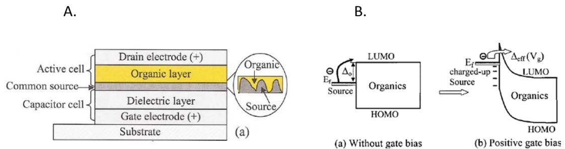
Figure 1.18. A. Fabricated VOFET device by Yang et al. on glass substrate. Copper is used as the gate electrode and in combination with 240nm lithium fluoride dielectric forms a capacitor cell. An aluminium source electrode and n-type  $C_{60}$  is used as the active layer B. Visualisation of the energetic barrier at the metal- semiconductor interface, key operating principle of the stacked architecture operating using an n-type semiconductor.
