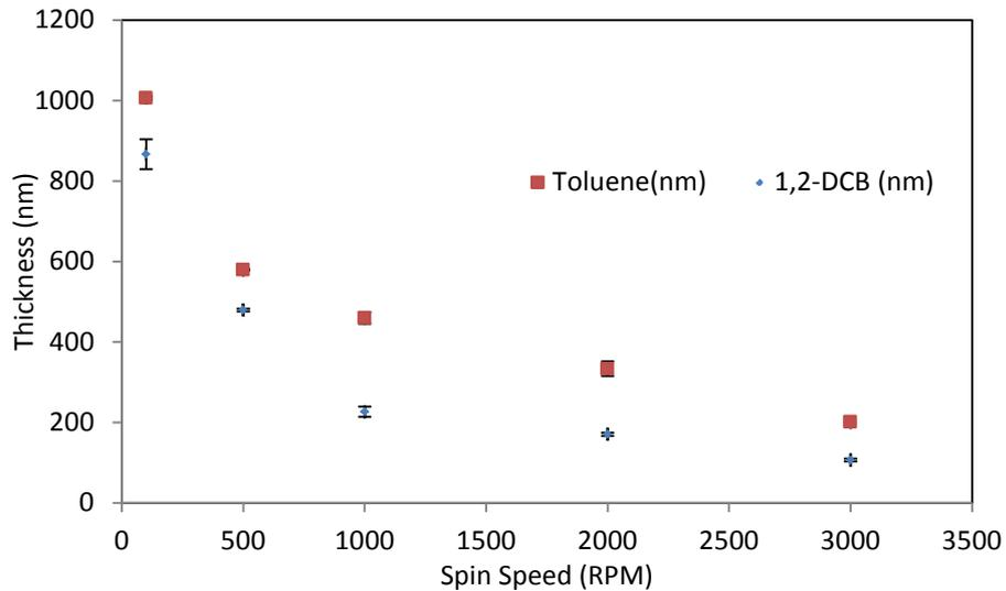
Figure A.2. Plot of measured film thickness (nm) vs. spin speed (RPM) for P3HT thin films prepared using 3% w/v 1,2- dichlorobenzene solvent (red dot) and toluene (blue dot). Error bars are the relative error calculated over three trials.
