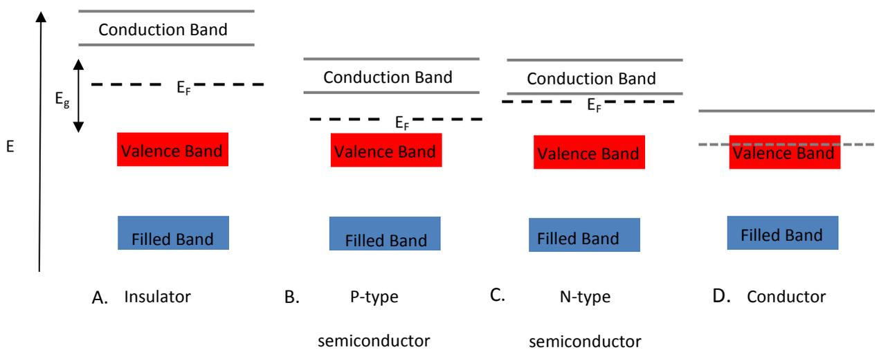
Figure 1.3. Energy band diagram describing the valence band and conduction bands in solid materials. A. Insulator material with a large band gap. B. Semiconductor with a small band gap and the Fermi energy situated mid gap and C. Conductor material with an overlap of valence and electron bands.
