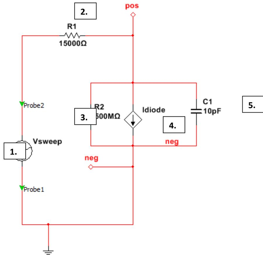
Figure B.2. Multisim 9.0 electronic circuit schematic for Schottky diode with functional elements labelled 1. Piecewise linear voltage, 2. Resistor 3. Resistor 4. ABM current source. 5. Capacitor.
