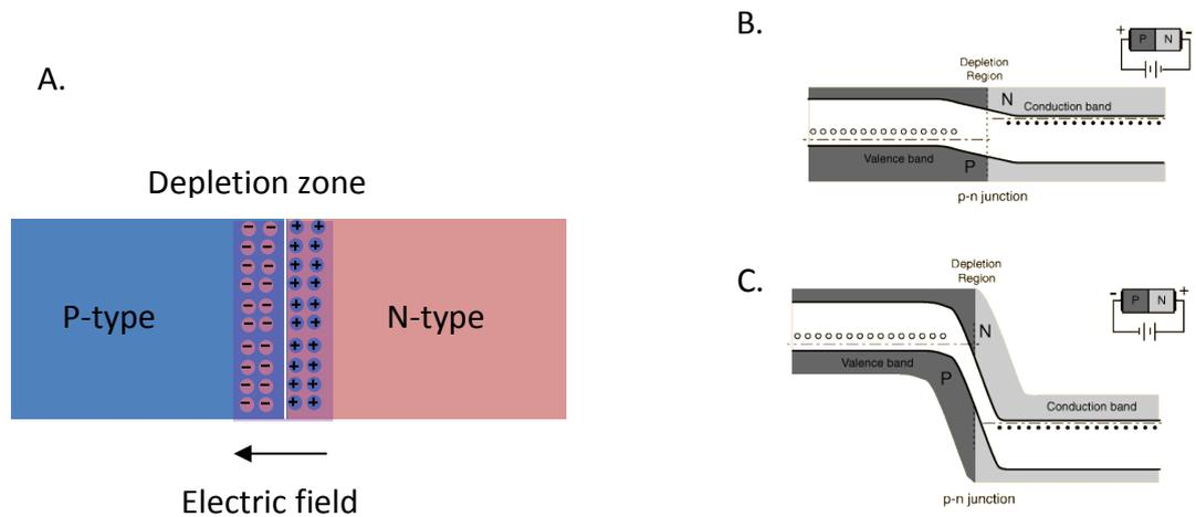
Figure 1.4. A. P-N junction between a p-type and n-type semiconductor material and the resulting rectifying junctions under applied biases. B. Under forward biasing the depletion zone contracts and produces a reduced potential resulting in a lower resistance. C. Under reverse biasing the depletion zone expands increasing the internal potential and increasing the resistance across the junction.
