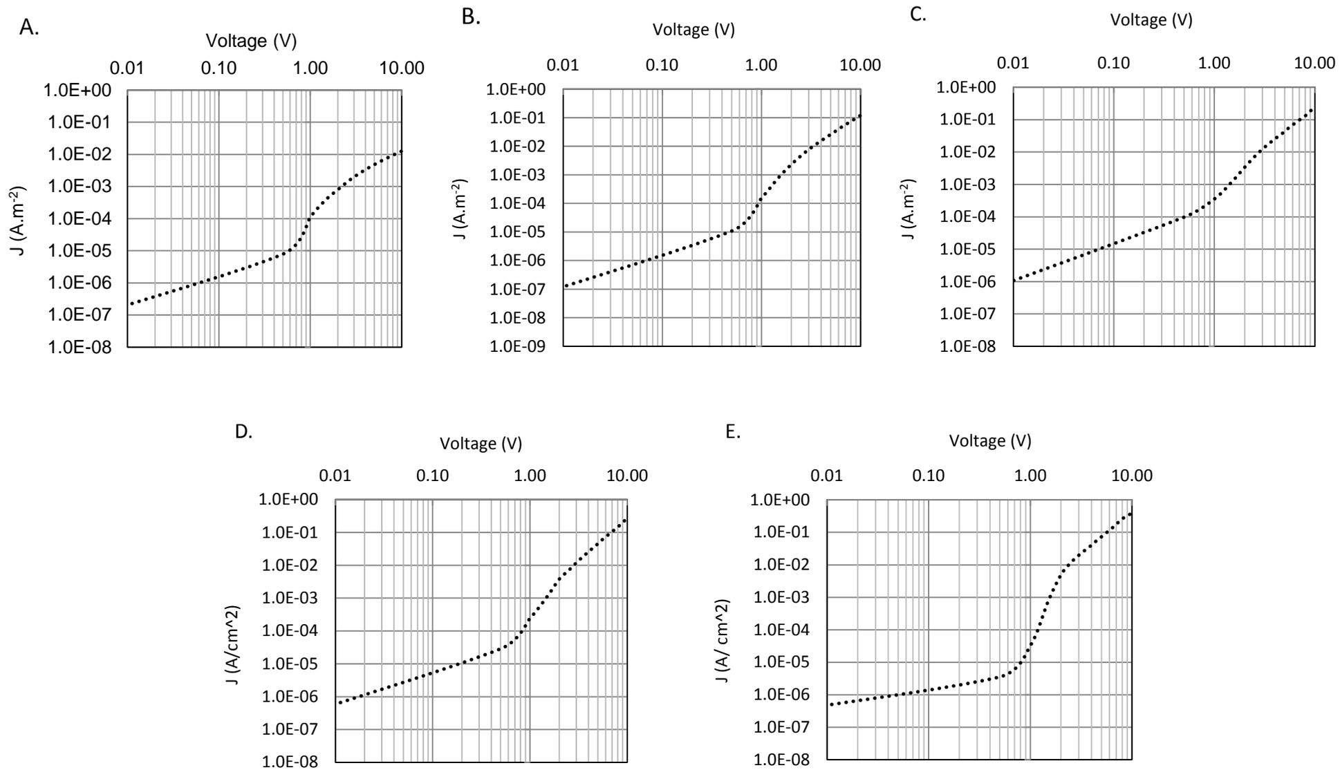
Figure C.5. log J vs. log V plots for Schottky barrier devices with varied active material thickness .A. Drop coat B. 500 RPM C. 1000RPM D. 2000 RPM. E. 3000RPM.
