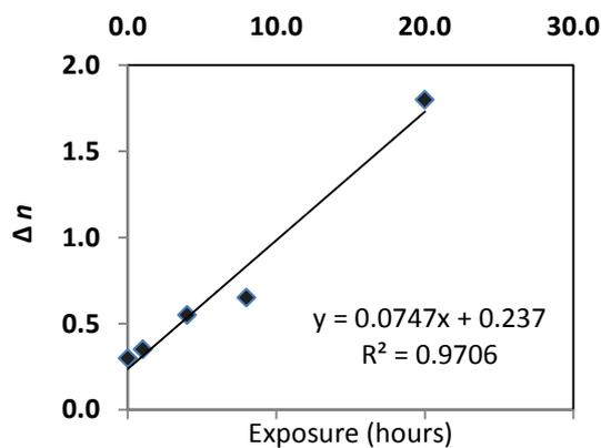
Figure C.3. Shift in the ideality factor with respect to exposure time. A linear fit is applied to the data and a regression  $r^2 = 0.97$  calculated.
