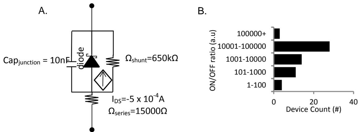
Figure 4.18. Statistical analysis of two terminal Schottky barrier batch processing. A. Statistically averaged device equivalent circuit. B. Bar graph showing the distribution of ON/OFF ratios over 50 devices.
