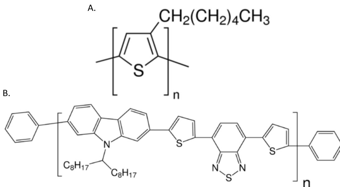
Figure 2.3. Chemical structure of semiconducting polymers. A. P3HT B. PCDTBT.
