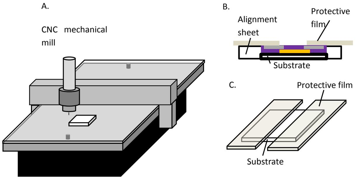
Figure 2.17. Mechanical cutter- LPK 40 A4 circuit board cutter schematic. A. Experimental schematic of the cutting procedure. B. Cross section schematic of the substrate position in the alignment sheet. C. Protective sheet cover protecting the top surface of the device surface with the cut path exposed for cutting.
