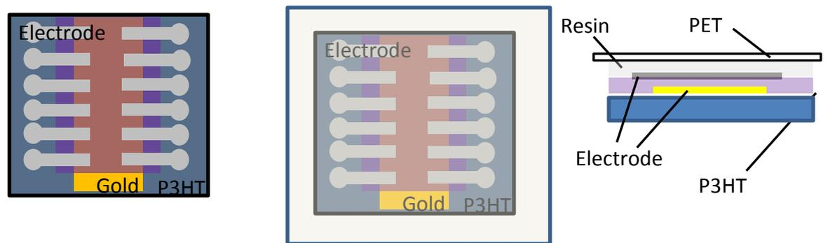
Figure D.1. Lift-off technique for the fabrication of layered structures on flexible PET substrate.
