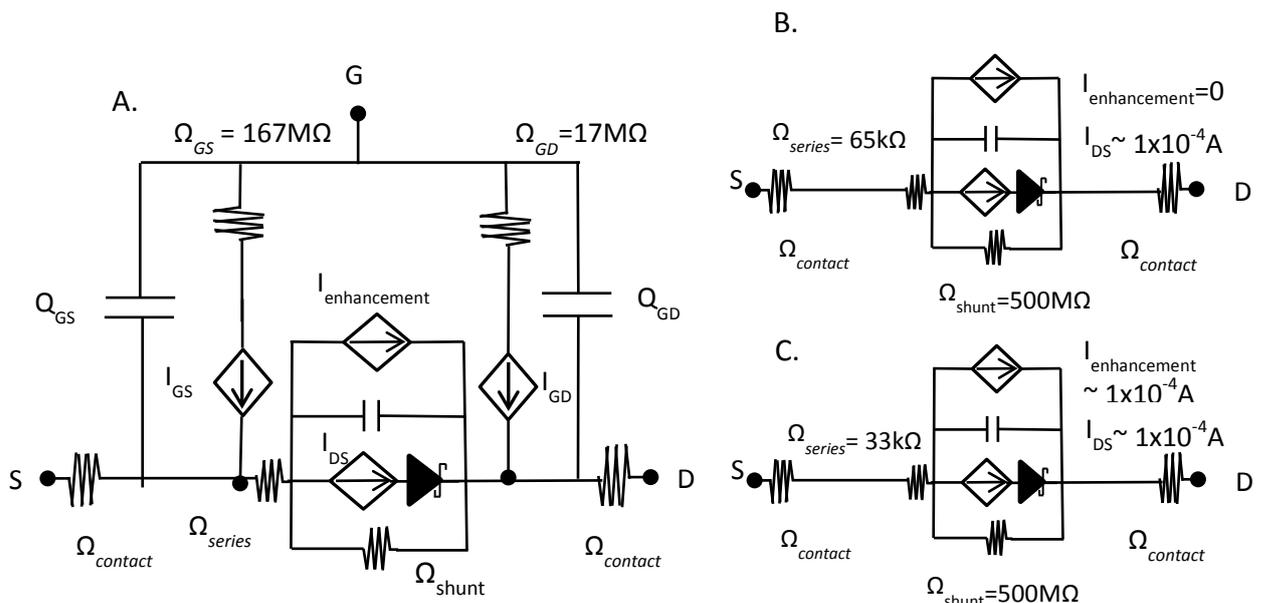
Figure 7.6. A. Proposed equivalent circuit for three terminal Schottky based OFET devices. B. Source-drain equivalent circuit with  $0V_{GS}$  gate bias. C. Source-drain equivalent circuit under an applied  $-30V_{GS}$  gate bias.
