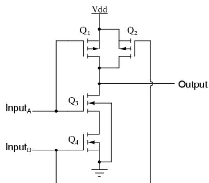
Figure 1.9. CMOS NAND logic circuit. The logic circuit operates utilising an inverter logic circuit with devices  $Q_1$  and  $Q_3$  on input A and devices  $Q_2$  and  $Q_4$  on input B. The resulting output will be high for all cases where either  $Q_1$  and  $Q_2$  saturate and will only go low if both  $Q_3$  and  $Q_4$  saturate.
