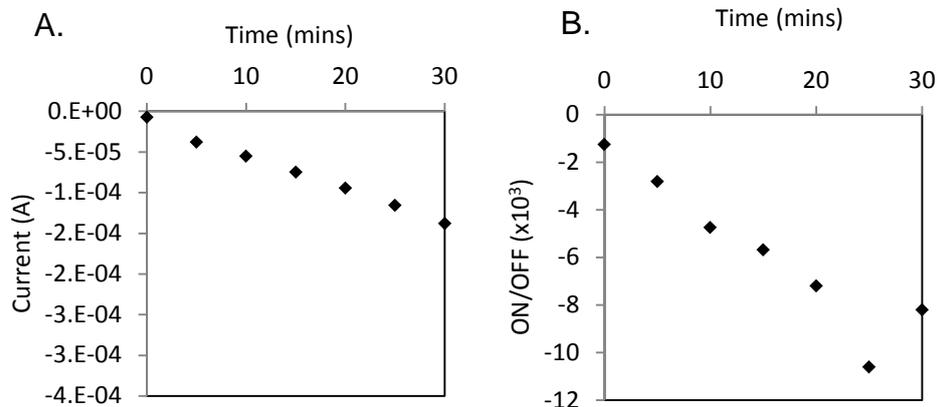
Figure 4.12. Forward current increases in fabricated devices as a function of time over 30mins of testing. A. Forward current performance. B. Rectification ratio over 30mins testing.
