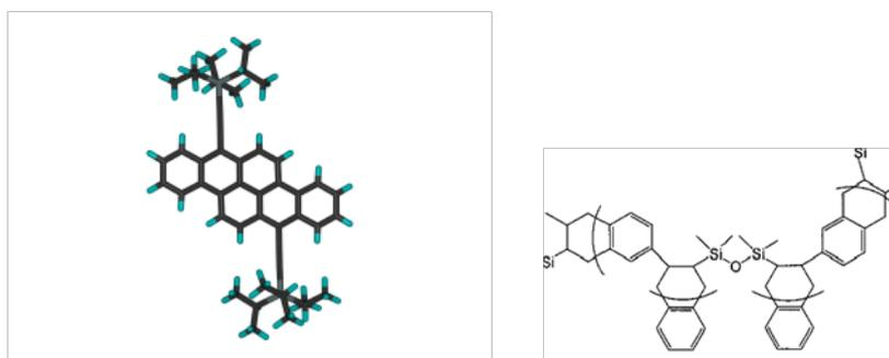
Figure 2.7. Chemical structure of materials in planar OFET structures. A. TIPS-DBC B. BCB
