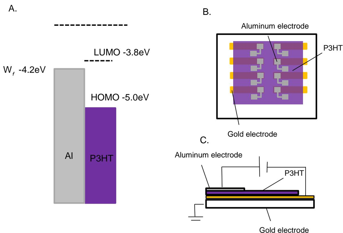
Figure 4.9. Fabricated P3HT-aluminium Schottky diodes. A. Energy level diagram at the P3HT-Al interface. B. Top view substrate schematic for two terminal Schottky barrier substrates C. Side view electrical characterisation cross section schematic indicating applied biases under testing for two terminal devices on polycarbonate. [27]
