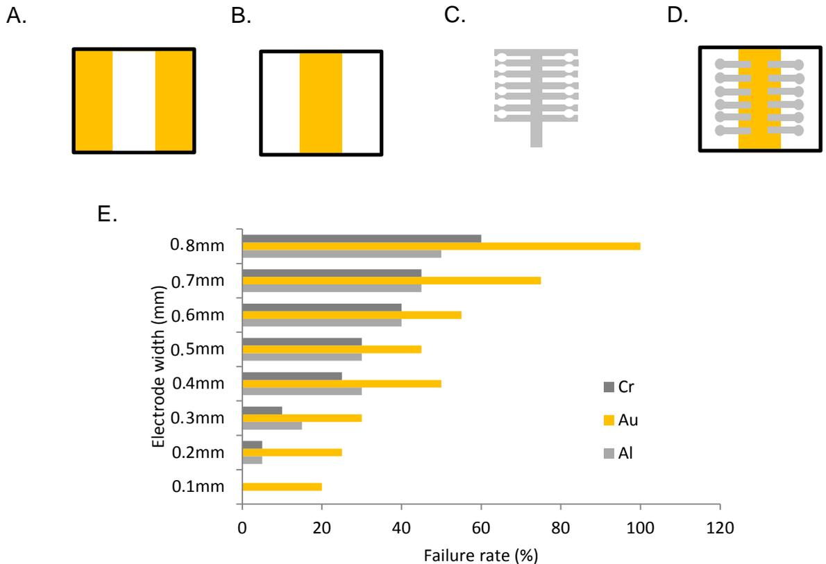
Figure 4.7. Electrode patterning for a manually aligned shadow mask featuring a rib cage design allowing for variable cross-sectional area. A. Uniform communal electrode shadow mask. B. Resulting patterned electrode. C. Top ribcage shadow mask with contact patch and variable electrode width. D. Resulting patterned top electrode. E. Failure rate for devices with various sputtered metal electrodes gold, aluminium and chromium with varied electrode width.
