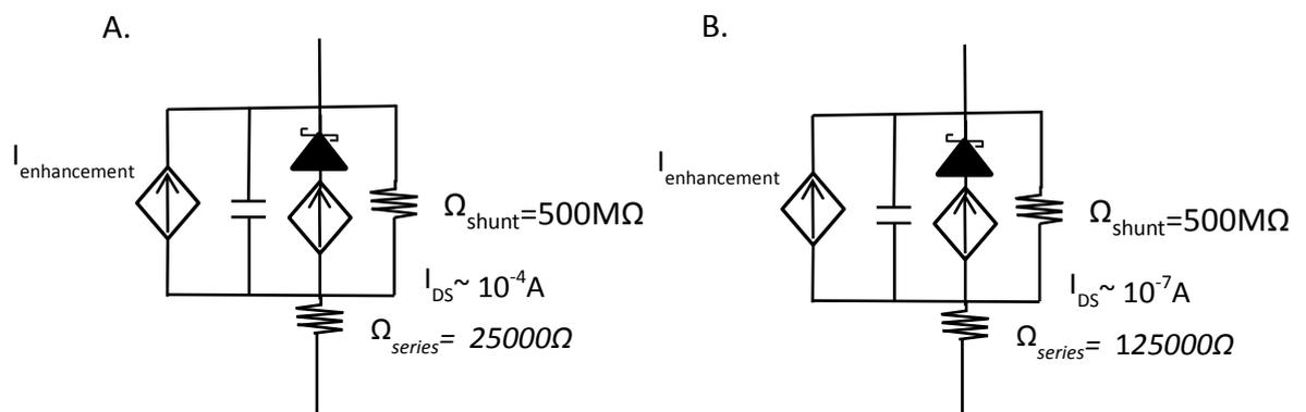
Figure 7.10. Proposed equivalent circuit describing the parallel currents contributing to the drain current. B. Source-drain equivalent circuit for a thin film schottky showing series resistance and OFF state currents. C. Source-drain equivalent circuit with labelled series resistance and OFF state current for drop cast three terminal devices. The current magnitude at  $-4V_{DS}$  is used to represent
