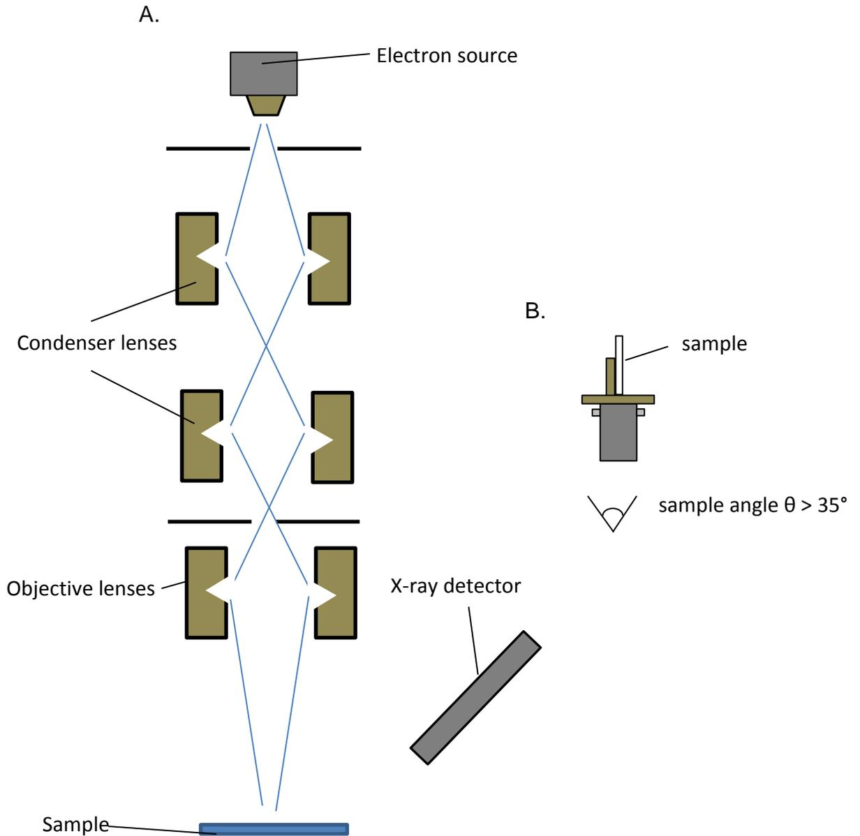
Figure 2.10. A. Schematic representation of the scanning electron microscope. An electron beam is focussed on a sample and the secondary electrons ejected from the surface and detected at a detector creating an image of the surface. B. Perpendicular sample mount stage allowing for the imaging of device cross sections.
