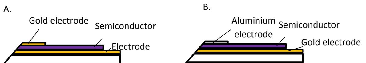
Figure 6.2. Cross section schematic of two terminal devices with different electrode configurations. A. Asymmetric electrode configuration with gold source electrode and aluminium drain electrode. B. Symmetric electrode configuration with gold source and drain electrode.
