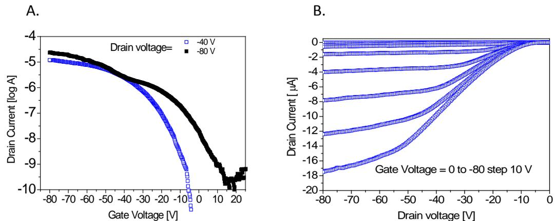
Figure 3.7. I-V characteristics of an TIPS-DBC device evaporated at 50°C. A. Transfer curve with gate voltage sweeping from -80 V to 25V. B. Output curve with gate voltage ramped to -80 V. Measurements were taken under room temperature in a nitrogen environment.
