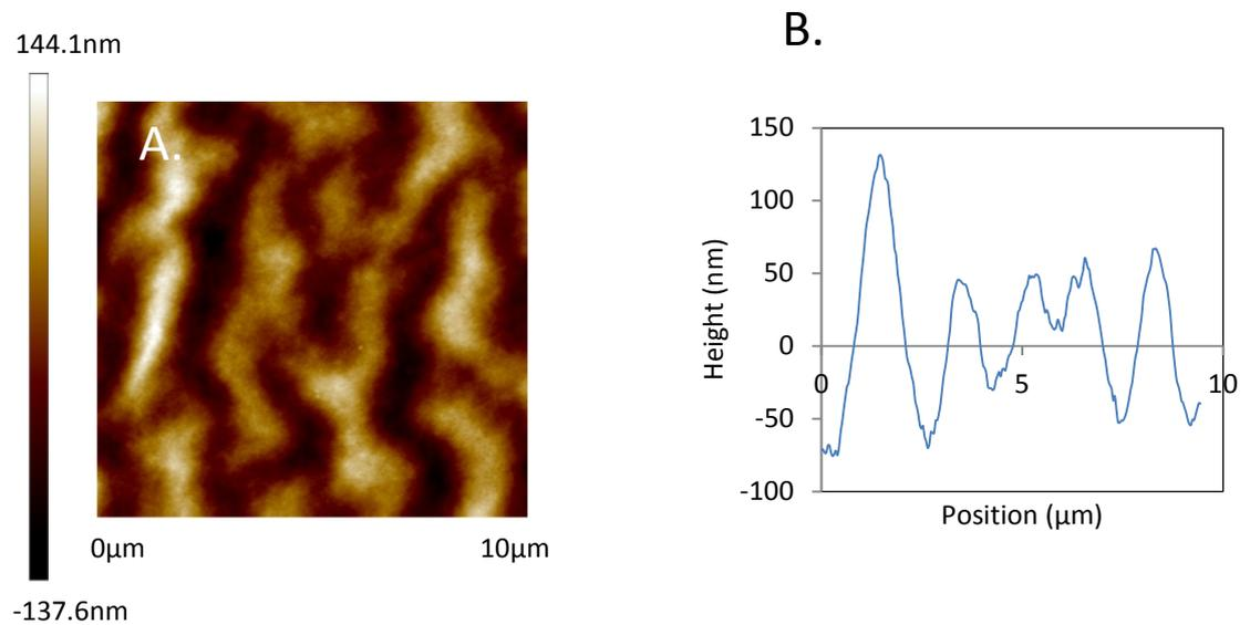
Figure 5.2. Film deformation from hot scalpel scoring of device substrates A. 10µm x10µm topographic height image of the polymeric deformation across the cut surface. B. Cross-section analysis of the topographic image.
