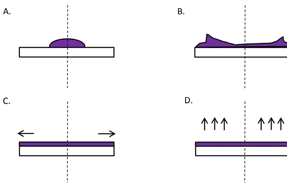
Figure 2.4. Schematic depiction of spin coating procedure. A. Deposition of solution on substrate. B. Rotation and spreading of the solution. C. Steady rotation and the removal of solution via viscous forces. D. Constant rotation where film thickness is reduced by solvent evaporation.
