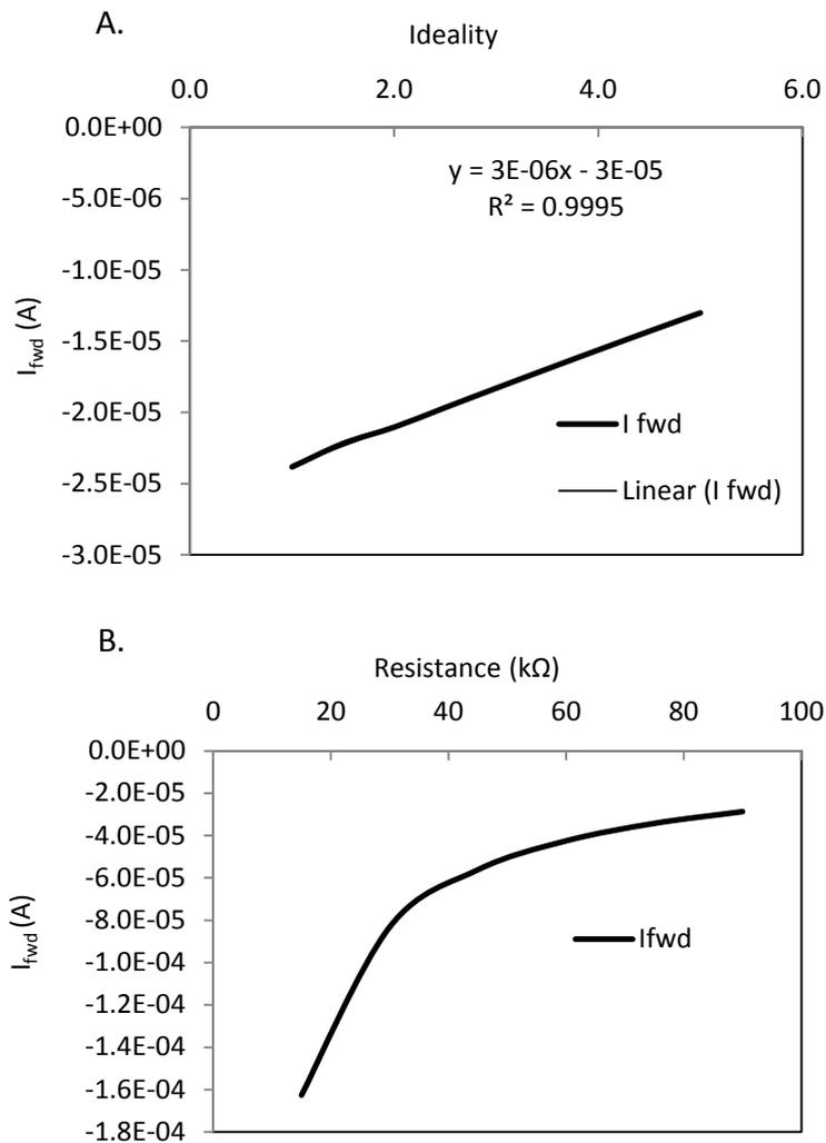
Figure B.4. Plotted forward current relationship A.  $I_{fwd}$  vs. ideality  $n$  and B.  $I_{fwd}$  vs.  $\Omega_{series}$ . A linear regression fit is used in A.
