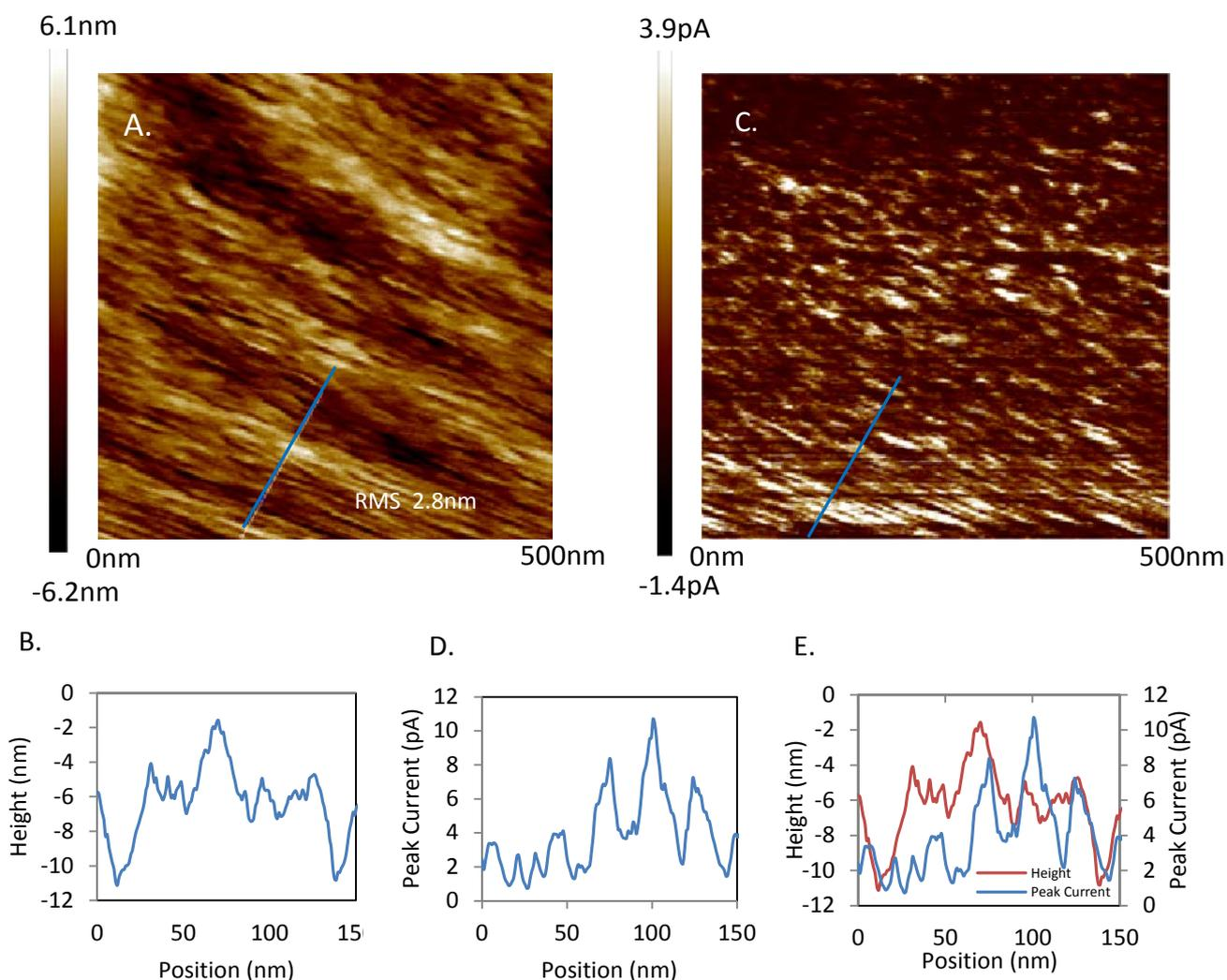
Figure 4.4. Conductive mapping of P3HT thin films A. 500nm x 500nm tapping mode height image of 150C annealed sample with area analysed by cross section (blue line). B. Cross section analysis showing height at the location labelled in A. C. Peak current conductive map over the imaged area with area analysed by cross section (blue line). D. Cross section analysis of the peak current magnitudes with respect to location. E. Superimposed topographic height and peak current cross section traces.
