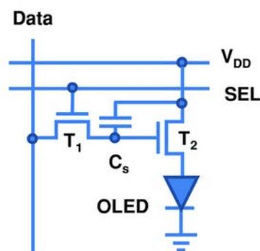
Figure 1.10. Two transistor- one capacitor pixel circuit operating via p-type transistor devices. [3]
