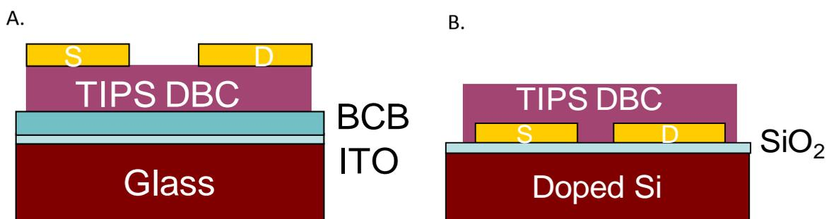
Figure 3.1. FET schematics for fabricated devices. A. top contact FET configuration and B. bottom contact FET configuration.
