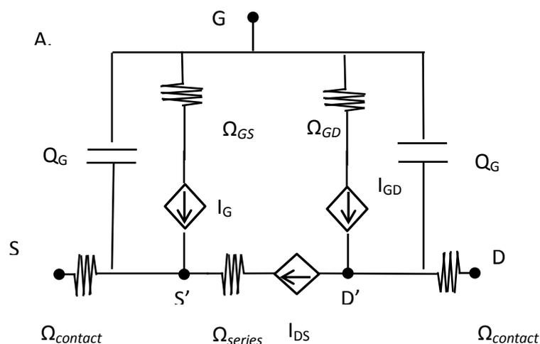
Figure 3.3. OFET equivalent circuit. A. Equivalent circuit describing the electrical performance of an OFET.
