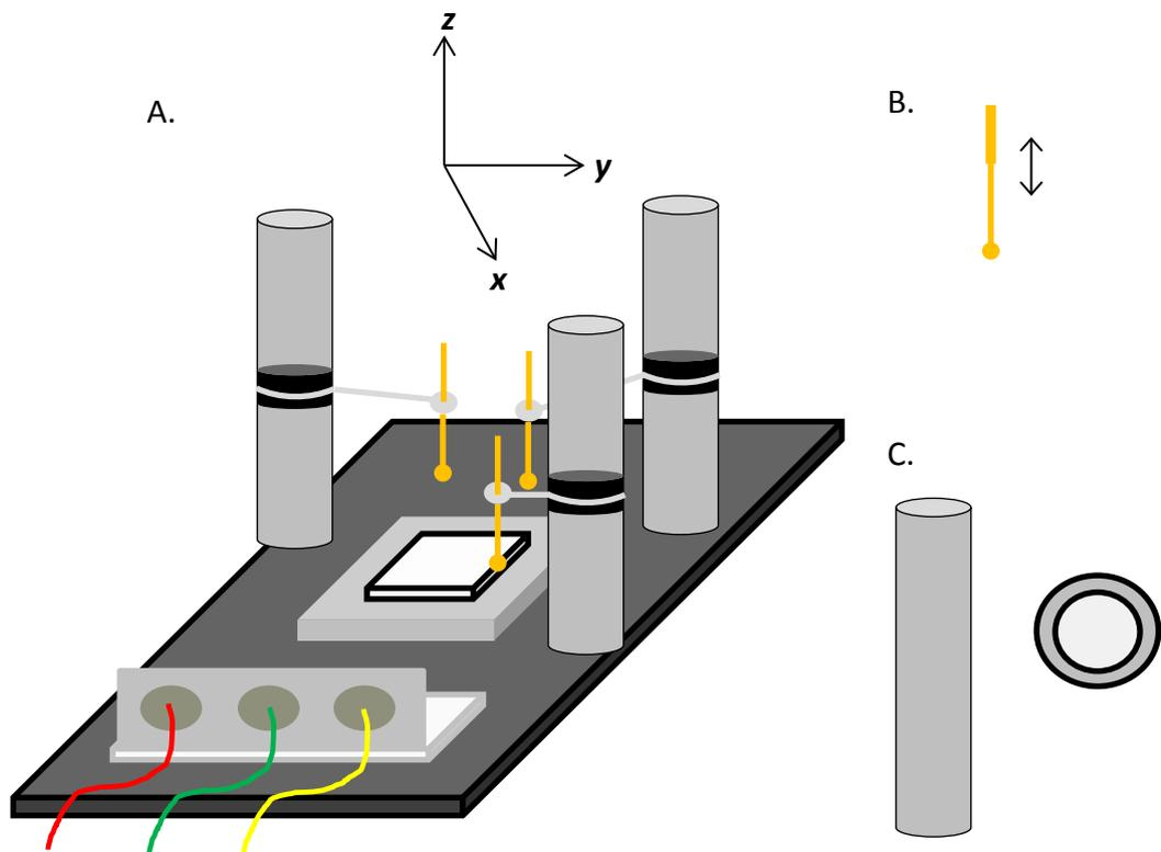
Figure 2.15. Electrical probe station. A. Probe station schematic B. Gold probe contact C. Manual positioning tower schematic featuring a magnetic base.
