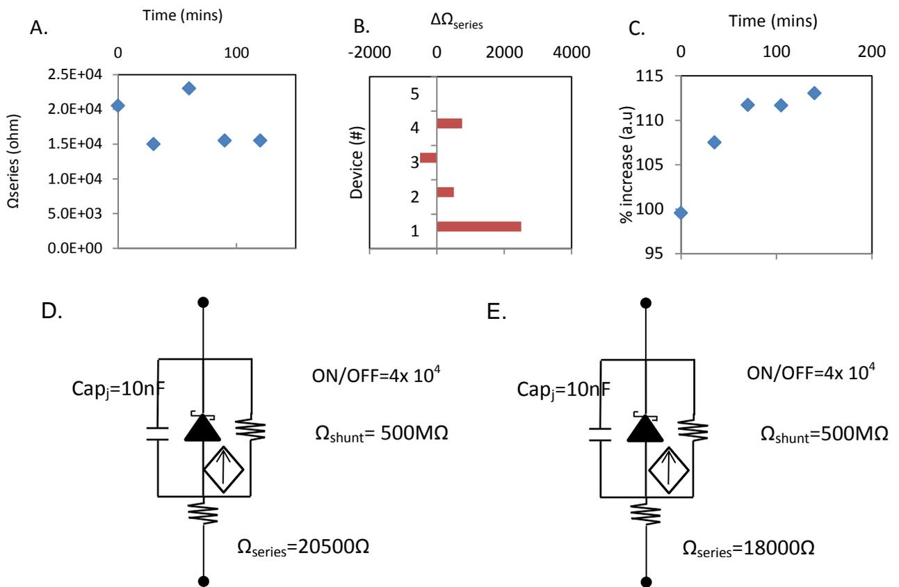
Figure 4.16. Device substrates stored in vacuum for 20 hours A. Simulated series resistance of devices with respect to time after electrode deposition. B. Changes in series resistance over 30mins of consecutive testing. C. Percentile increase in forward current with respect to time after electrode deposition. D. Simulated equivalent circuit for a device immediately removed from vacuum E. Simulated equivalent circuit after 30mins of consecutive testing.
