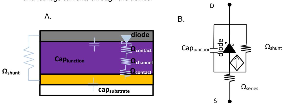
Figure 4.10. Schottky diode equivalent circuit A. Side view schematic of a two terminal device indicating elements of equivalent circuit. The contributions to the series resistance,  $\Omega_{contact}$  and  $\Omega_{channel}$ , the junction capacitance  $cap_{junction}$ , the shunt resistance  $\Omega_{shunt}$  and the Schottky barrier. B. Proposed equivalent circuit based on the Shockley equation.
