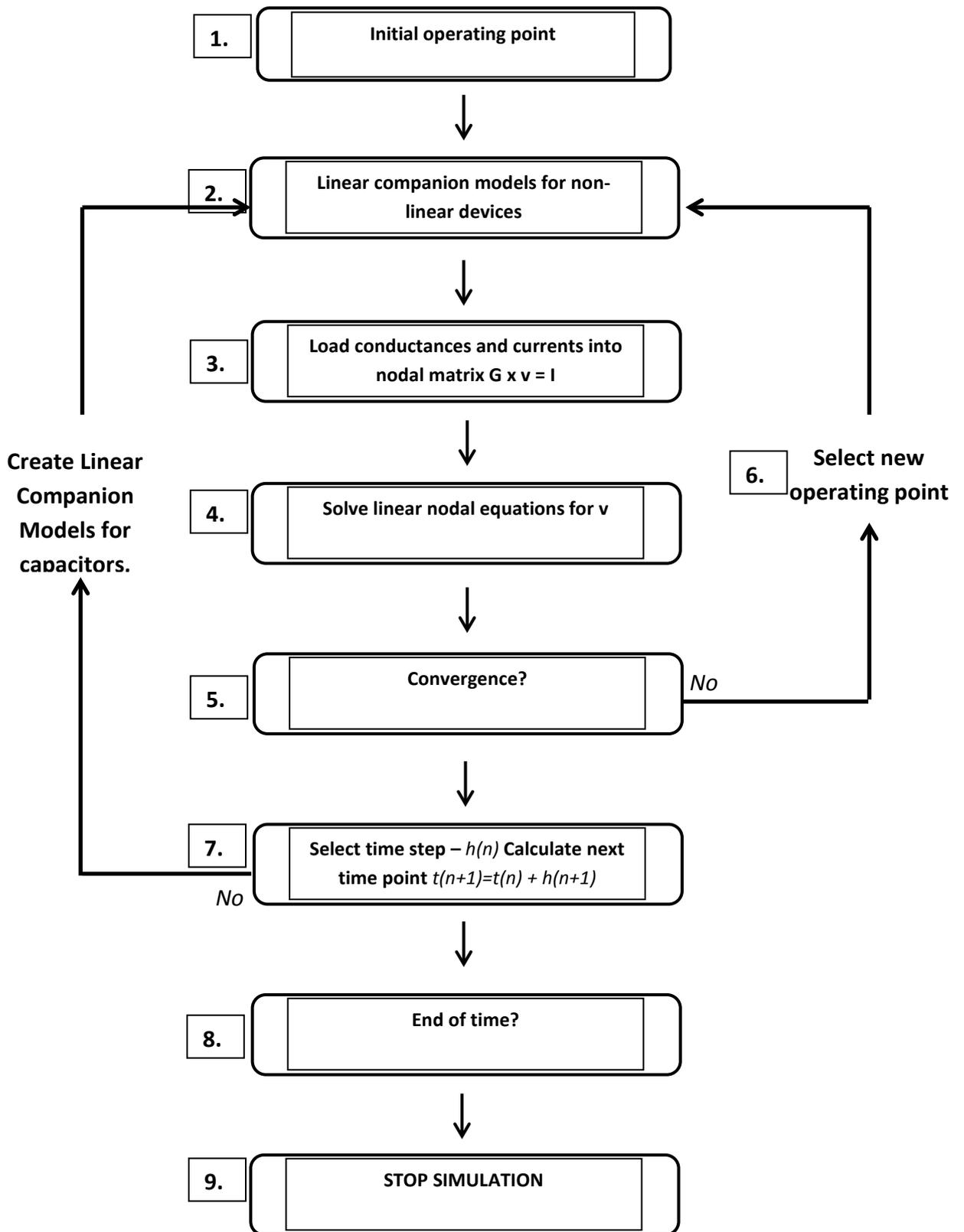
Figure B.1. SPICE computational flow chart describing the nodal analysis undertaken in a transient analysis and the iteration steps for determining a complete time analysis.
