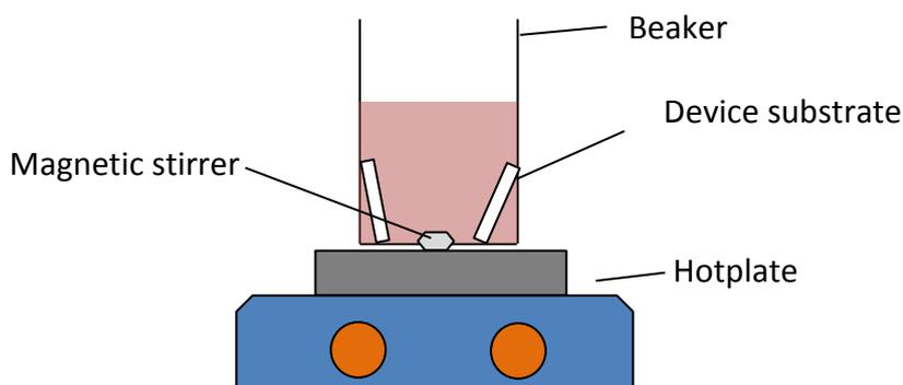
Figure 2.1. Schematic for dilute pyroneg caustic cleaning of polycarbonate substrates. Devices were immersed in the solution and heated on a low heat for 30 mins prior to device fabrication.
