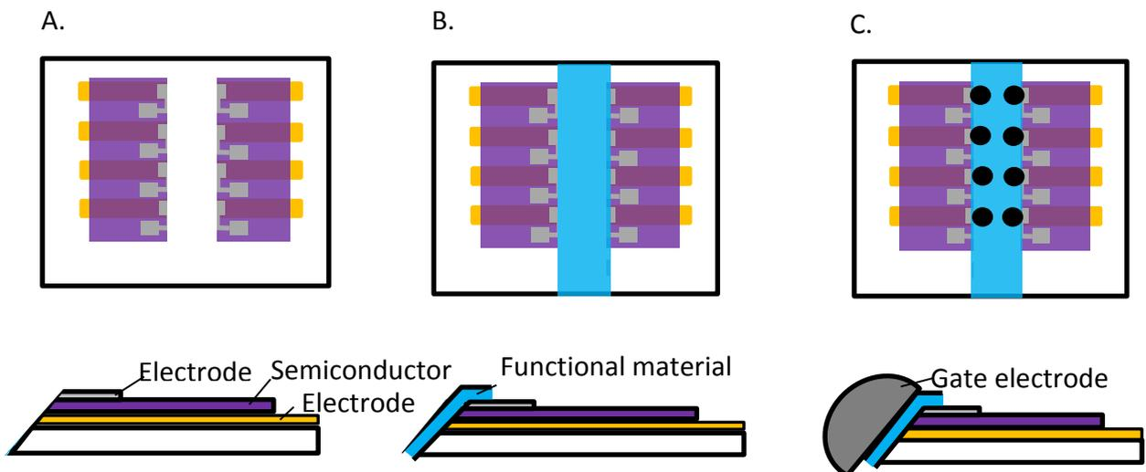
Figure 6.1. Top view and side view schematic describing deposition of dielectric material towards a three terminal device work flow. A. Cutting of two terminal device substrates. B. Dielectric film deposition. C. Gate epoxy electrode deposition.
