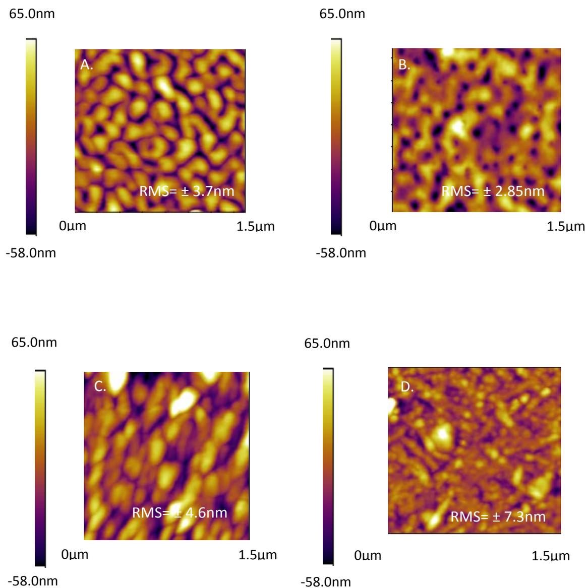
Figure 3.7. AFM images of evaporated thin films of TIPS-DBC under various processing conditions. A. 25 °C anneal temperature. B. 25°C anneal temperature with a PFBT/HDMS primer treatment. C. 50°C anneal temperature with a PFBT/HDMS primer treatment. D. 75°C anneal temperature with PFBT/HDMS primer treatment.
