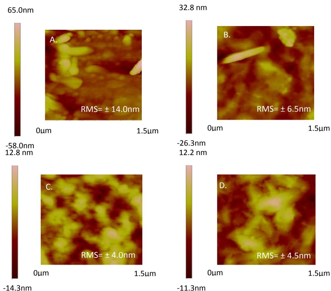
Figure 3.5. AFM images of solution processed films on top of BCB substrates .A. 1000RPM, B. 3000RPM, C. 4500RPM and D. 8000RPM.
