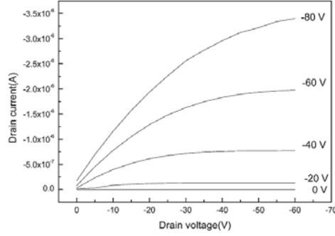
Figure 1.6. Typical output plot for a p-type accumulation device with drain voltage ( $V_{DS}$ ) being swept and that gate voltage ( $V_{GS}$ ) being stepped in 20V increments.[1]
