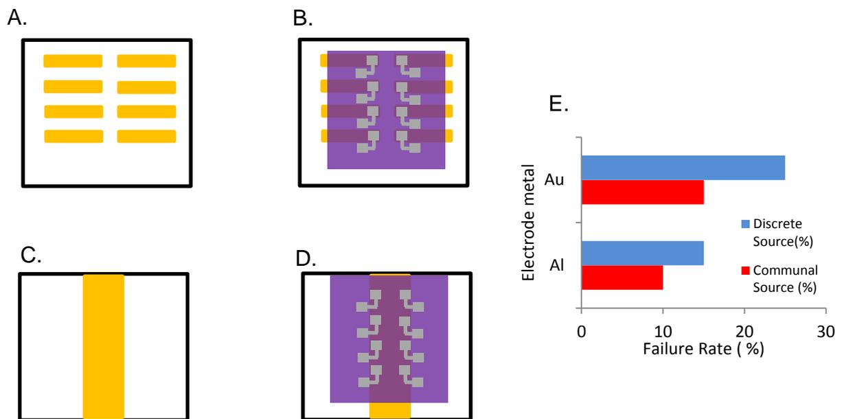
Figure 4.8. Electrode pattern schematics. A. Discrete electrode pattern. B. Resulting device fabricated with top electrode. C. Communal electrode pattern. D. Resulting devices fabricated with top electrode. Cross sectional area  $1.5\text{mm}^2 \pm 0.01\text{mm}^2$ . E. Failure Rates for gold and aluminium top electrode devices with communal (blue bar) and discrete source (red bar) pattern.
