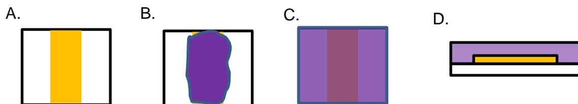
Figure 2.6. Spin coating procedure undertaken in the spin coating of thin polymeric films. A. Top view of a cleaned polycarbonate substrate with patterned electrodes. B. Top view of 10 $\mu$ L aliquot of polymer solution in solvent deposited across the centre of patterned electrodes. C. Top view of spin cast substrate between 500RPM-3000RPM creating a thin film. D. Side view of completed spin cast samples.
