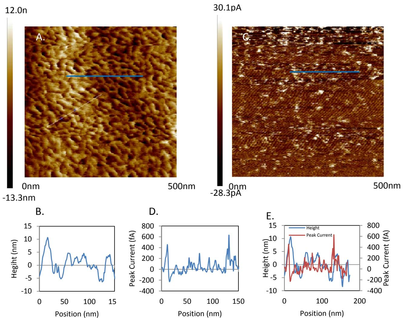
Figure 4.5. Conductive mapping of P3HT thin films A. 500nm x 500nm tapping mode height image of room temperature annealed sample with area analysed by cross section (blue line). B. Cross section analysis showing height at the location (blue line) A. C. Peak current conductive map over the imaged area. D. Cross section analysis of the peak current magnitudes with respect to location. E. Superimposed topographic height and peak current cross section traces.
