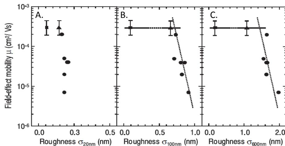
Figure 7.16. Linear regime  $\mu_{\text{FET}}$  with respect to interface roughness over three length scales with an evaluated gate field  $2\text{-}3\text{ MVcm}^{-1}$  as produced by Sirringhaus *et al.*[16] A.  $\delta_{20\text{nm}}$  B.  $\delta_{100\text{nm}}$  C.  $\delta_{600\text{nm}}$ . Straight lines are used as a visual guide of correlation.
