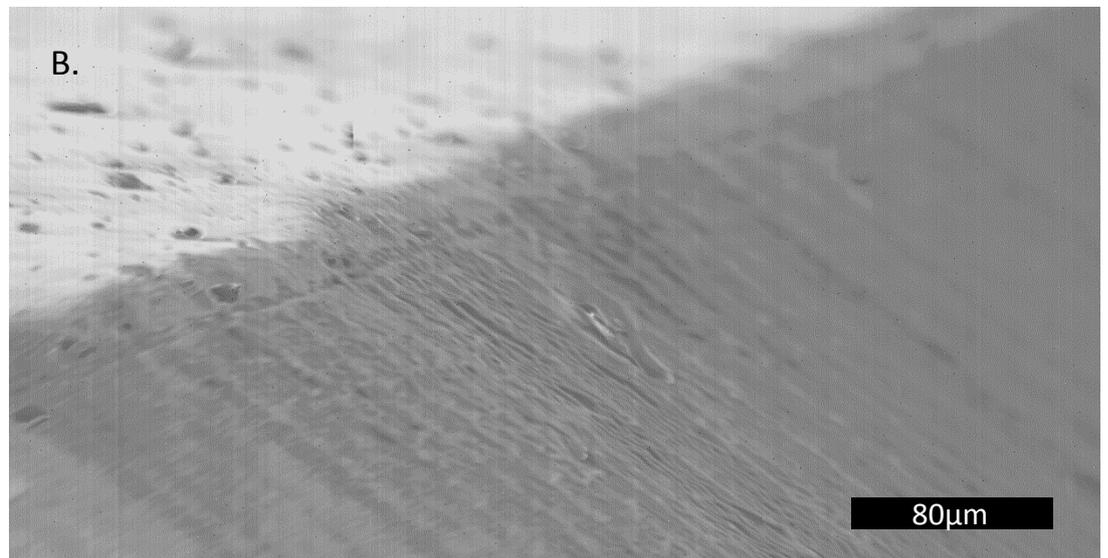
Figure 6.6. Scanning electron microscope images of two terminal device substrates before solution processing of a functional material. A. Macro scale Image taken down the axis of the vertical cut showing the vertical wall down the distance of the substrate. B. Zoomed in at the surface cut edge at the top electrode.
