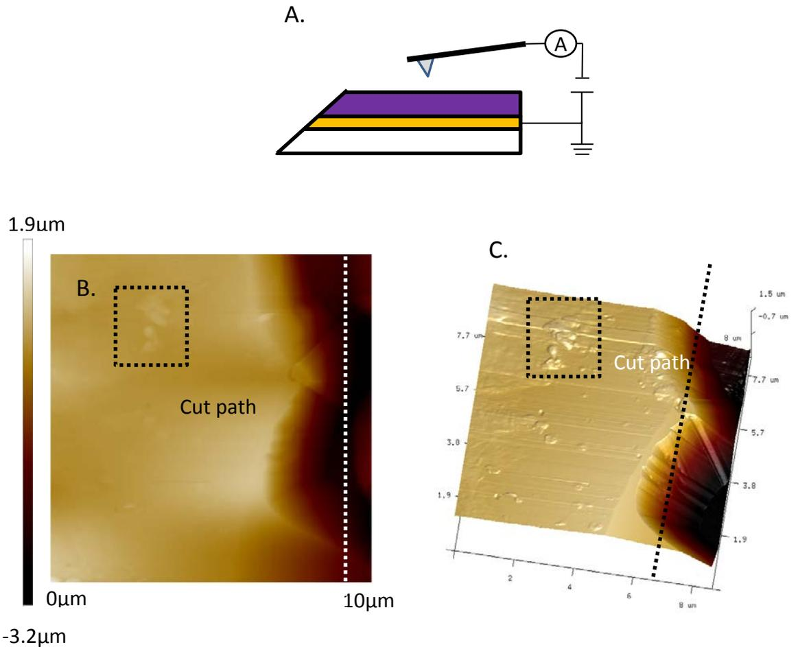
Figure 5.10 . Obtained topographic images of the cut edge A. Experimental schematic showing biases applied. B.10μm x 10μm AFM tapping mode height image of the cut-polymer interface. C. Three-dimensional topographic image of the tapping mode two dimensional image.
