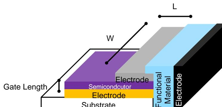
Figure 1.20. Schematic for a general vertical electrical platform. With physical parameters width ( $W$ ), length( $L$ ) and gate length labelled.
