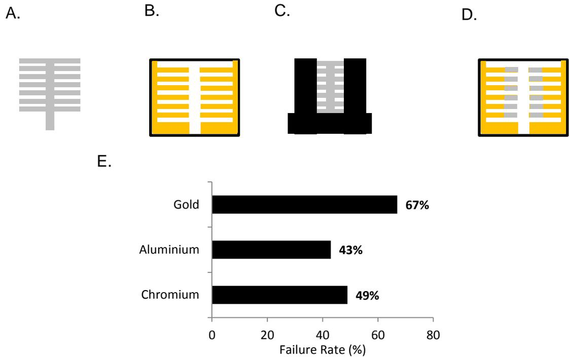
Figure 4.6. Electrode patterning work flow for a manually aligned shadow mask featuring a rib cage design allowing thin  $\sim 0.2\text{mm}$  wide devices. A. Manually aligned rib cage shadow mask. B. Resulting patterned electrode post metal deposition. C. Manually aligned rib cage mask with functional taping. Resulting patterned top electrode. E. Failure rate for devices with various sputtered metal electrodes gold, aluminium and chromium.
