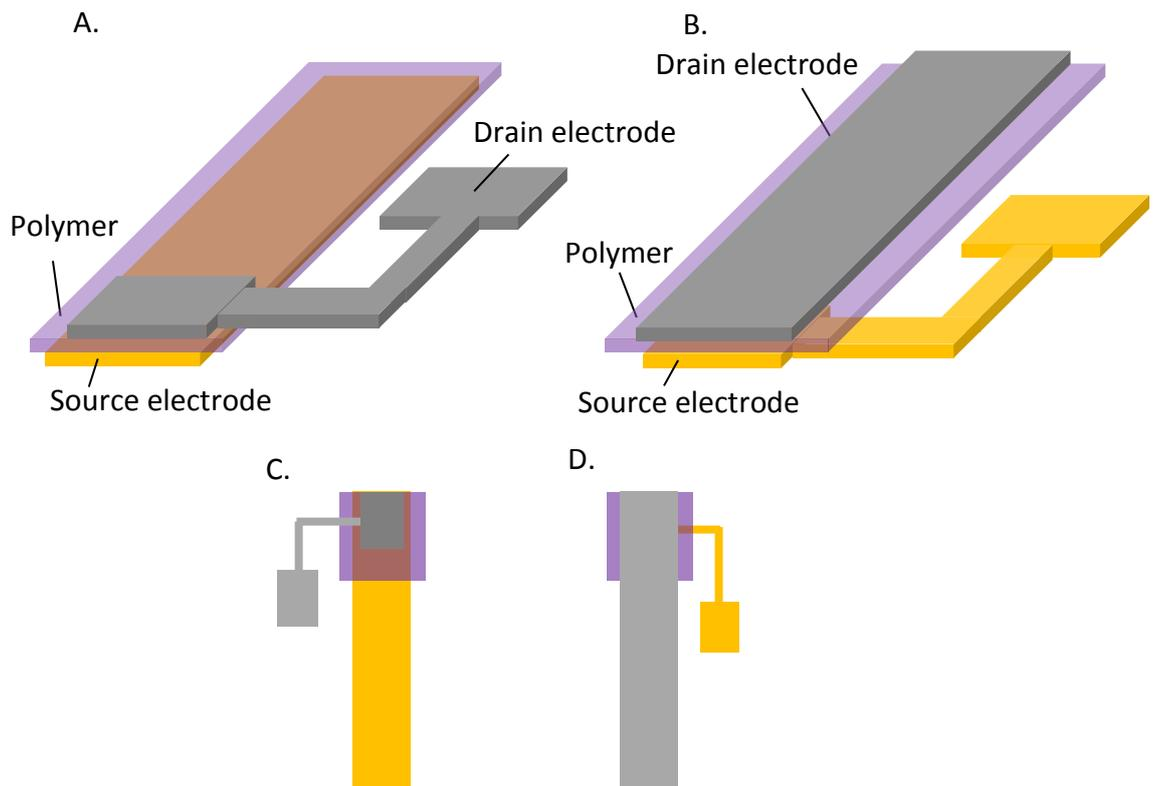
Figure 6.9. Graphical schematic of batch processed electrode patterns. A. Standard electrode pattern. B. Encapsulating electrode pattern .C. Top down schematic view of the showing standard electrode pattern D. Top down schematic view of the showing encapsulating electrode pattern.
