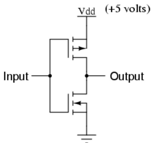
Figure 1.2. CMOS Inverter logic circuit. The logic circuit operates utilising an p-type FET (top) and an n-type FET (bottom). The circuit is the basis for digital logic circuits. The power usage and speed of transistors in the circuit is a key performance criteria in logic applications determining
