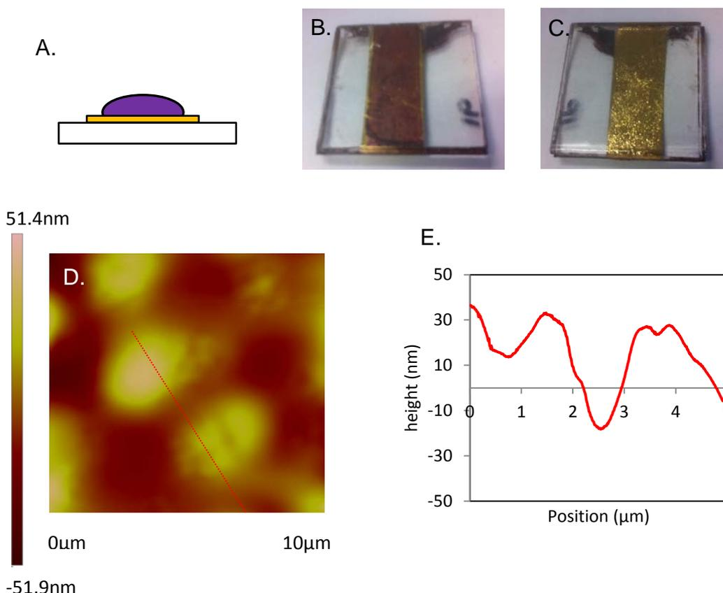
Figure 4.1. Atomic force microscope images on devices with observed stress cracking behaviour. A. Deposition schematic. B. Device substrate after the solution deposition of thin film. C. Underside of device substrate after thin film deposition D. 10µm x 10µm topographic image of top electrode in completed device. The area analysed through cross-section measurement indicated by the red line E. Cross section height analysis of polymer surface.
