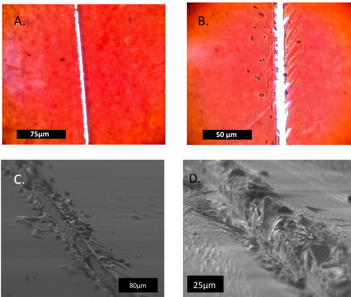
Figure 5.1. Optical and scanning electron microscope images of vertical wall architecture introduced by hot scalpel cutting. A. Optical microscope image of scalpel cut. B. Zoomed in optical microscope image of scalpel cut substrates. C. Scanning electron microscope image of hot scalpel cut. D. Zoomed in scanning electron microscope image showing the top interface of the cut surface and topographic features of the scalpel cut.
