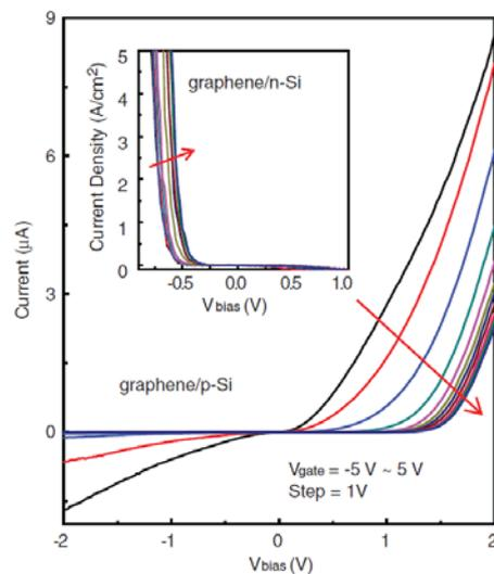
Figure 1.20. Three terminal graphene barristor output plot A. P-type silicon output plot. Potential voltage  $V_{ds} = \pm 2V$  whilst gate potential,  $V_{GS}$  is swept  $-5V$  to  $5V$  in  $1V$  increments. INSET- N-type silicon output plot. Potential voltage  $V_{ds} = \pm 1V$  whilst gate potential,  $V_{GS}$  is swept  $-5V$  to  $5V$  in  $1V$  increments.
