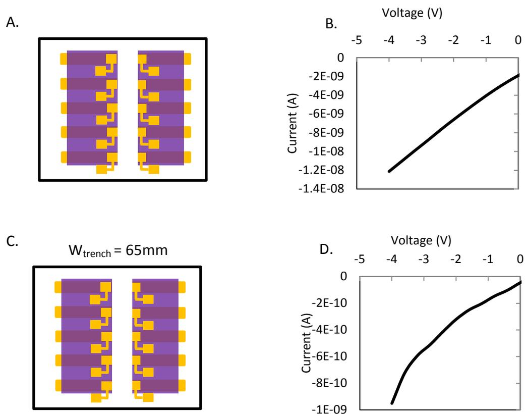
Figure E1. Reduction of operational area through increased trench width. A. Initial machine cut trench with width  $w = 42\text{mm}$ . B. 3 device average forward current with trench width = 42mm C Reduced operating area device with increased trench width of 62mm. C. 3 device average forward current with trench width = 65mm.
