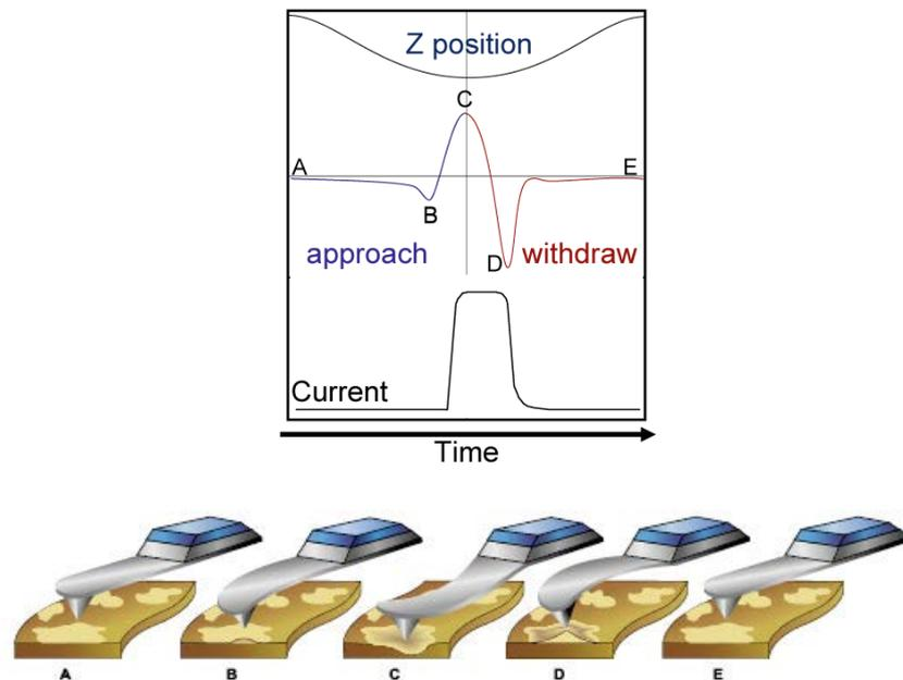
Figure 2.12 A. Force-distance forces experienced by a tapping mode probe during an approach and withdraw cycle. B. Schematic representation of probe position relative to sample surface.[1]
