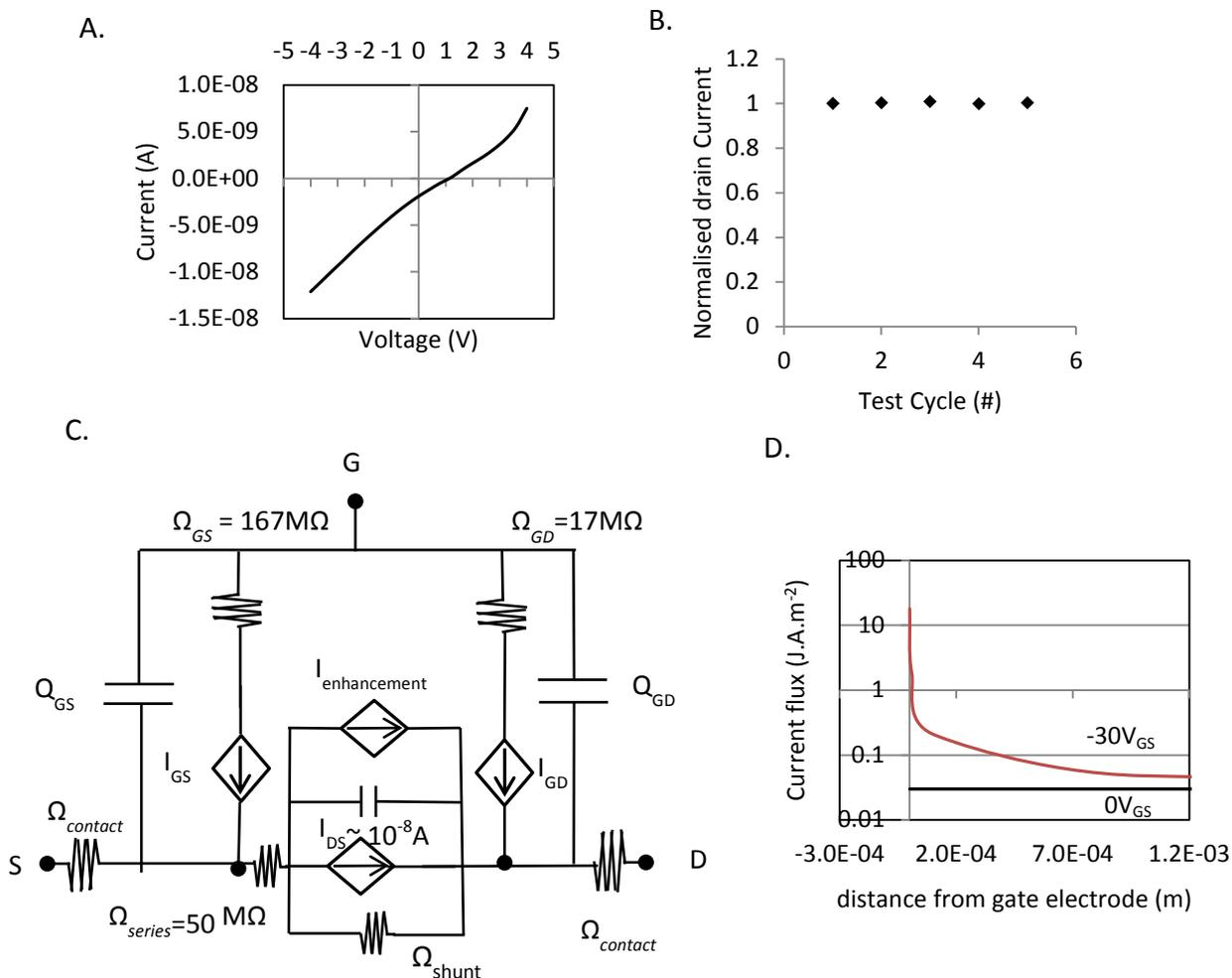
Figure 7.13. A. Proposed equivalent circuit for PCDTBT based OFET devices. B. Source-drain equivalent circuit for a thin film schottky showing series resistance and OFF state currents. C. Source-drain equivalent circuit with labelled series resistance and OFF state current. D. Current flux profile for the active layer at  $V_{GS}=0\text{V}$  (black line) at an applied  $V_{GS}=-30\text{V}$ .
