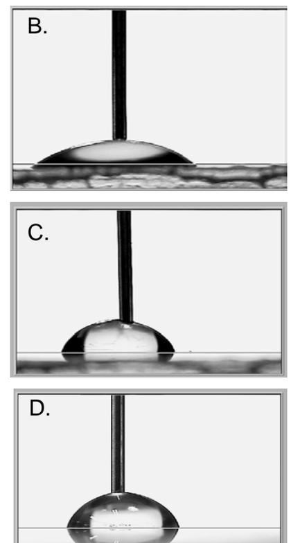
Figure A.4. Contact angle vs. time for evaporated (blue dots) and evaporated (red dots) gold samples. Example digital capture of obtained contact angle droplets for A. 1,2-DCB on cleaned Au after 30mins. B. 1,2-DCB on UV-NVS cleaned surface after 60mins C. Pyroneg cleaned UV-NVS with water D. Cleaned Au with water droplet.
