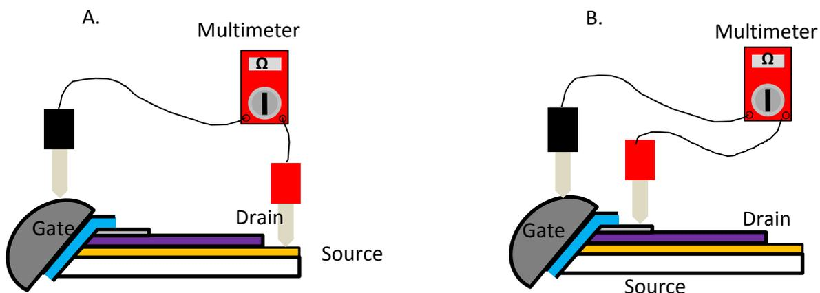
Figure 6.3. Failure analysis for three terminal devices A. Gate-source failure testing. B. Gate-drain failure testing.
