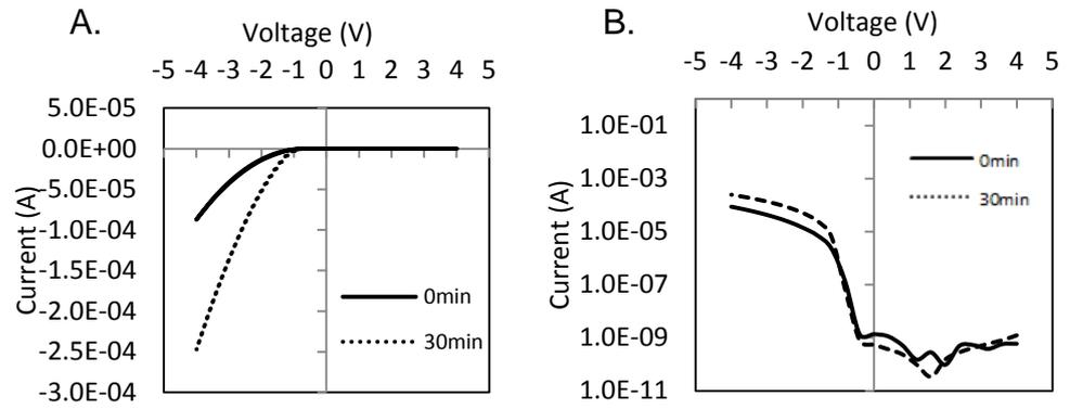
Figure 4.11 .Two terminal Schottky barrier device current-voltage characterisation immediately after fabrication. A. -/- quadrant output plot over a 30 min testing period. Initial trace (solid line) and after 30mins testing (dashed line) B. Log vs. V characteristic plot for two terminal Schottky barrier devices. Devices were tested in a nitrogen environment after the deposition of evaporated aluminium.
