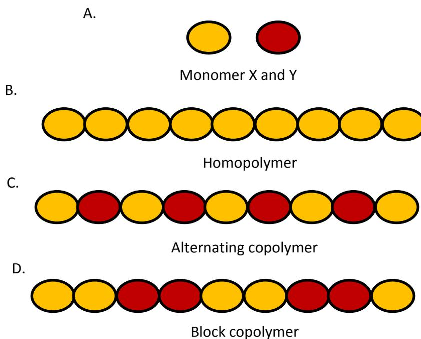
Figure 1.8. Schematic representation of polymer classification and the resulting polymer matrix. A. Discrete monomers X and Y. Monomers are individual molecules that may bond to create a polymer with the arrangement of monomers classifying the polymers. B. Homopolymers comprised of a discrete monomer repeating unit. C. Alternating co-polymers comprised of alternating monomers. D. Block co-polymers comprised of blocks of monomer units.
