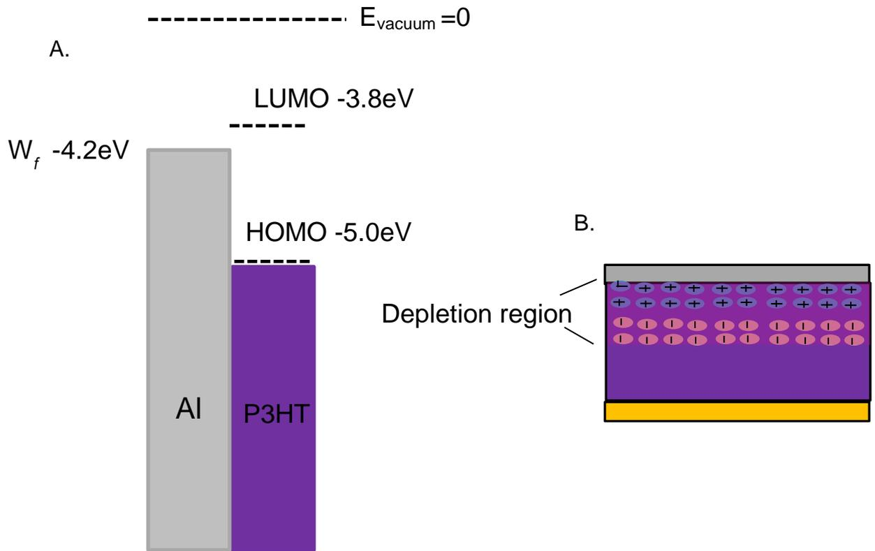
Figure 1.17. A. Energy level schematic of the aluminium-organic interface. B. Depletion region sketch within a two terminal schottky barrier device.
