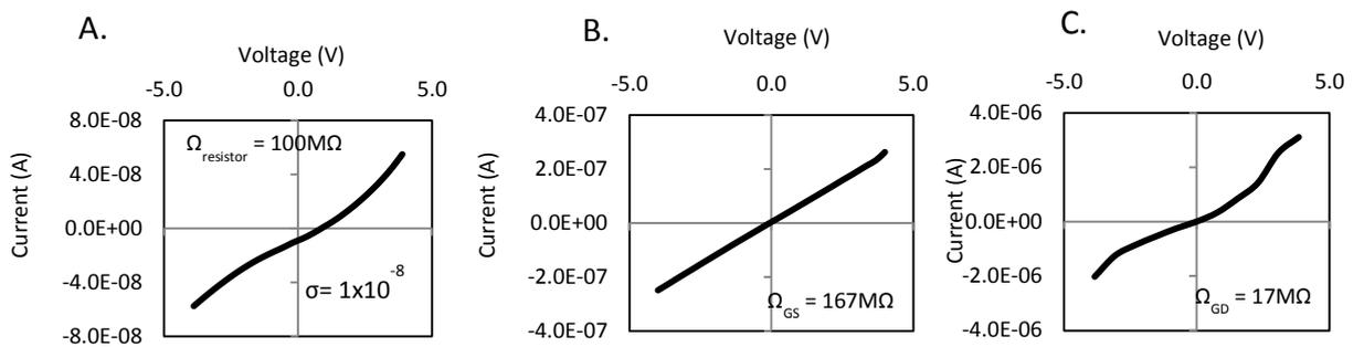
Figure 6.4. UV-NVS resistance measurements taken from leakage current-voltage characteristics for epoxy gated three terminal devices with UV-NVS spin coated dielectric material. Devices are an average compiled over 10 devices on 3 substrates. A. Current-voltage characteristic for a two terminal UV-NVS resistor cell. B. Gate-source leakage current. C. Gate- drain leakage current.
