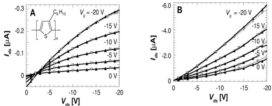
Figure 1.15. A. Obtained output electrical characteristics of planar OFET devices fabricated through solid state embossing. B. Obtained output plot of VOFET devices. A lack of saturation is observed in output plot for vertical devices.
