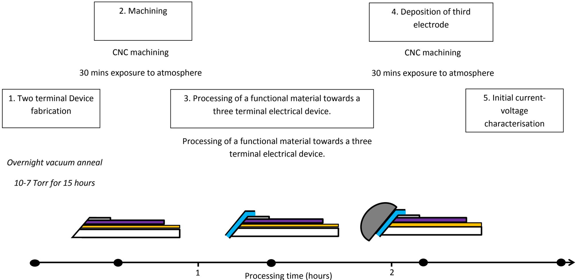
Figure 2.9. Device processing flow chart towards a three terminal device showing experimental work flow. 1. Two terminal device processing using the sequential processing methodology 2.CNC machine cut introducing a vertical wall. 3. Processing of a functional material towards a three terminal device. 4. Deposition of gate electrode. 5. Initial current-voltage characterisation.
