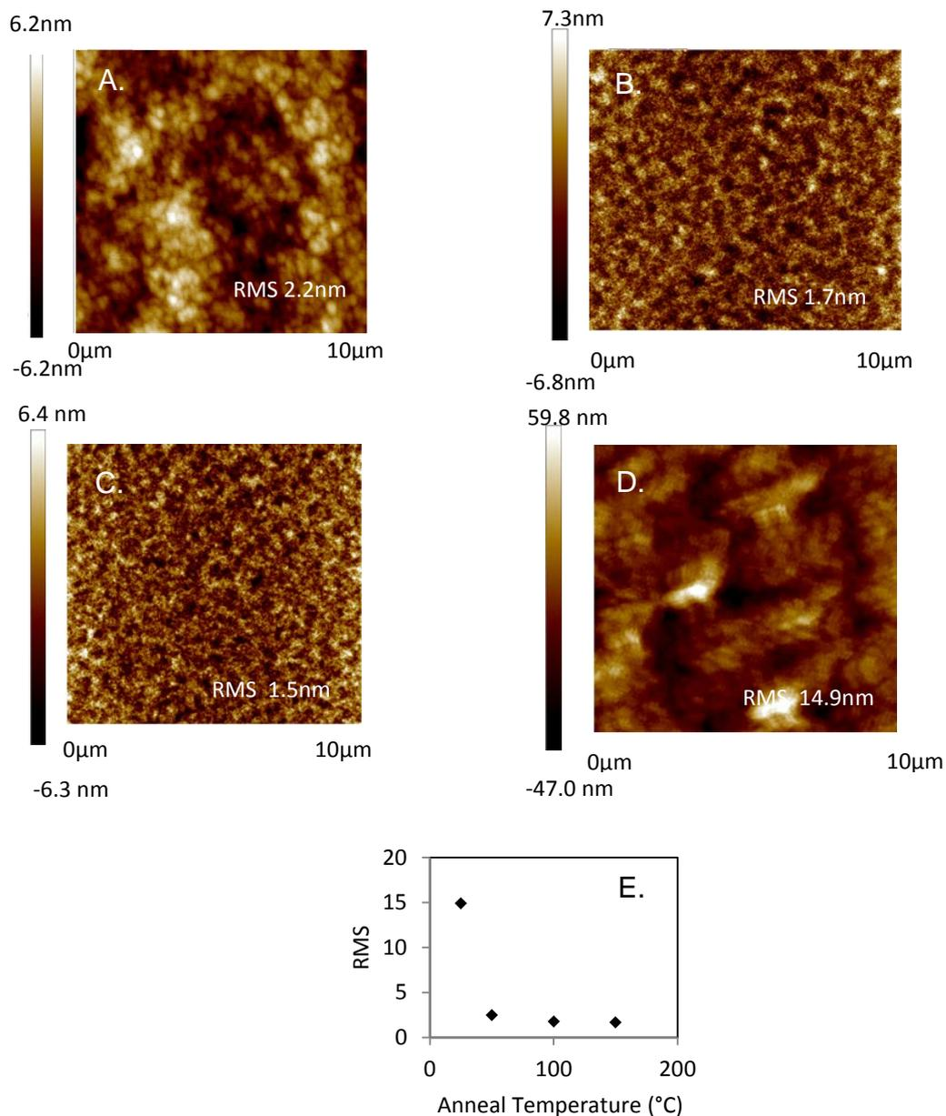
Figure 4.3. Comparison of 10um x 10um AFM height images of P3HT thin films with varying annealing temperatures A. 50°C , B. 100°C, C. 150°C and D. Room temperature. E. RMS roughness plotted with respect to anneal temperature.
