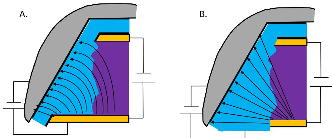
Figure 7.15. A. Polymer delamination at the polymer-gold interface and B. Gold delamination at the gold-polycarbonate interface. The architectures represent deviations from the ideal device architecture resulting in non-ideal lateral electric fields. Schematic depiction of possible lateral electric fields and resulting charges induced at the semiconductor-dielectric interface.
