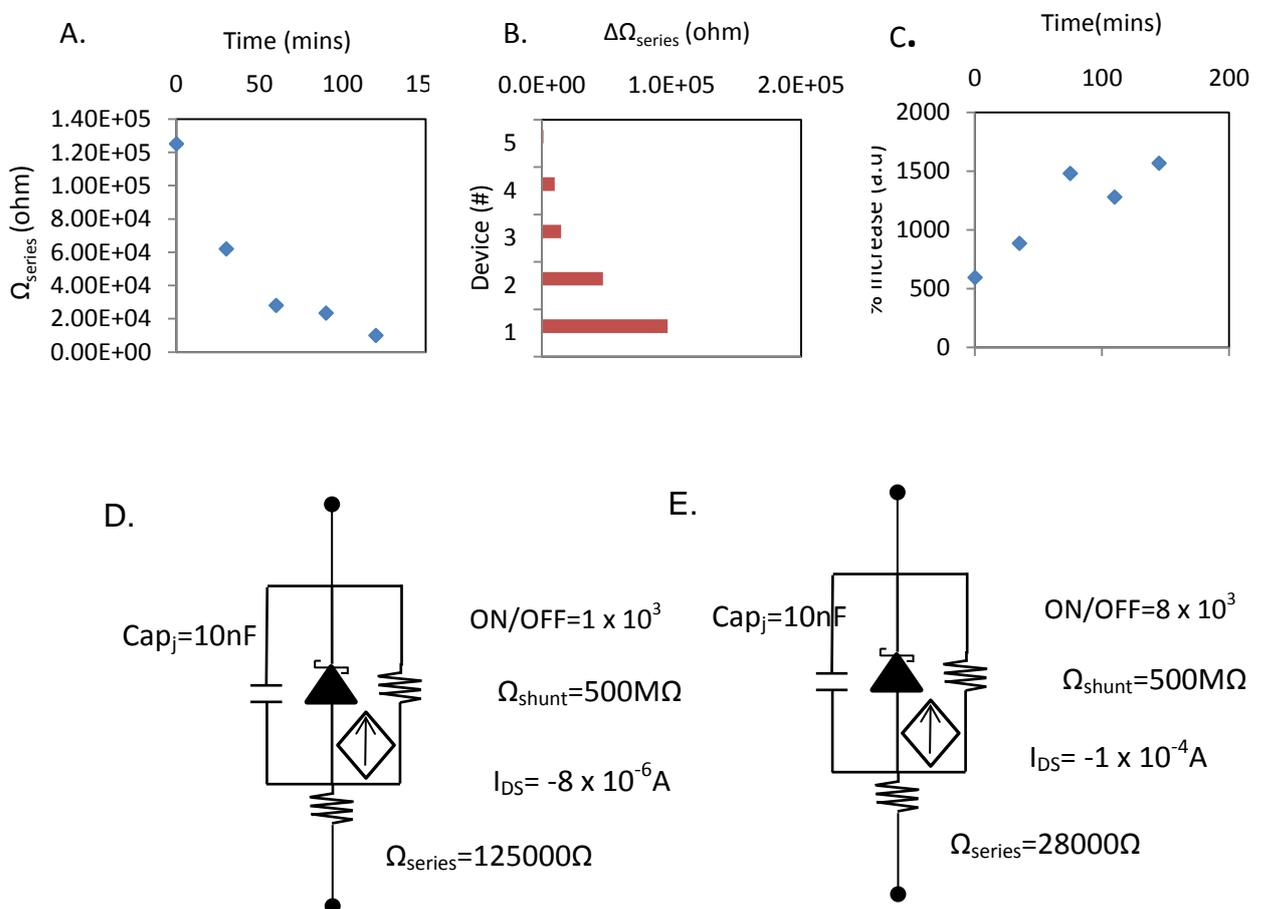
Figure 4.13. Equivalent Circuit behaviour for an immediately tested device substrate. A. Simulated series resistance of devices with respect to time after electrode deposition. B. Changes in series resistance over 30mins of consecutive testing. C. Percentile increase in forward current with respect to time after electrode deposition. D. Simulated equivalent circuit for a device immediately removed from vacuum E. Simulated equivalent circuit after 30mins of consecutive testing.
