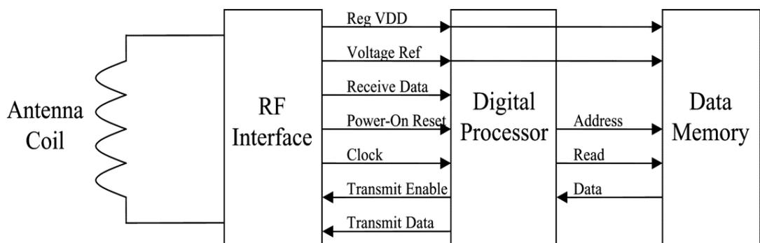
Figure 1.11. Block diagram of an RFID device. The critical components in reading, writing and erasing data are described. Critical to the implementation of the FRID is the antenna coil capable of turning the radio frequency data from a RFID reader into computable information.
