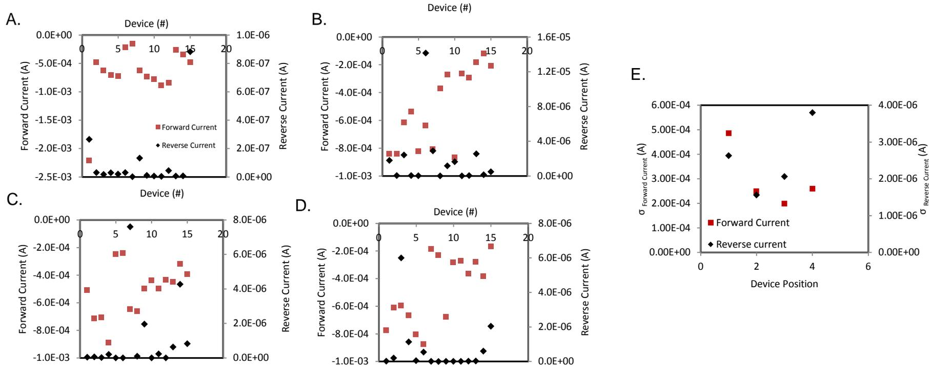
Figure 4.17. Distribution of forward current (red) and reverse currents (black) with respect to device position and the resulting standard deviation. A. Distribution of currents in position 1. B. Distribution of currents in position 2. C. Distribution of currents in position 3. D. Distribution of currents in position E. Calculated standard deviation by device position.
