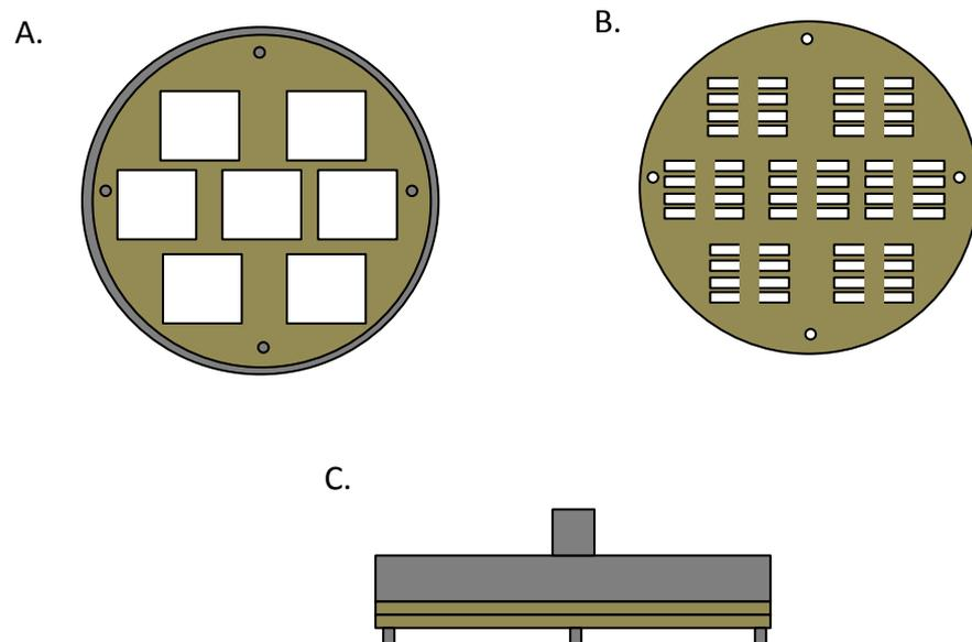
Figure 2.2. Batch metal evaporation for device substrates. A. Sample holder tray. B. Example source electrode shadow mask C. Side-on view of evaporator sample mount.
