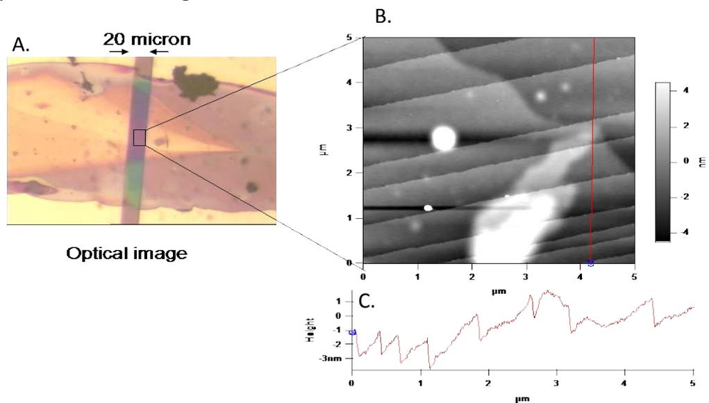
Figure 3.6. A. Optical image of thin film processed by drop casting producing large crystals on top of the source-drain Au electrodes. B. 5µm x 5µm AFM topography image. C. height profile across surface environment.
