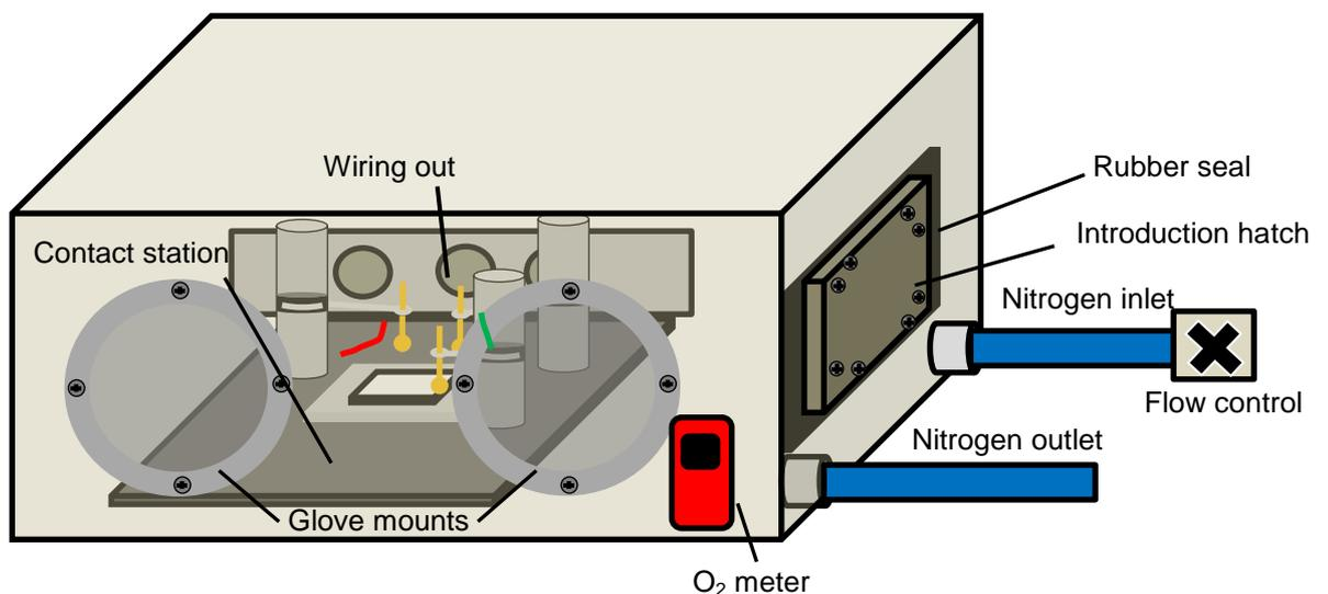
Figure 2.16. Schematic of inert testing chamber during testing procedure. The chamber allowed for testing in an inert atmosphere. An  $O_2$  meter allowed for the monitoring of oxygen levels in the environment.
