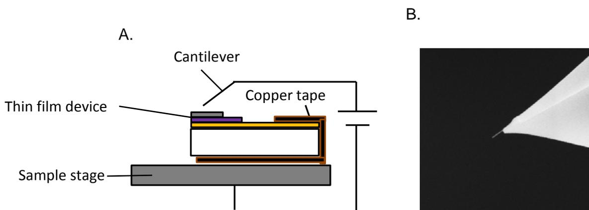
Figure 2.13. Experimental schematic for conductive AFM. A. PF-TUNA sample stage with applied biases during conductive mapping. A double sided copper tape is used to make electrical contact with the sample. A completed device is mounted with the copper tape providing a contact with a terminal in the thin film device. B. High resolution PtIR cantilever tipped with a carbon nanotube attached from the functional end of the probe as developed by Stapleton *et al.*
