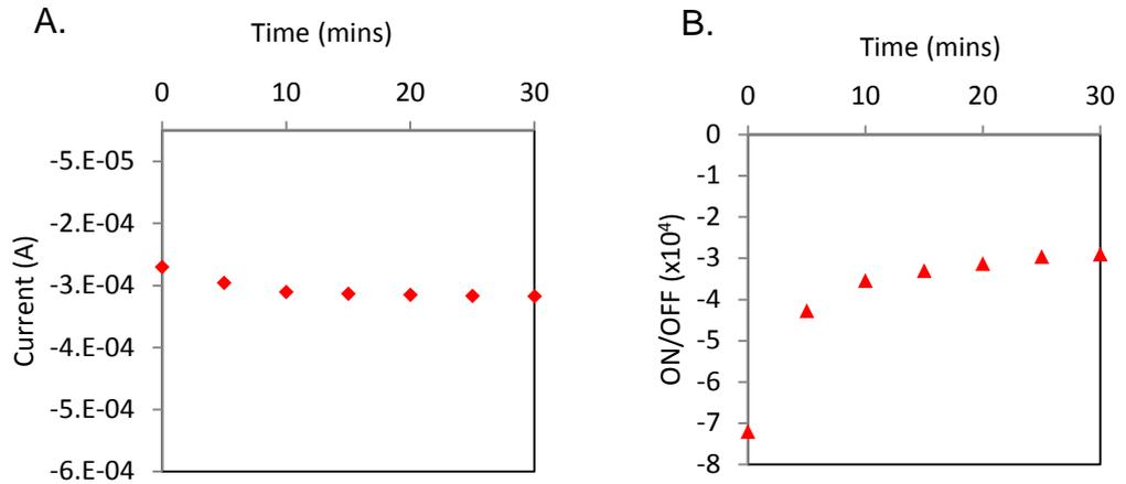
Figure 4.15. Forward current increases in vacuum stored devices as a function of time over 30mins of testing. A. Forward current performance. B. Rectification ratio over 30mins testing.
