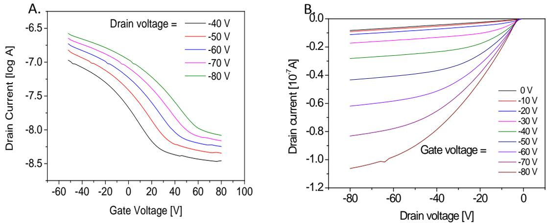
Figure 3.2. I-V characteristics of spin cast TIPS-DBC devices. A. Transfer curve with gate voltage sweeping from -50 V to 50 V and B. output curve with gate voltage ramped to -80 V. Measurements were taken under room temperature in a nitrogen environment.
