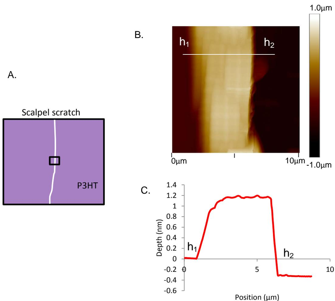
Figure A.1. Example of P3HT step height calculation. A. Schematic of scratched sample. B. Example height profile obtained across scalpel cut. C. 2D section analysis showing step height (nm) vs. position analysis. A step height of 276nm was obtained in this example.
