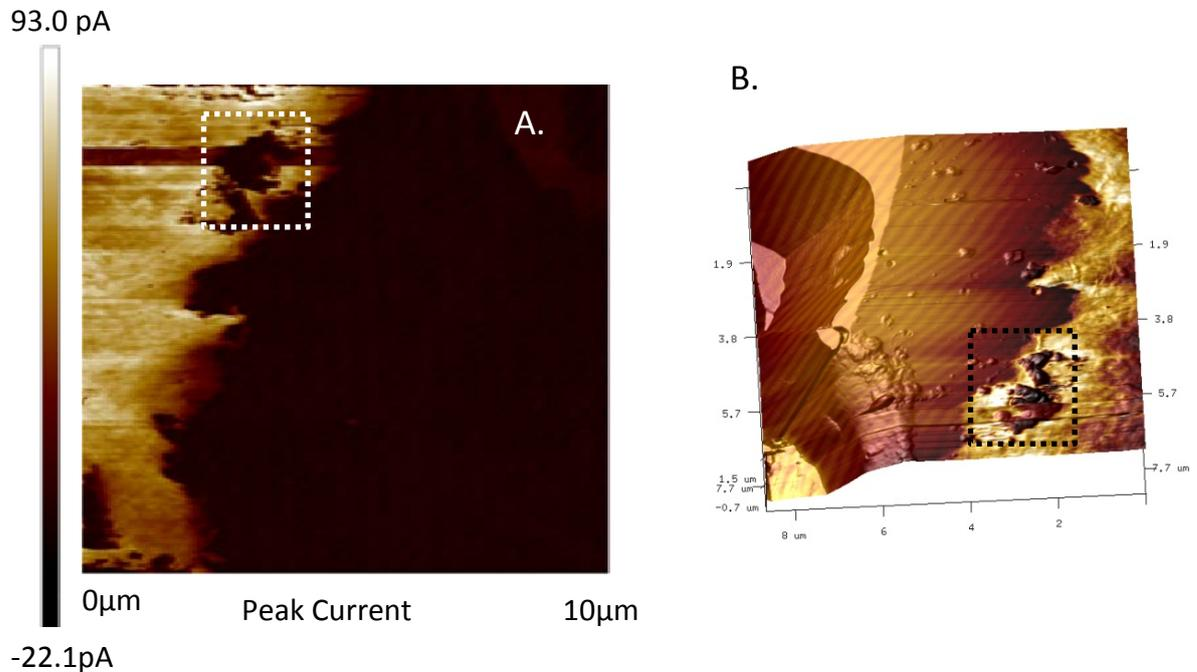
Figure 5.11. Conductive AFM conductive map and corresponding 3D render of the cut edge A. 10 μm x 10 μm AFM peak current image. B. Rotated three dimensional render of the topographic height image with superimposed peak current map.
