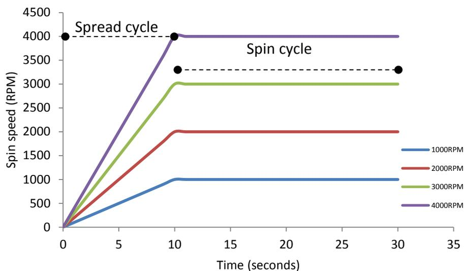
Figure 2.5. Spin coater spin speed vs. time pre-programmed deposition cycles for four recipes. 1000RPM (blue) 2000RPM (red) 3000RPM (green) 4000RPM (purple).
