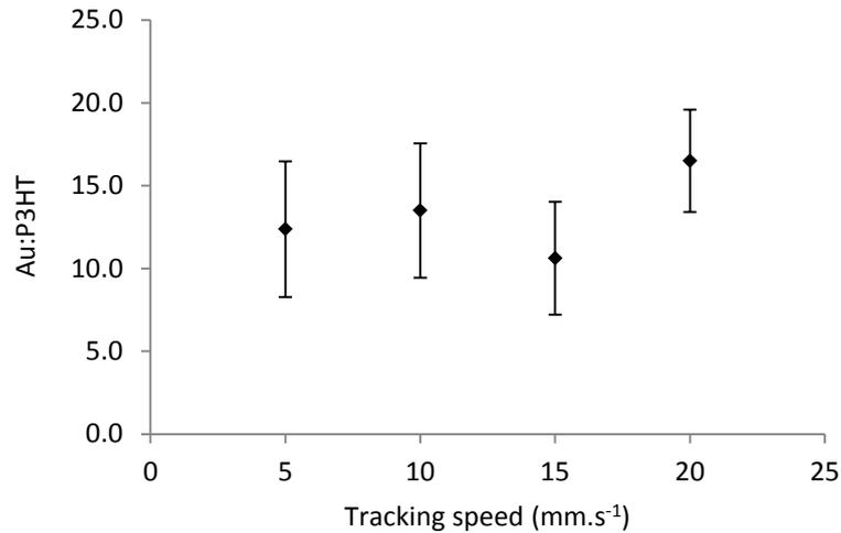
Figure 5.9. Gold adhesion failures at the electrode-cut interface with respect to CNC circuit board spindle head tracking speed. Error bars represent the standard error corresponding to a 68% confidence interval.
