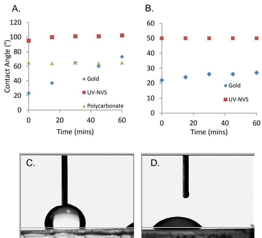
Figure 4.2. Contact angle measurements with respect to time. A. Water contact angle for UV-NVS (red square), polycarbonate (green triangle) and gold (blue diamond). B. 1,2-dichlorobenzene contact angle for UV-NVS (red square) and gold (blue diamond). C. Optical image of water droplet on UV-NVS film. D. Optical image of 1,2-dichlorobenzene droplet on UV-NVS.
