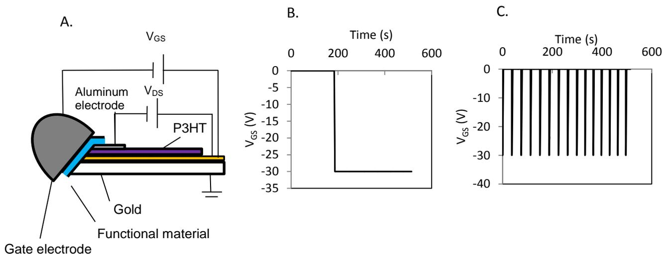
Figure 7.7. Planar schematic of two terminal Schottky substrates and gate input signals. A. Cross section and biasing schematic of a discrete device. B. Turn on gate signal input in which  $-30V_{GS}$  is applied turning the device from an OFF ( $0V_{GS}$ ) to ON state C.  $-30V$  gate signal input turning the device from an OFF state to an ON state. Source-drain current were measured under the incident signals to determine drain current magnitude during the applied signal.
