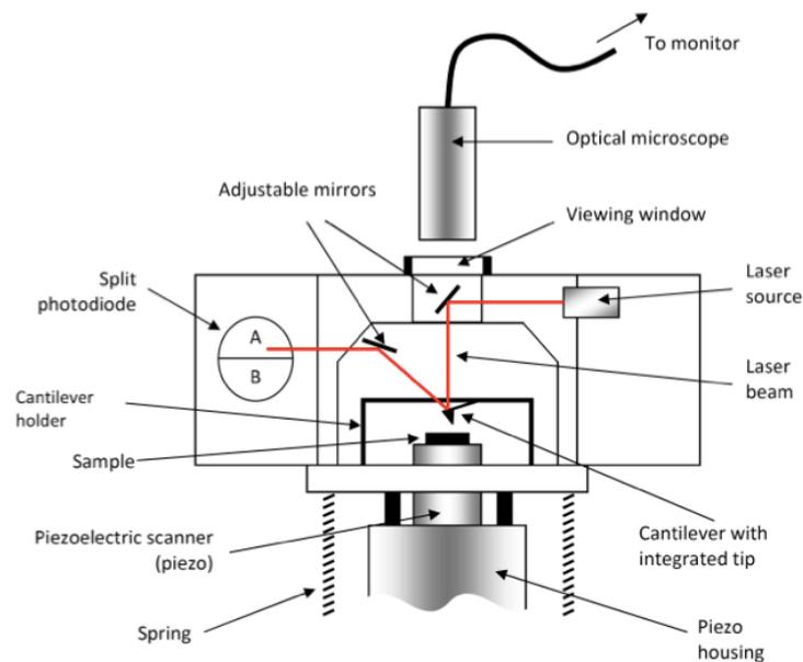
Figure 2.11. Schematic representation of atomic force microscope in operation. Surface topography is mapped through a feedback loop monitoring the oscillation of the cantilever across the surface as it undergoes chemical interactions. A piezoelectric scanner rasters across the x-y direction of the surface as the feedback loop controls the z-positioning relative to the sample[1]
