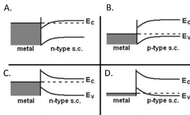
Figure 1.5. Energy level diagrams describing charge injection at the source electrode under varied electrical conditions. A. n-type material at 0 gate bias, B. p-type at 0 gate bias, C. n-type material at positive gate bias, D. p-type at negative gate bias
