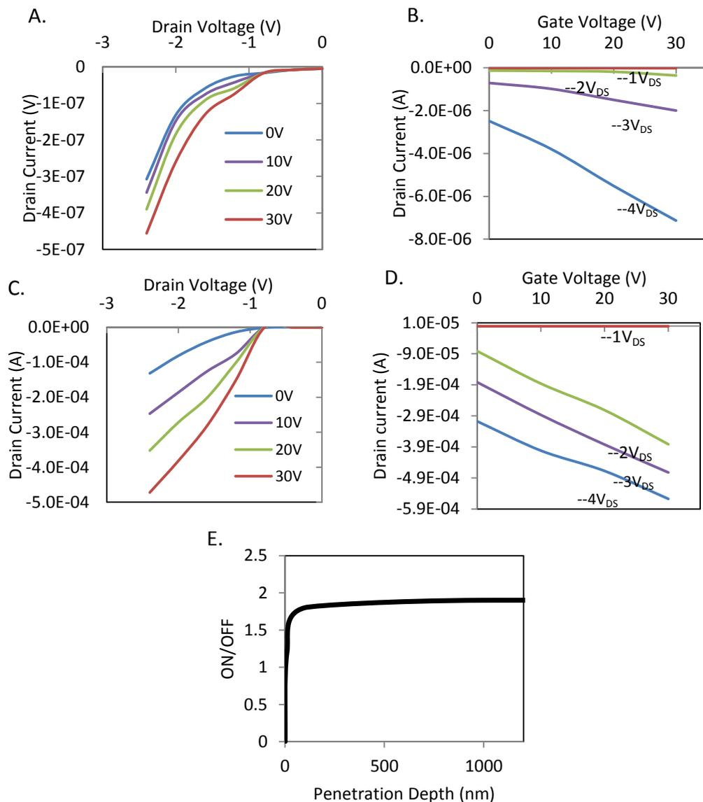
Figure 7.5. Simulated transistor performance. A. Output plot for 20 $\mu\text{m}$  active layer thickness. B. Transfer plot. C. Output plot for 225nm active layer thickness. D. Transfer plot. E. Role of penetration depth on transistor performance.
