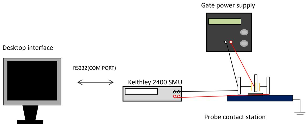
Figure 2.14 Electrical characterisation schematic. Current-voltage measurements are obtained via integration of a source-meter unit with a PC loaded GUI via an RS232 com port. A Floating source potential is applied through the source-meter unit and a secondary power supply unit can supply a floating gate potential. Electrical characterisation through this apparatus is capable of 10uA measurement accuracy of 0.1nA. Range of 2V measurement accuracy of 10uV with a voltage ramp  $0.65V.s^{-1}$
