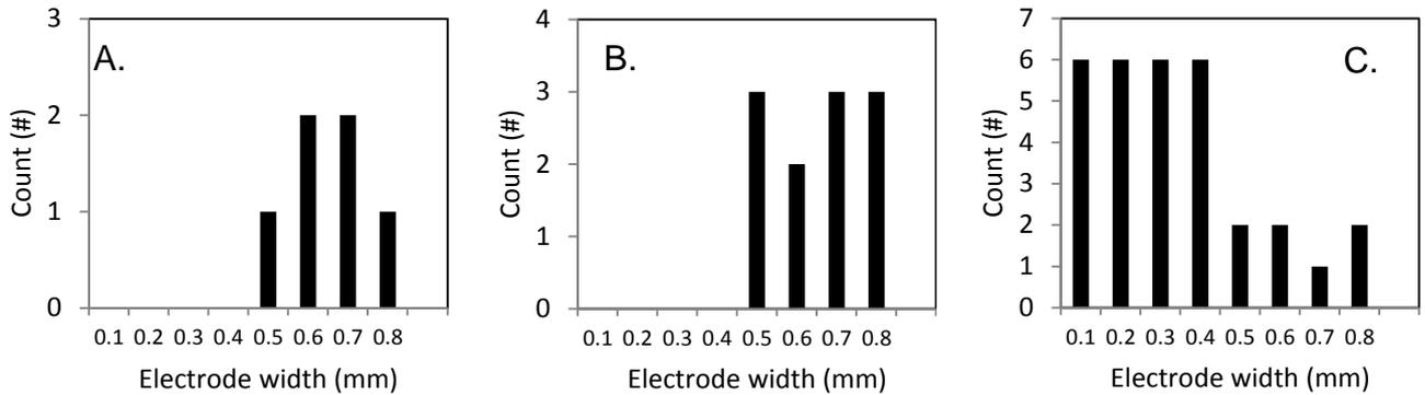
Figure D.2. Histogram plots for lift-off technique in the fabrication of layered device structures on flexible PET substrate.
