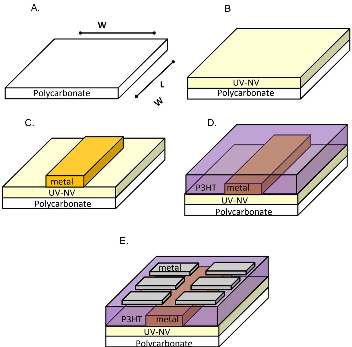
Figure 2.8. Device fabrication. A. Commercial polycarbonate sheets are laser cut to  $25.4\text{mm}^2$  with an accuracy of  $\pm 0.01\text{mm}^2$  and used as a working substrate. B. UV-NVS resin is spin coated onto the surface. C. A working electrode metal is deposited by means of sputtering or evaporation through a shadow mask. D. The semiconducting polymer P3HT is spin cast from solution onto working electrode and annealed. E. A second working electrode is deposited through shadow mask.
