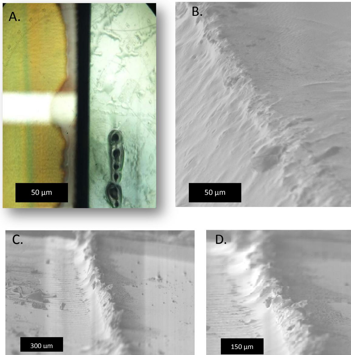
Figure 6.5. Microscopy images of UV-NVS coating on two terminal device substrates. A. Top-down optical microscope image of the cut edge with a UV-NVS coating completed over an aluminium electrode edge. B. Scanning electron microscope image of a coated cut surface C. Coated device substrate with polymeric active layer peeled off showing UV-NVS morphology over the cut edge. D. Zoomed in image of the morphology of UV-NVS at the cut edge.
