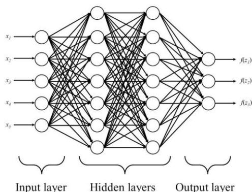
Fig. 5. Artificial neural network showing an input layer, two hidden layers and an output layer.
