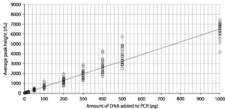
Figure 9.2 Average peak height for GlobalFiler profiles produced on a 3130xl with varying amount of input DNA.
