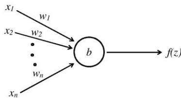
**Fig. 4.** A single neuron showing inputs ( $x$ ), weights ( $w$ ), bias ( $b$ ) and output ( $f(z)$ ).
