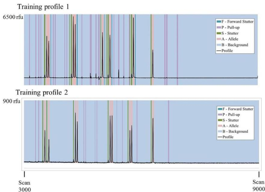
**Fig. 8.** Two 6-FAM training data sets used to train the ANN showing scans and approximate intensity in relative fluorescent units (rfu) as produced on a 3130xl (Life Technologies).
