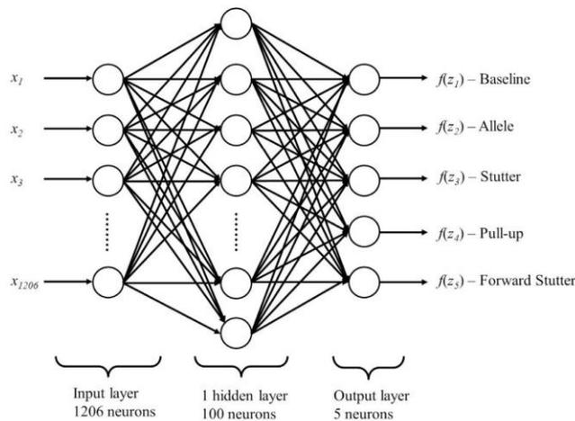
Fig. 7. ANN used in this study for classifying electrophoretic signal.
