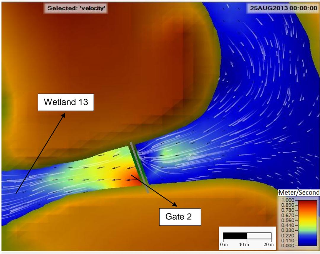
Figure 15 Velocity profile and fluid movement through Gate 2(fully opened) on 25th August
