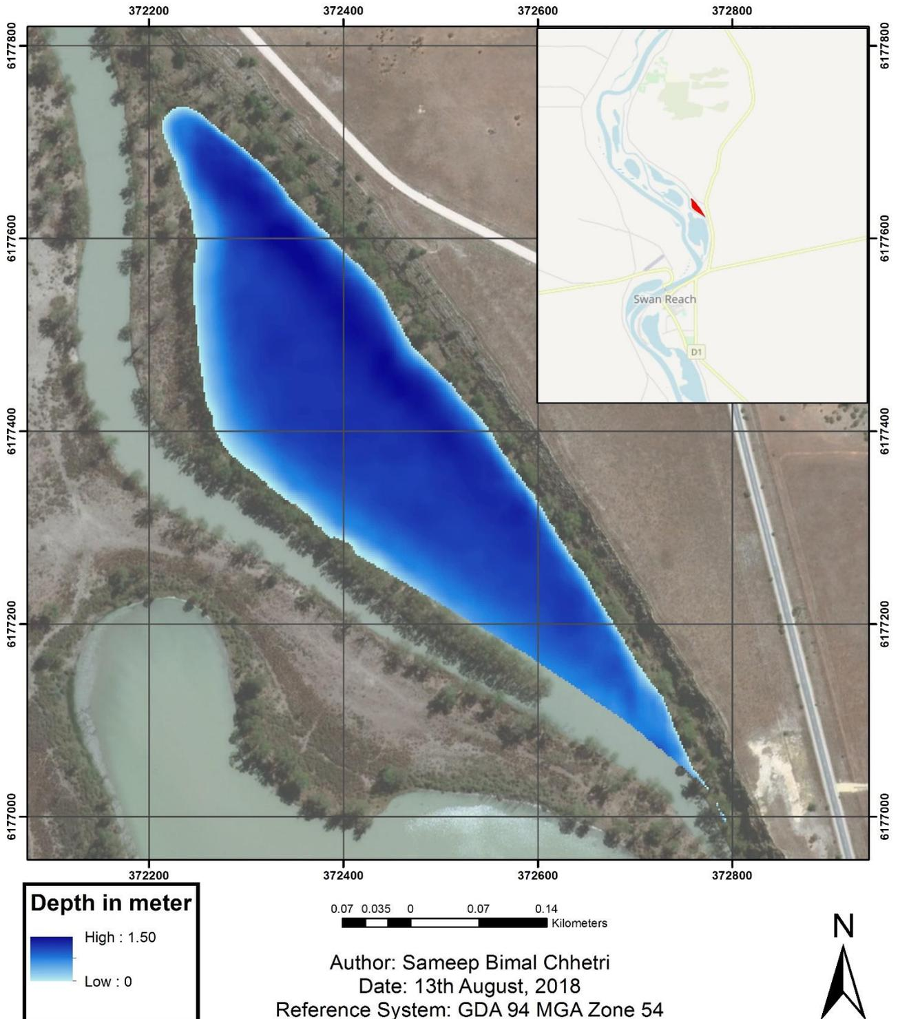
Figure 27 Maximum inundation map for wetland 12
