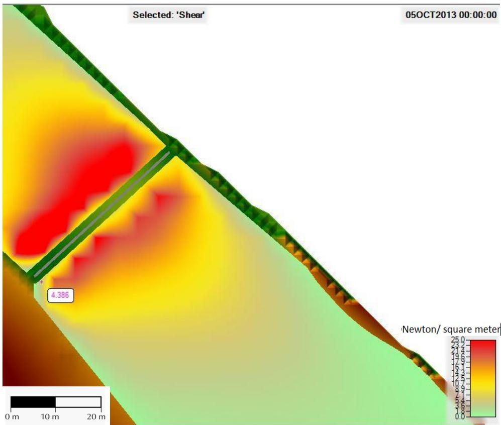
**Figure 49 Local shear stress levels at gate 1 (open)**
