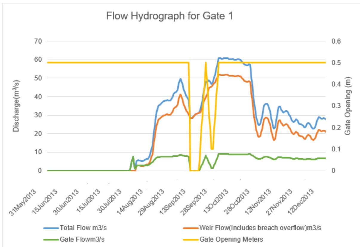
Figure 9 Flow hydrograph for Gate 1
