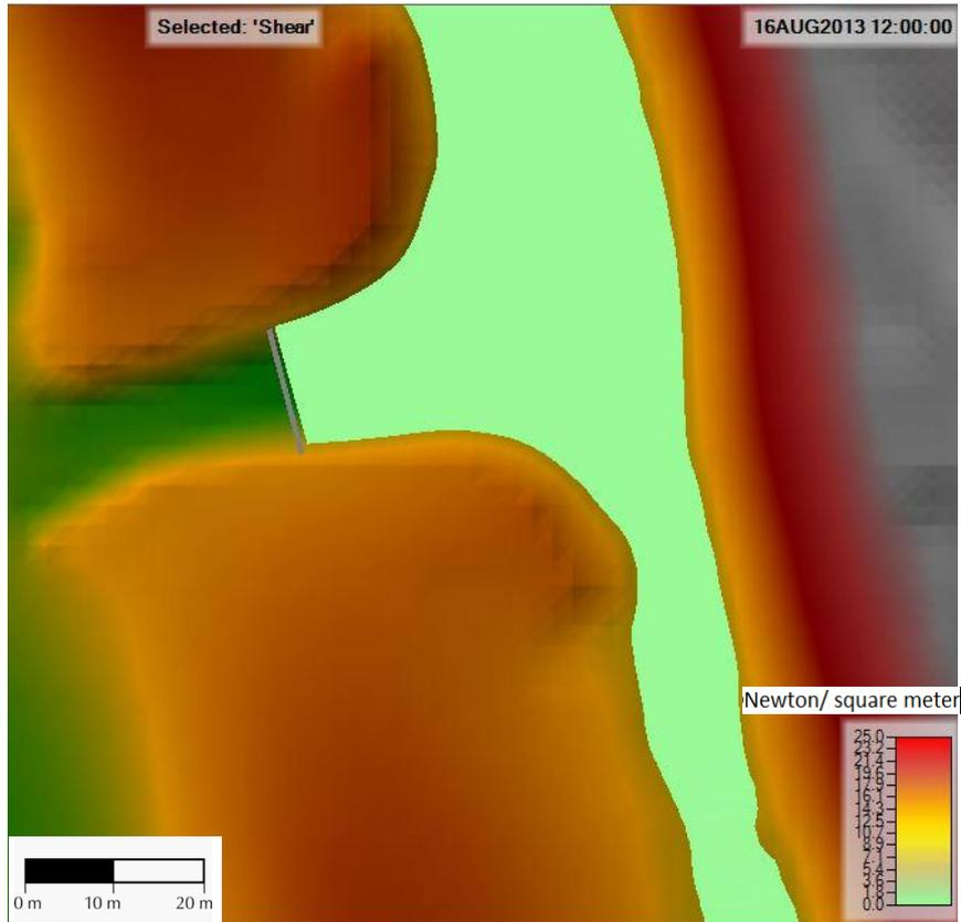
Figure 205 Local shear stress levels at gate 2 (closed)
