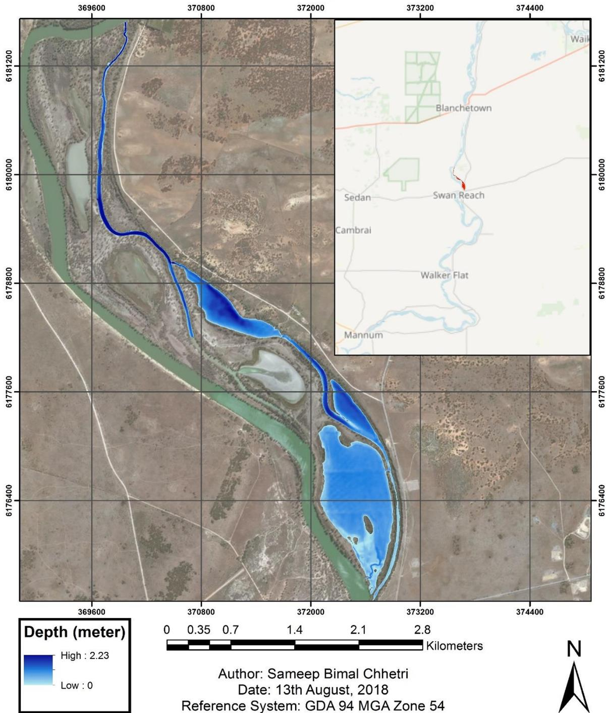
Figure 24 Maximum Depth Map for Wetland 7, 12 and 13 of Sugar Shack Complex
