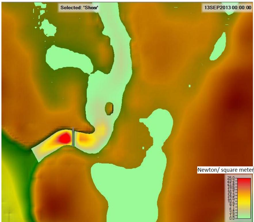
Figure 23 Local shear stress levels at gate 3 (open)
