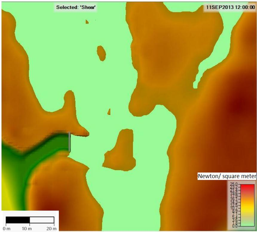
Figure 22 Local shear stress levels at gate 3(closed)
