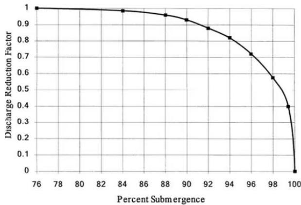
Figure 6 Submergence curve
