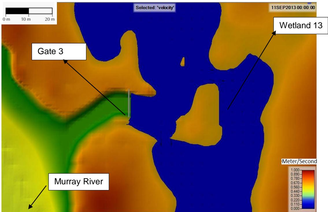
Figure 26 Velocity profile and fluid movement through Gate 3(fully closed) on 11th September
