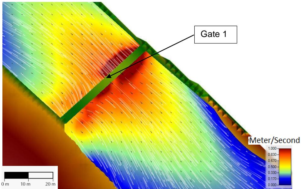
**Figure 13 Velocity profile and fluid movement through Gate 1(fully closed) on 08th sept**
