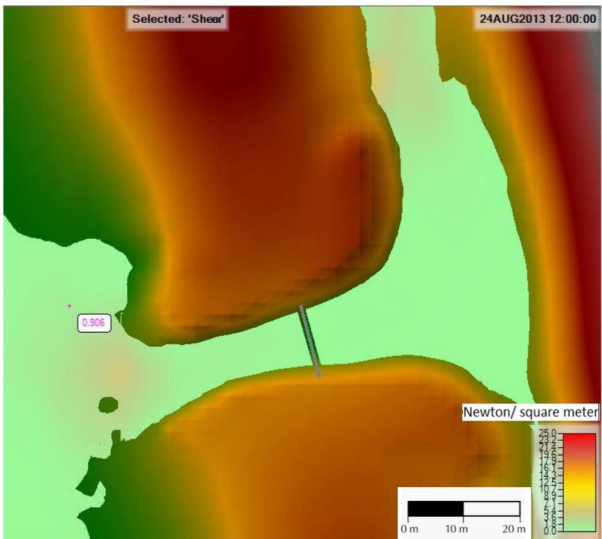
Figure 21 Local shear stress levels at gate 2 (open)
