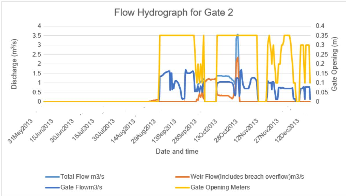
Figure 10 Flow hydrograph for Gate 2
