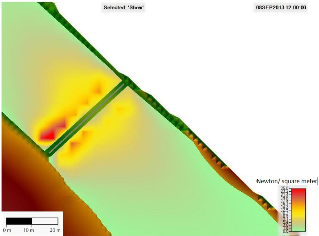
**Figure 38 Local shear stress levels at gate 1 (closed)**
