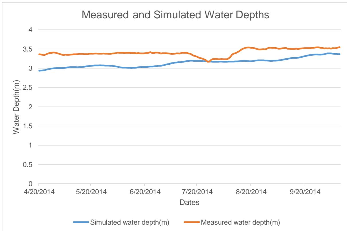
**Figure 7 Measured water depth and simulated water depth just upstream of Lock 1**
