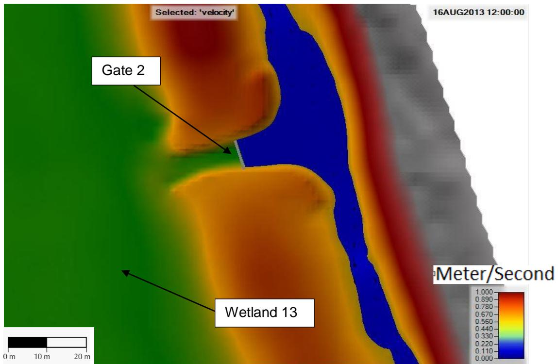
**Figure 14 Velocity profile and fluid movement through Gate 2(fully closed) on 16th August**
