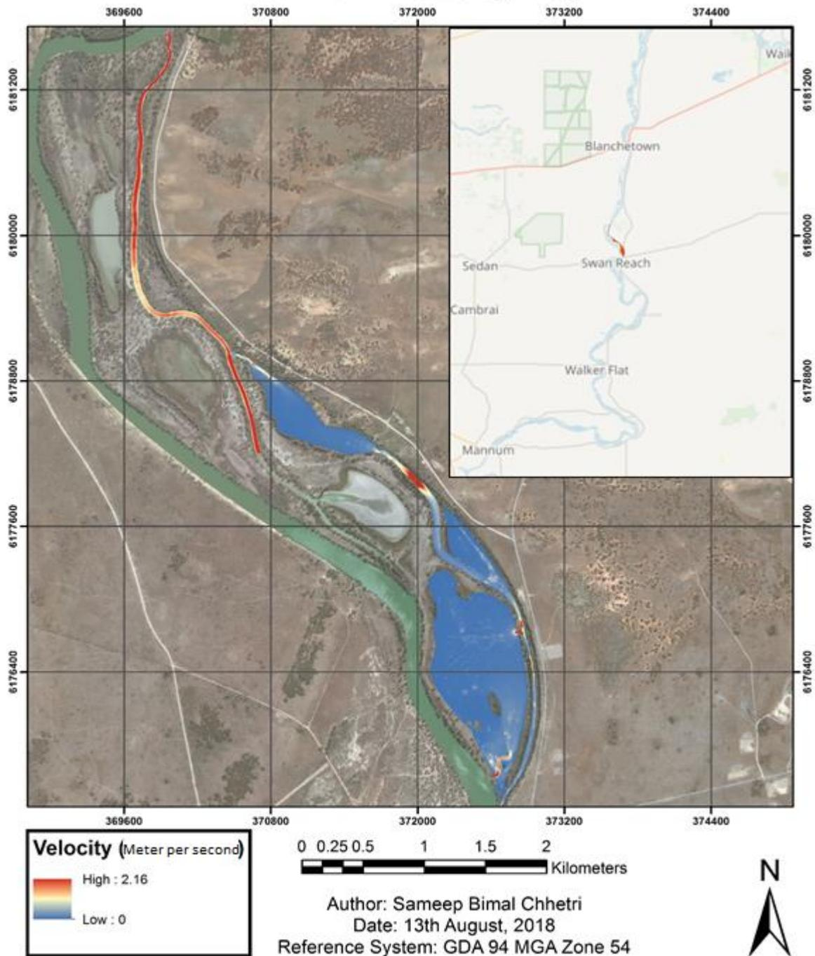
Figure 25 Maximum velocity map for Wetland 7,12 and 13 of sugar shack complex
