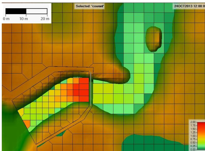
**Figure 8 Courant number for individual grids at Gate 3 on 24 october.**
