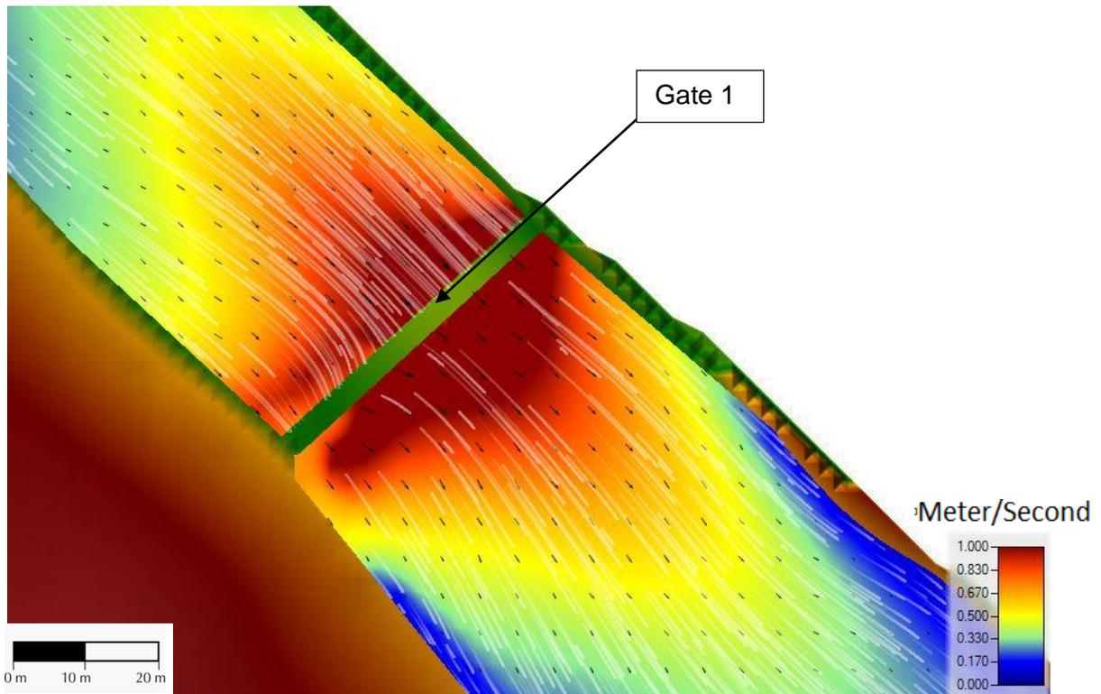
**Figure 12 Velocity profile and fluid movement through Gate 1(fully opened) on 05th oct**
