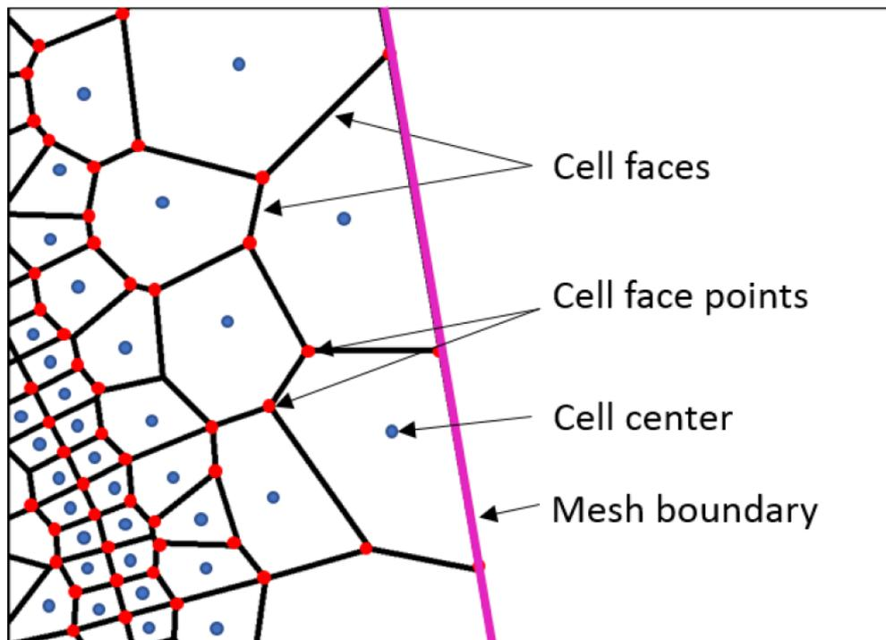
**Figure 5 Cell faces and computation faces of grids**
