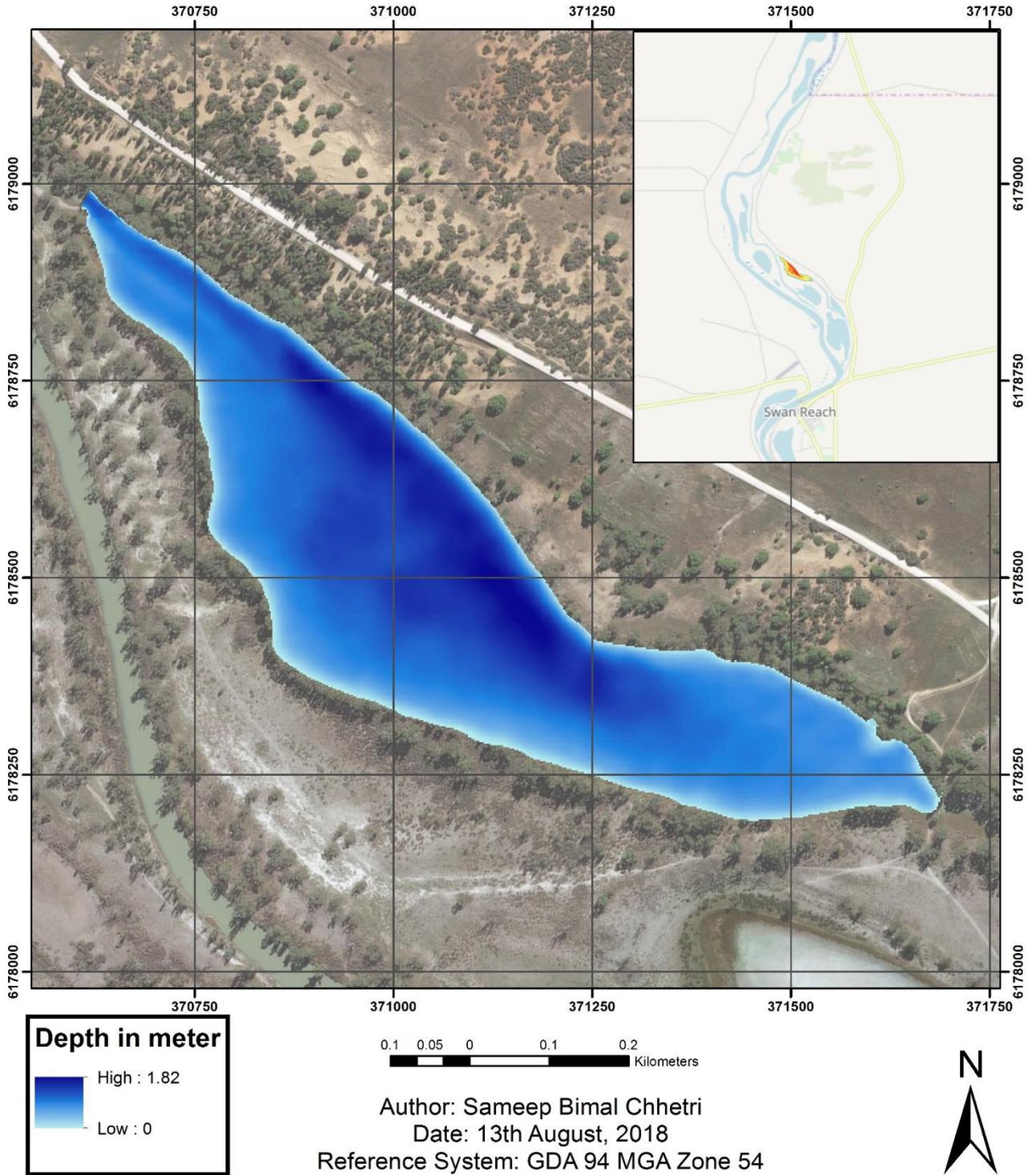
Figure 26 Maximum inundation map for wetland 7
