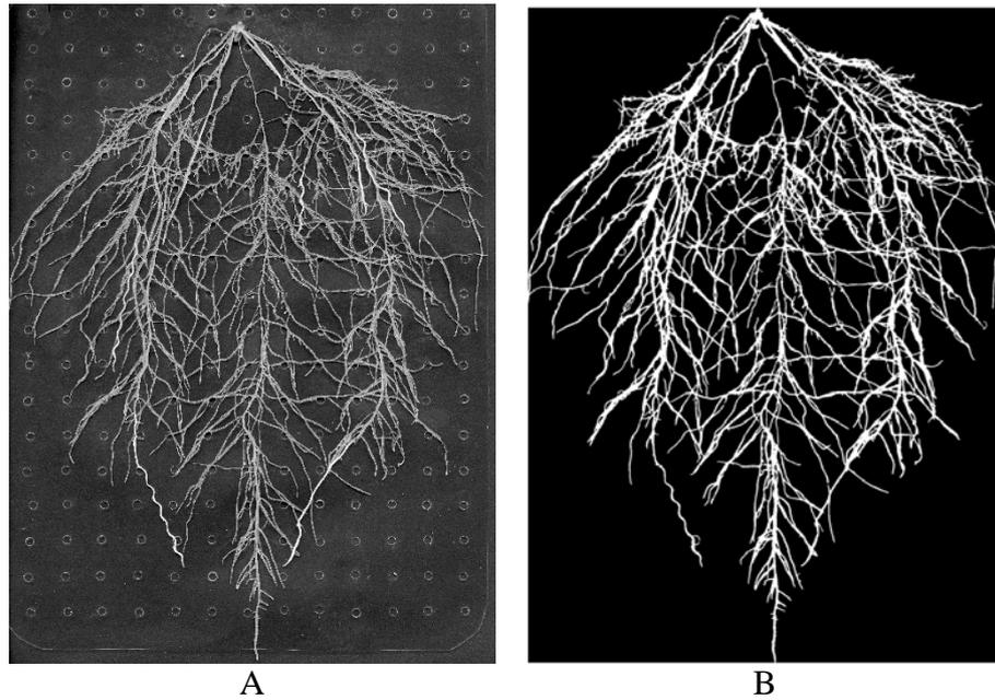
**Figure 4.6.** Original image (A) and the image processed by DIRT (B).
