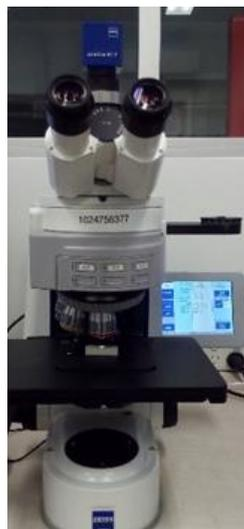
*Figure 23: ZEISS Optical Microscope used for porosity and microscope observation*
