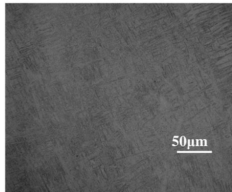
Figure 32: Optical images of sample 2 – Ti-28Nb-7Zr
