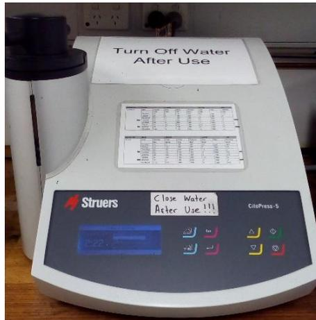
Figure 20: Mounting machine for sample preparation
