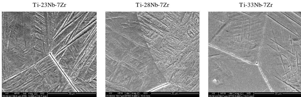
*Figure 37: Comparison of acicular and lath martensitic structure*
