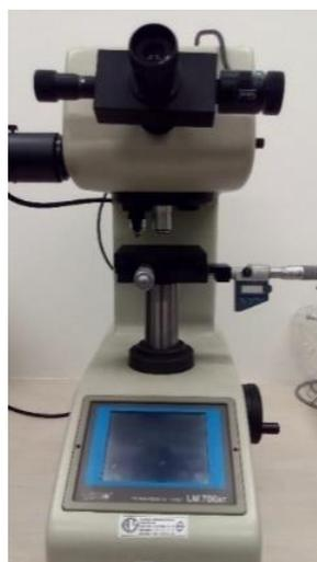
Figure 26: LM 700AT Microhardness Tester
