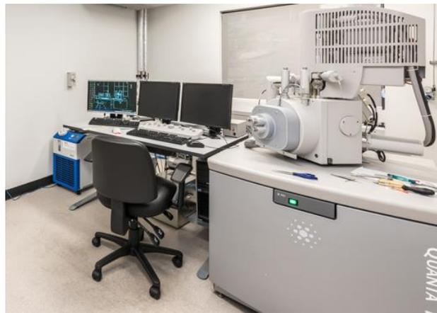
*Figure 24: Scanning Electron Microscope Quanta 450 with EDS Analyser*
