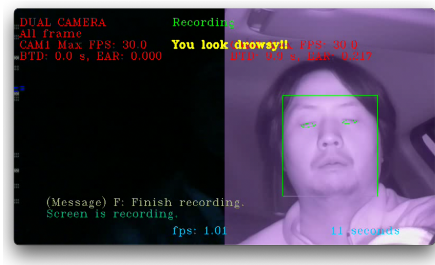
Figure 14 MS webcam vs Night Vision at low light
