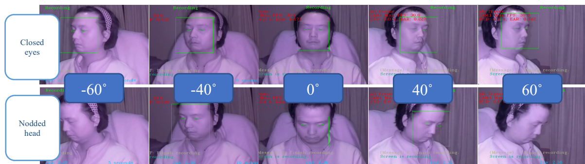
Figure 13 Screenshots showing the view of closed eyes and noddled head of Night Vision camera with various angles
