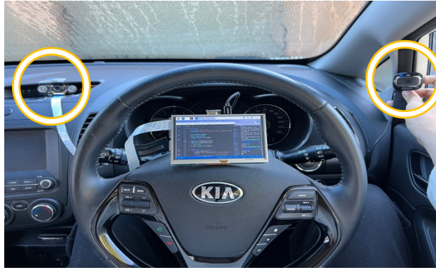
Figure 15 Experimental environment showing the position of the two cameras
