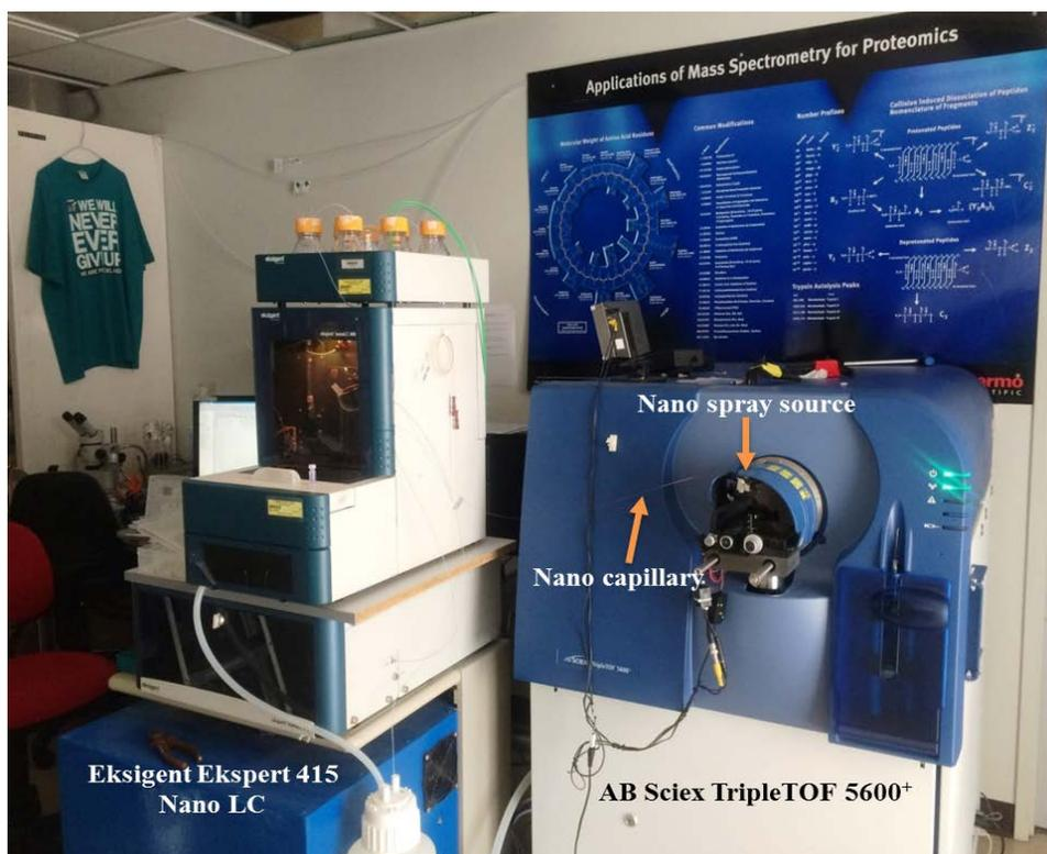
**Figure 2.3** A photograph to show the Nano-spray LC [Eksigent Ekspert 415] system coupled to AB Sciex TripleTOF 5600+ mass spectrometer [photograph taken in house (Flinders Proteomics facility)].
