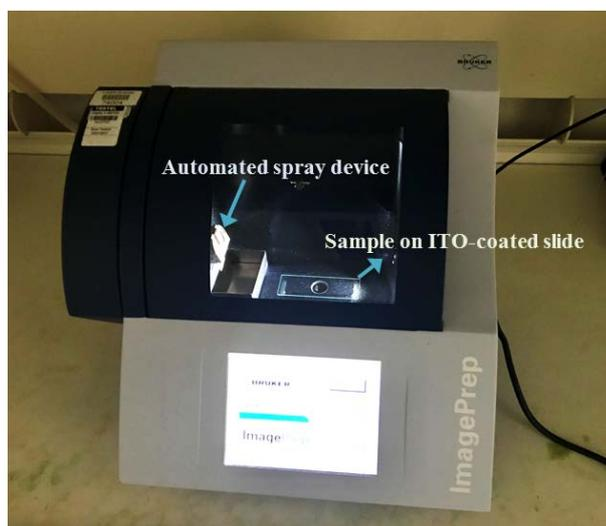
**Figure 2.4** A Photograph to show the ImagePrep station (Bruker Daltonics, Bremen, Germany) used for the automated homogenous sample preparation [Photo taken in the Flinders Mass Spectrometry Facility].
