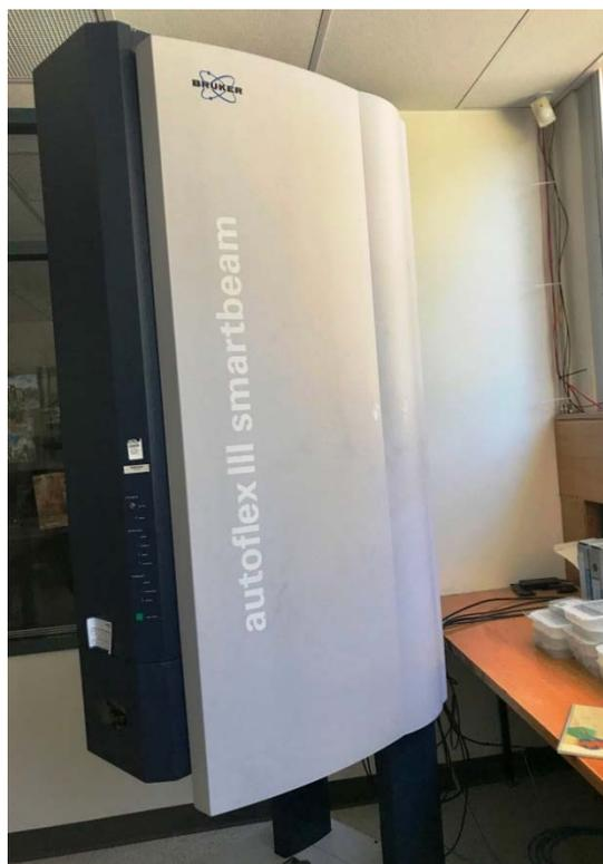
**Figure 2.1** A photograph to show the Autoflex-III MALDI-TOF-MS [Bruker Daltonics, GmbH, Germany] mass spectrometer. Photograph taken in house [Flinders Analytical].
