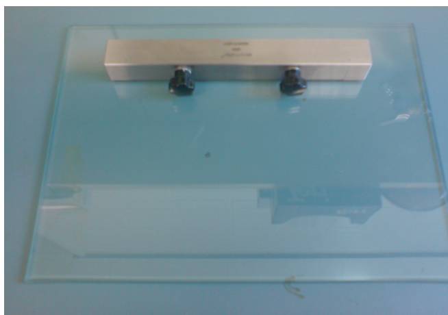
Figure 2.2. Set up for membrane casting with doctor's blade and glass plate.
