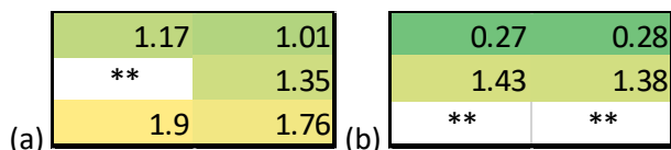
Figure 10: The methamphetamine concentrations for the Kitchen wipe samples (a) the pre-remediation heat map; (b) the post remediation heat map
