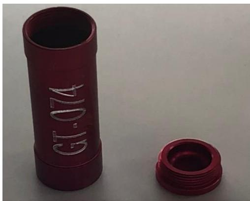
*Figure 5.3. Al can used in NAA for long sample irradiation times.*
