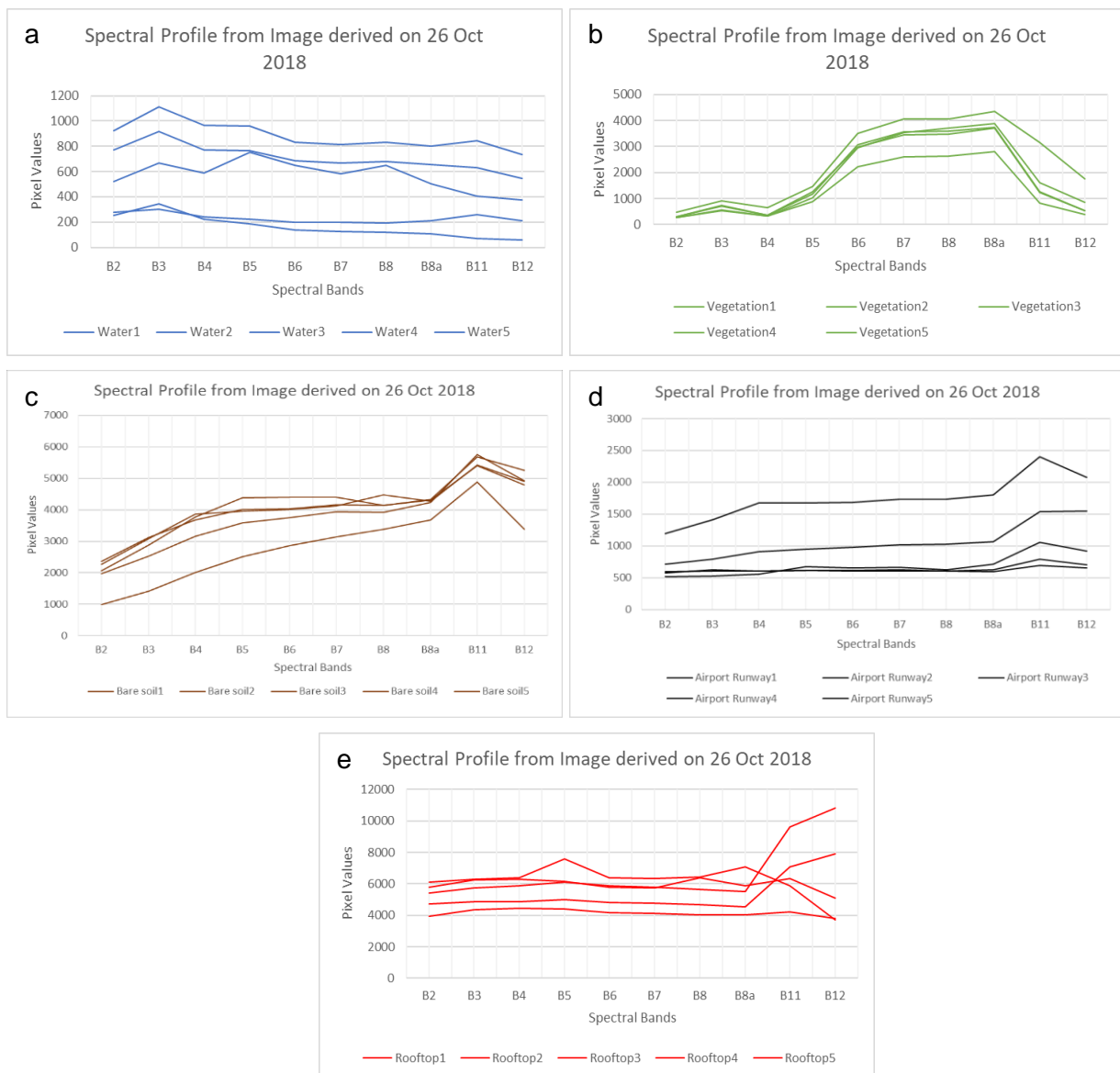
Figure 22: The spectral profiles of five different landcover types derived from the Sentinel 2 image acquired on 26 October, 2018; a) spectral signature of water; b) spectral signature of vegetation; c) spectral signature of bare soil; d) spectral signature of the airport runway; e) spectral signature of rooftops.
