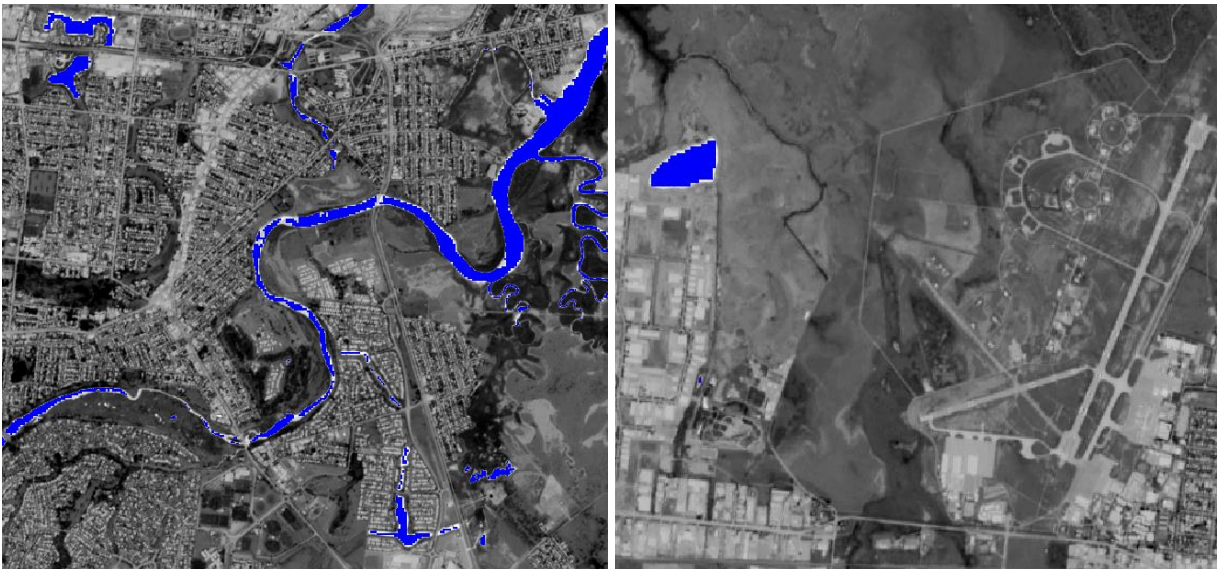
Figure 27: Results from the combination of the threshold of NDWI and the threshold of a single SWIR band.
