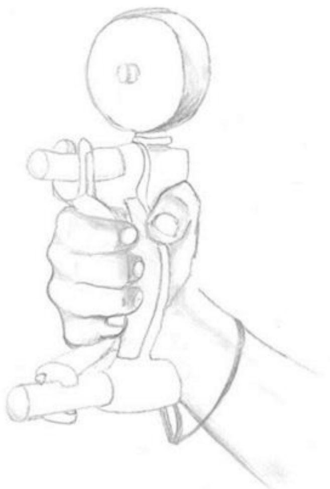
Figure 3: HGS measured with a sealed Jamar hydraulic dynamometer (Artist: Sasha Simpson)
