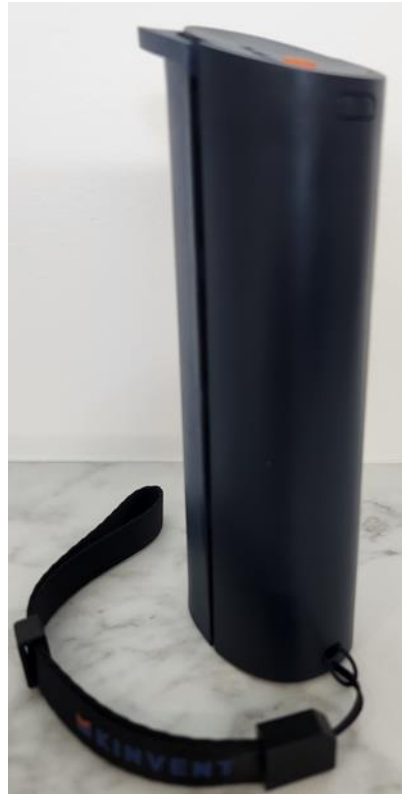
Figure 20: K-force hand grip strength measurement tool (photographed by author)
