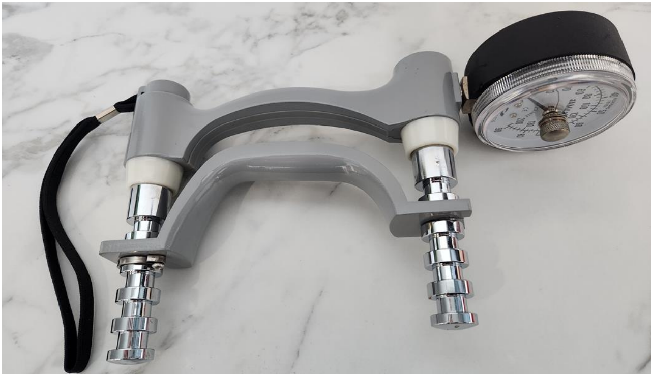
Figure 19: Jamar hydraulic hand grip dynamometer (photographed by author)
