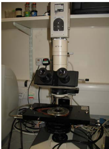
Figure 1. 34: Optical rheology apparatus that can take images of the samples while it models the affects of a rheometer.
