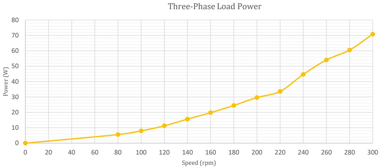
Figure 124: Load power calculated for the three-phase resistive test
