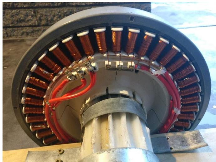
*Figure 115: Regrouped stator with rotor and shaft attached*
