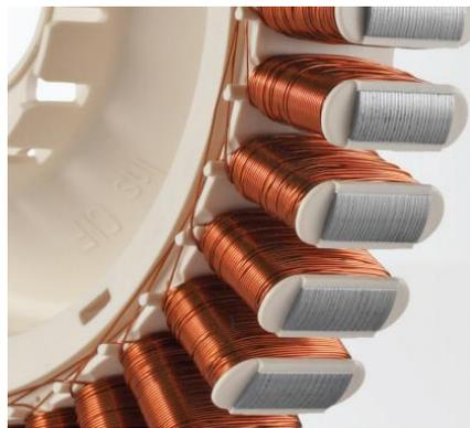
Figure 111: Picture showing the plastic coating of the stator, with exposed iron at the tips [28]
