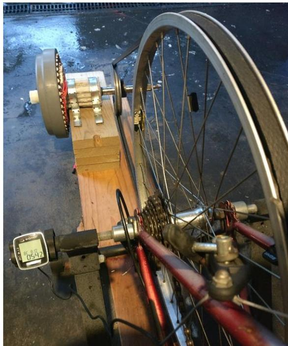
Figure 117: Tachometer in the setup used for speed measurement
