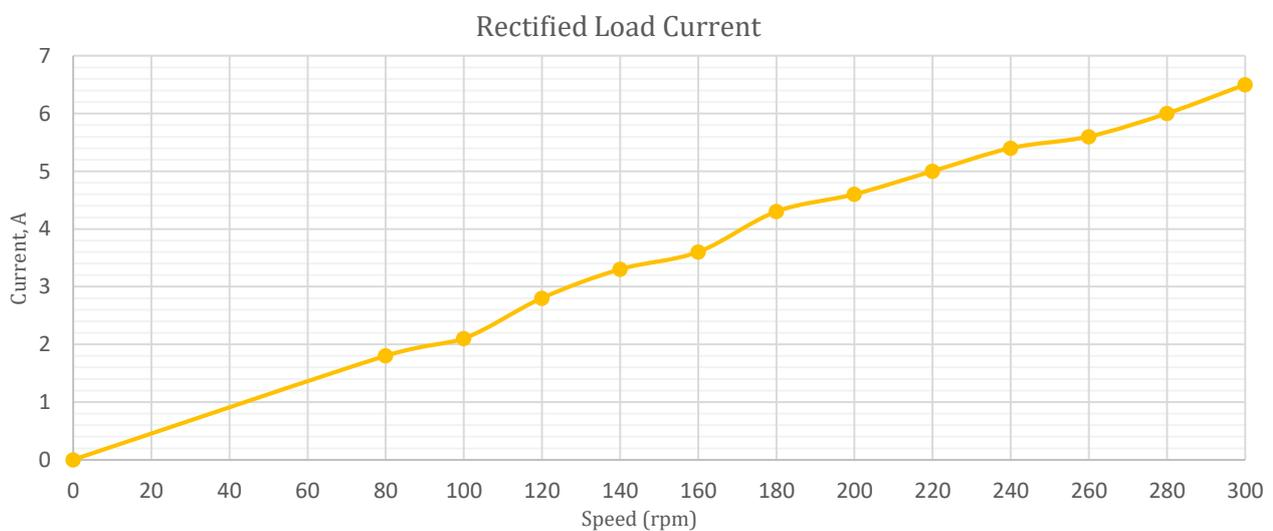
Figure 126: Measured current over 3 $\Omega$  load with rectified output
