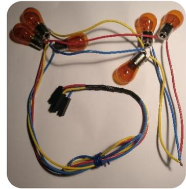
*Figure 118: Three-phase incandescent bulb load*
