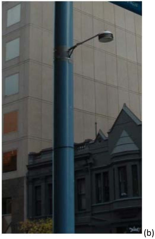
Figure 2: (a) A collection of Maxim Thermochron ibutton sensors set up for calibration, (b) An ibutton placed in the louvred radiation shield and mounted from a lighting standard pole in the CBD (Guan et al., 2013).
