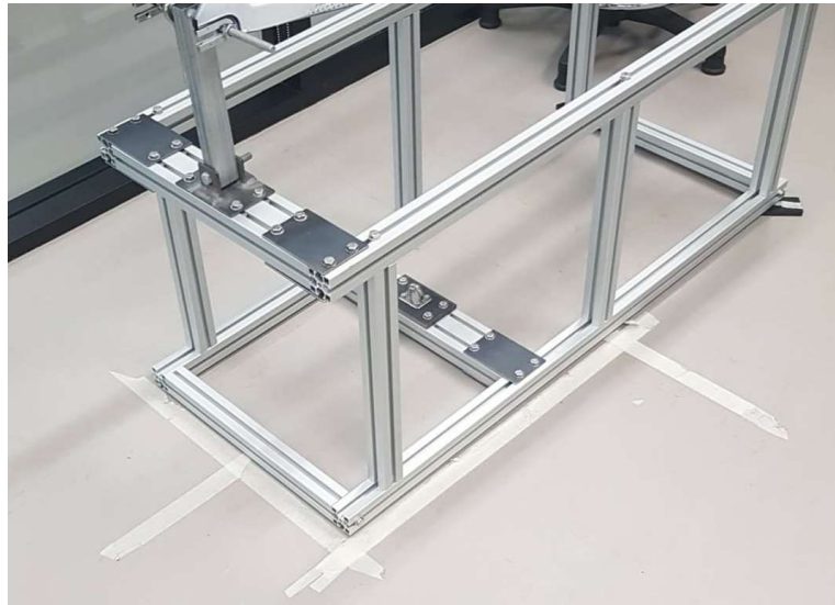
Figure 30: Tape Applied on Ground to Show Where the Cameras Were in Focus
