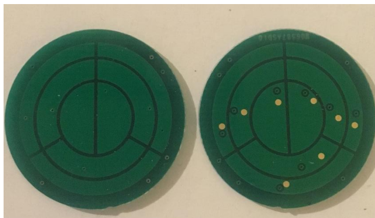
Figure 43 - Resulting electrode design (Author's own)
