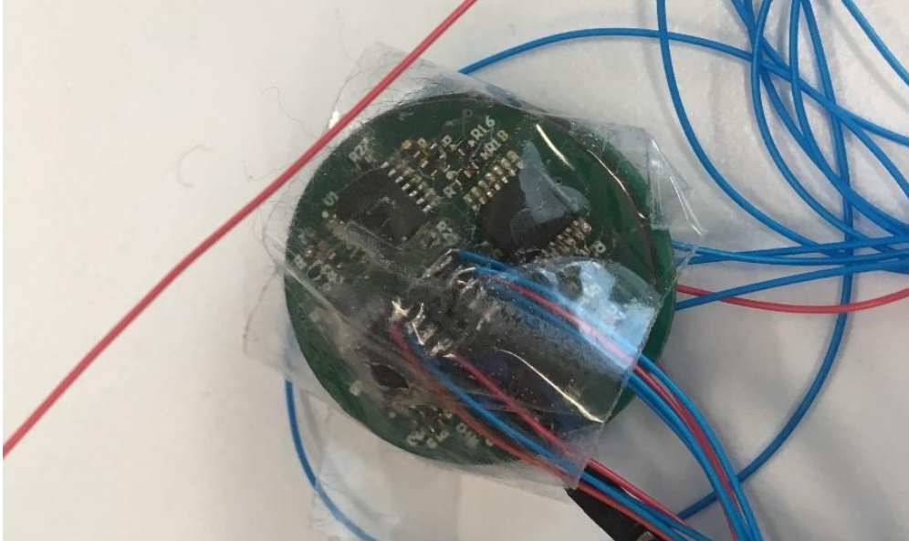
Figure 40 - Sensor and dummy electrode connected back to back (Author's own)
