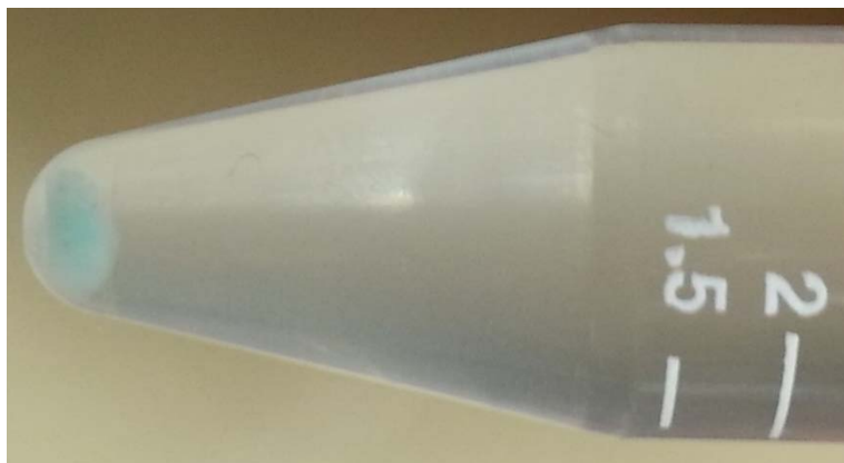
Figure 61: Cy5 labelled target sequence adsorbed to cleaned, bare amine functionalised nanoparticles shown as blue
